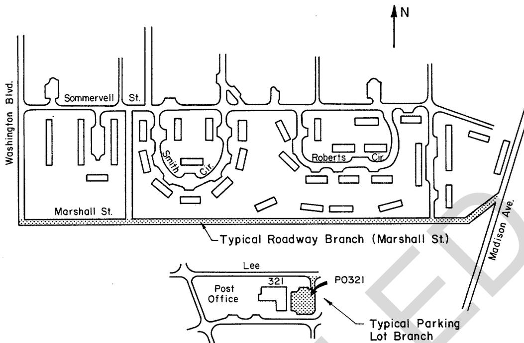
Figure 2-1. Installation map showing typical pavement branches.
