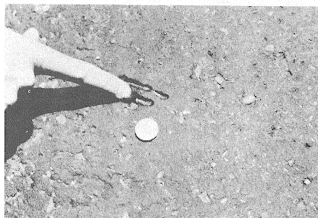
Figure B-9. Medium-severity bleeding.
