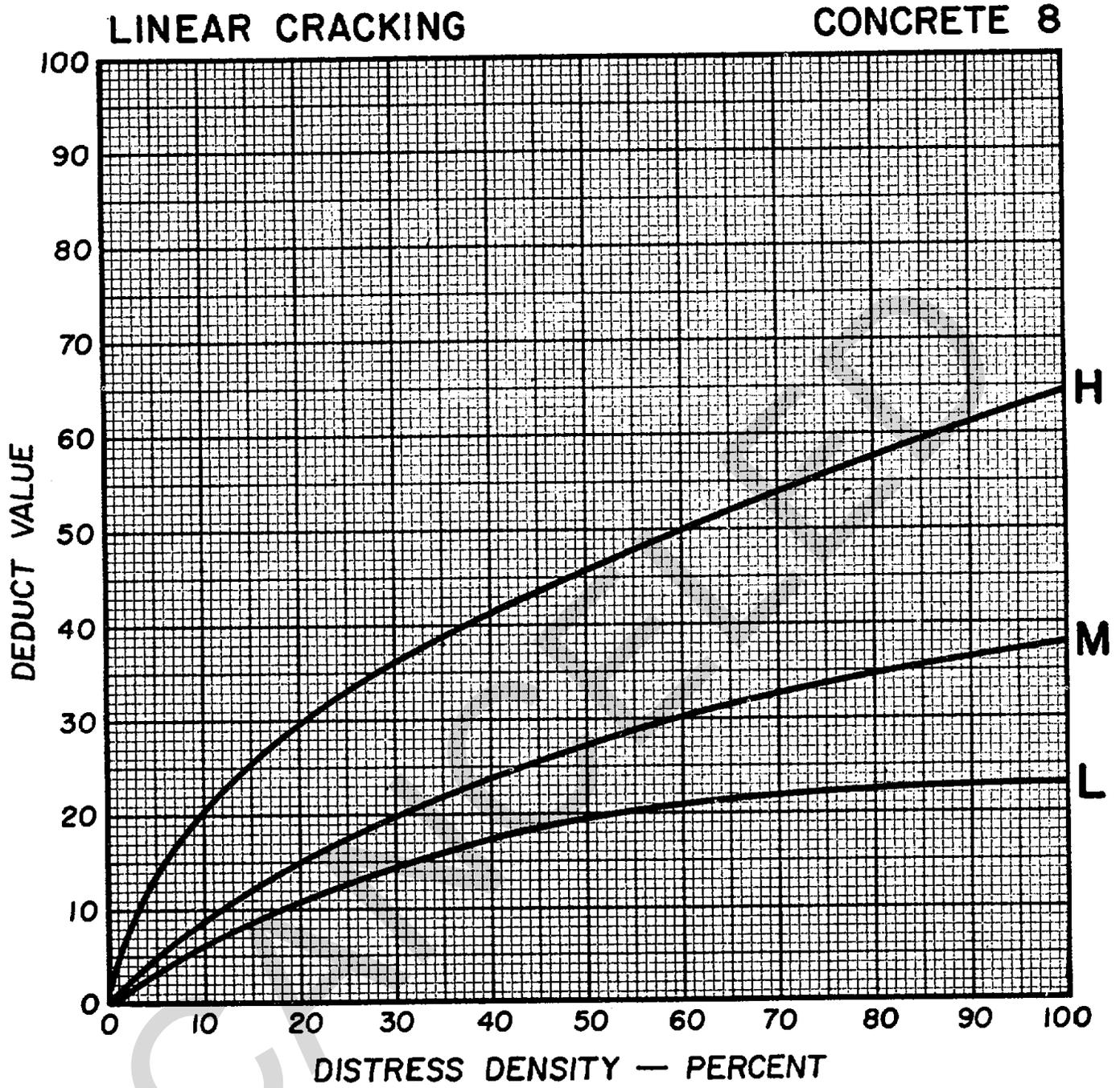
Figure C-28. Deduct value curves for linear cracking.
