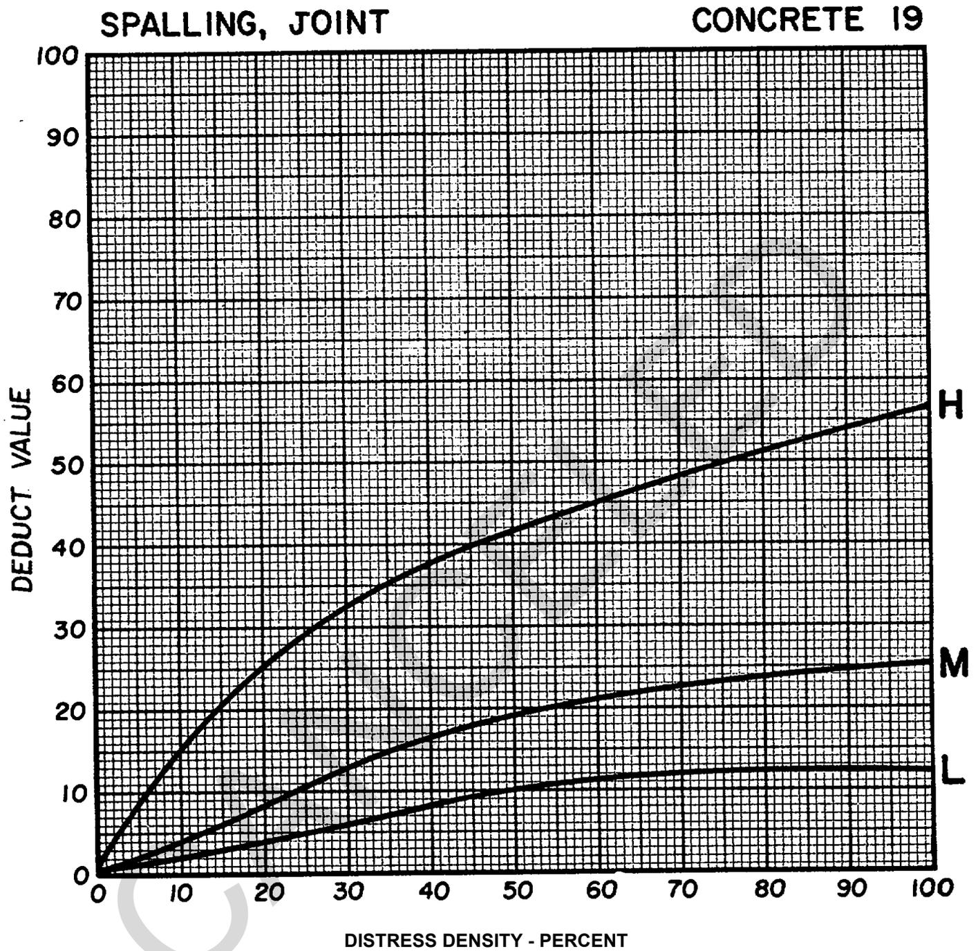
Figure C-39. Deduct value curves for spalling, joint.
