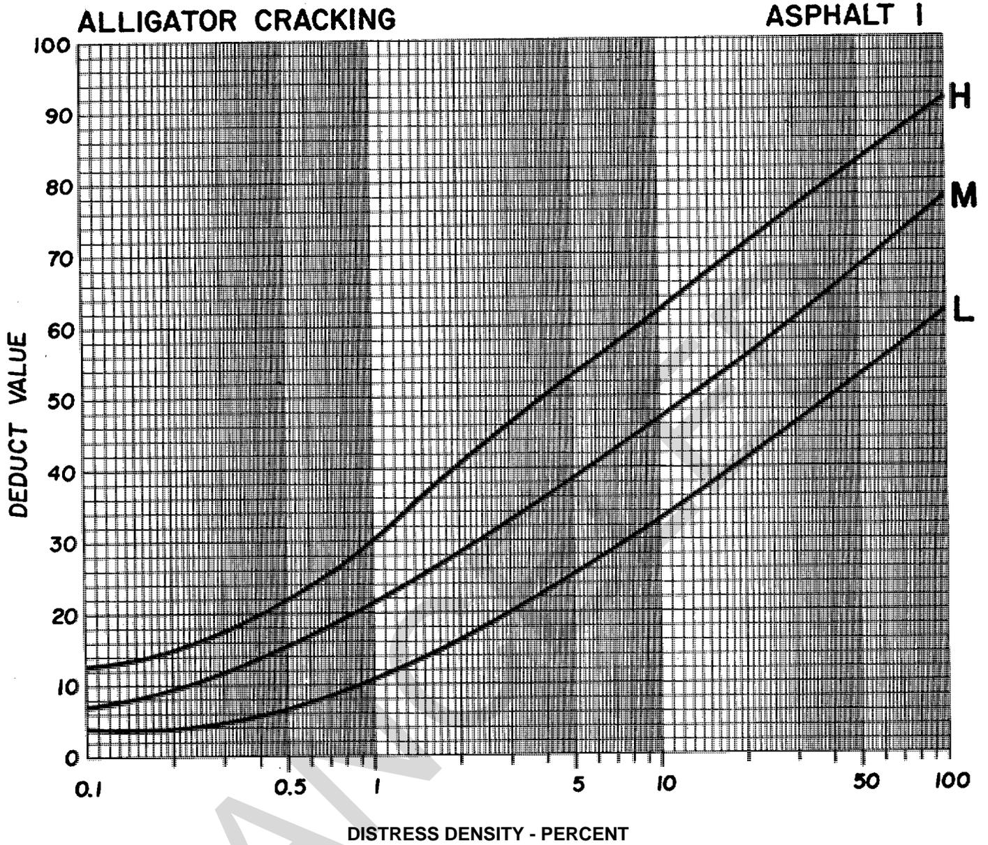
Figure C-1. Deduct value curves for alligator cracking.
