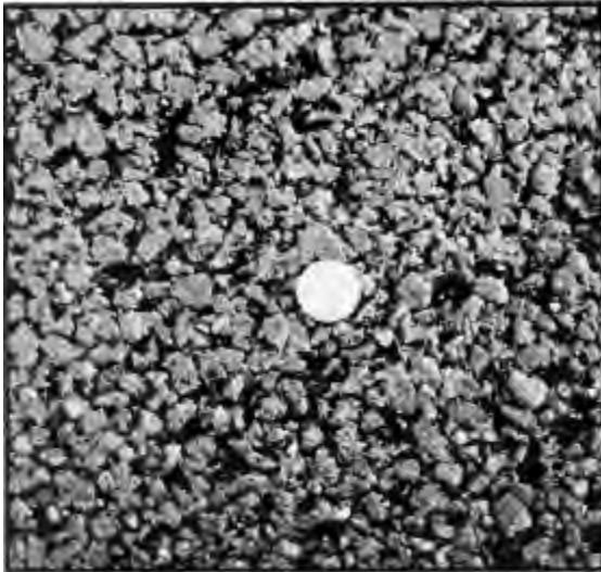
Figure 8.2. Porous friction pavement patch using hot-asphalt plant mix
