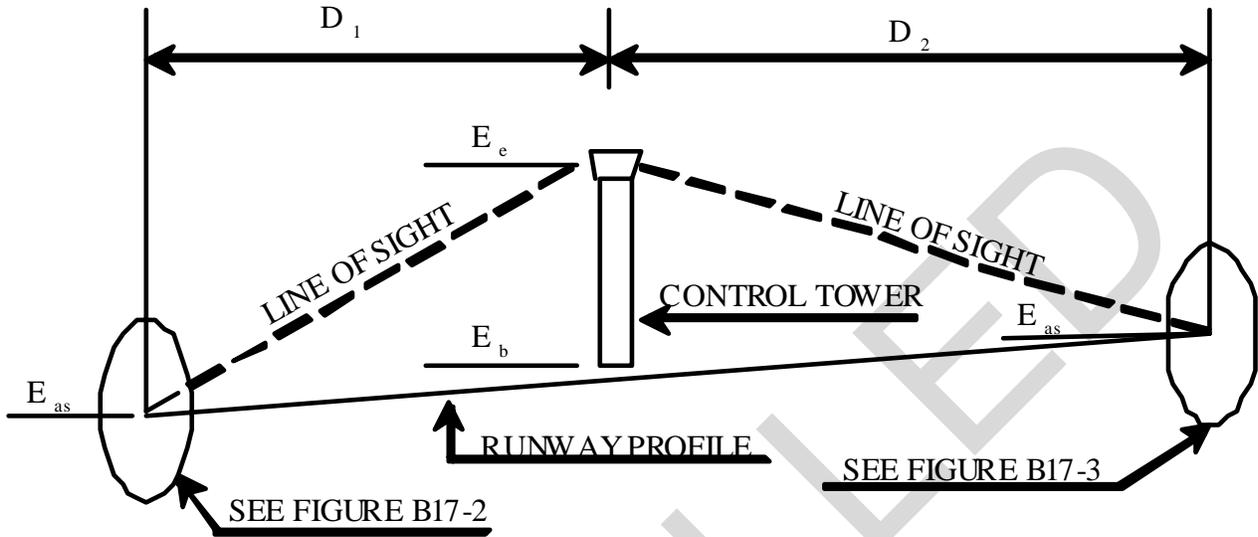
Figure B17-2. Minimum Eye-Level Determination
