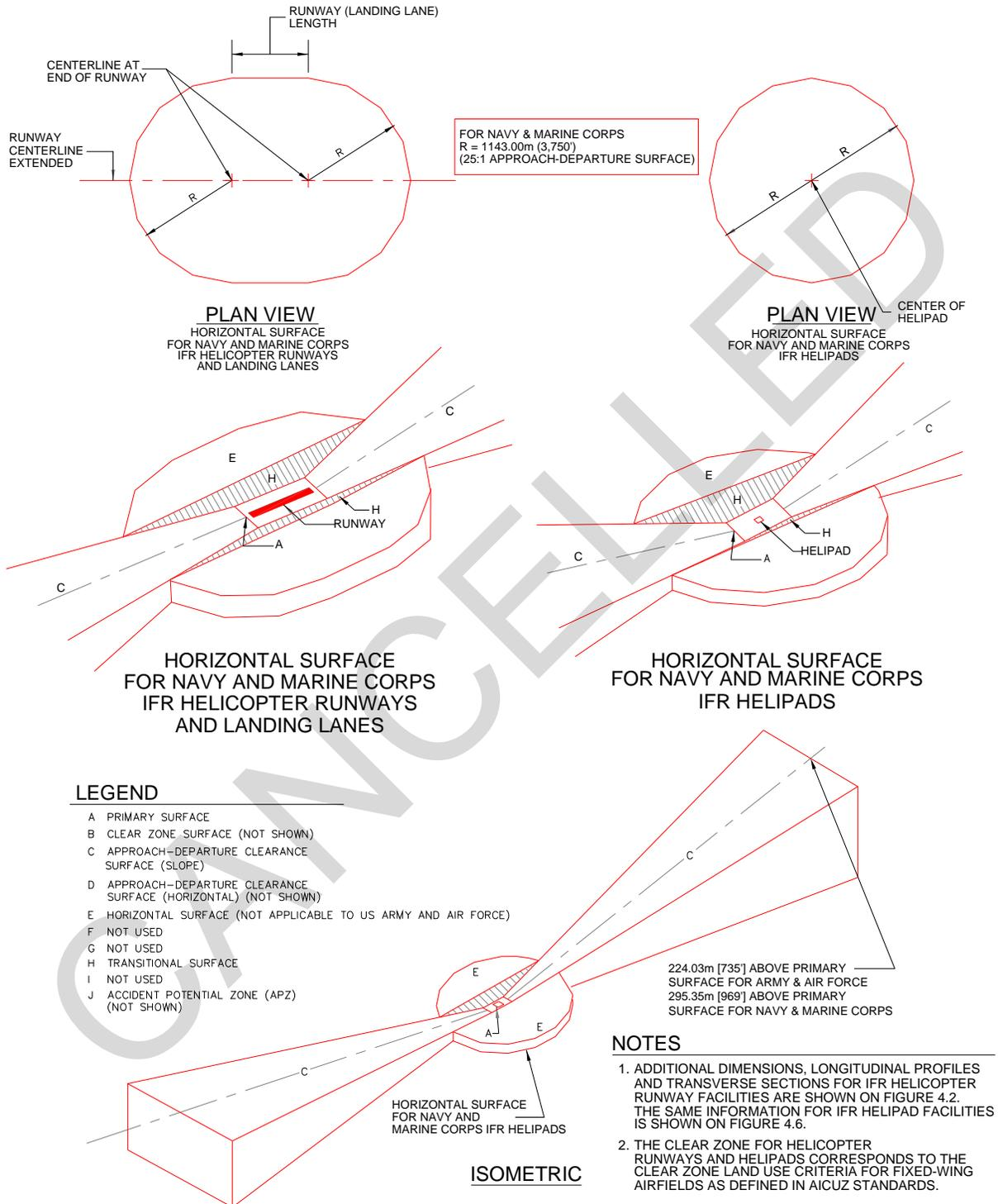
4-4 **HELIPADS.** Helipads allow for a helicopter hovering, landing, and takeoff. Except at facilities where helicopter runways are provided, helipads are the landing and takeoff locations for helicopters. The Army and Air Force provide for three types of helipads: standard VFR helipad, limited use helipad, and IFR helipad. The Navy and Marine Corps provide only one type of helipad: standard size helipad. The type of helipad depends on these operational requirements:
