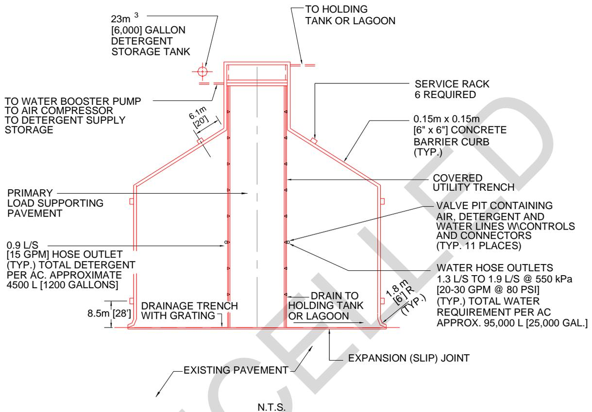
6-14.8 **Wastewater Collection.** Waste drains will be located in the center of the wash rack pavement to collect wash water contaminants (oils, alkaline, salts, and other contaminants) generated from aircraft washing operations. Off-center waste and trench drains are permitted only where necessitated by the aircraft landing gear configuration or where the off-center drains reduce construction costs or suit existing conditions.
