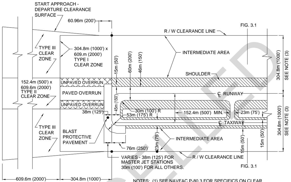
914.4m (3000') LONG CLEAR ZONE, WIDTH IS THE SAME AS APPROACH-DEPARTURE CLEARANCE SURFACE. SEE NAVFAC P-80.3 & FIG. 3.6 FOR DETAILS.
