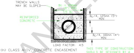
SHOULD BE DESIGNED BY A REGISTERED STRUCTURAL ENGINEER, AND MAY YIELD HIGHER LOAD FACTORS THAN INDICATED.
