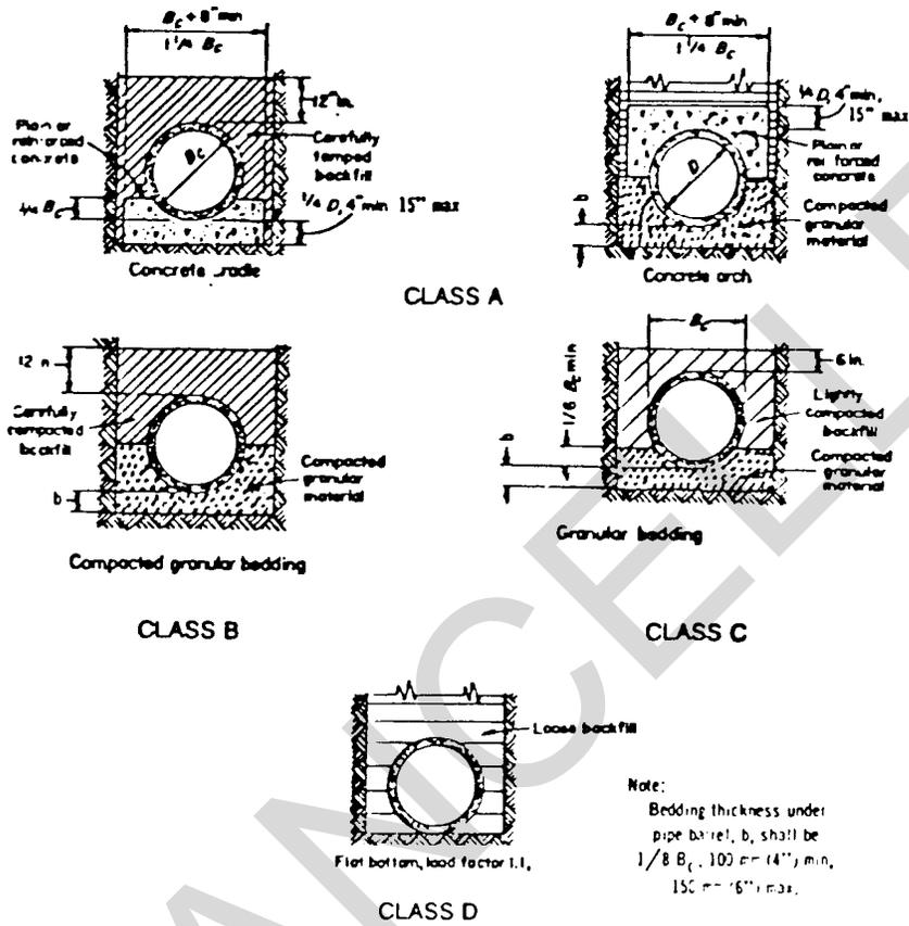
Figure C-4. Trench Beddings for Circular Pipe
