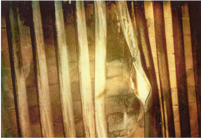
Figure 4-9 Failed Boiler Tube
