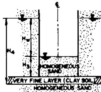
TO AVOID BOTTOM HEAVE,  $\gamma_T \times H_3$  SHOULD BE GREATER THAN  $\gamma_W \times H_4$ .
