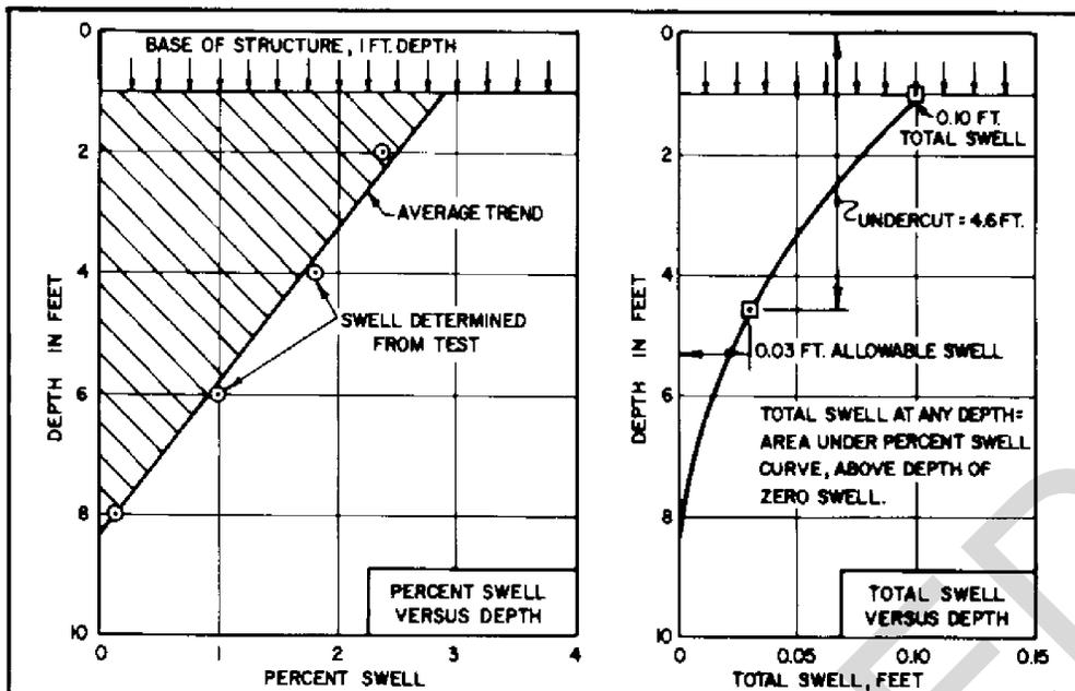
MATERIALS INVESTIGATED ARE CLAYS, HIGHLY OVERCONSOLIDATED BY CAPILLARY STRESSES THAT ARE EFFECTIVE PRIOR TO THE CONSTRUCTION OF THE STRUCTURE UPON THEM.
