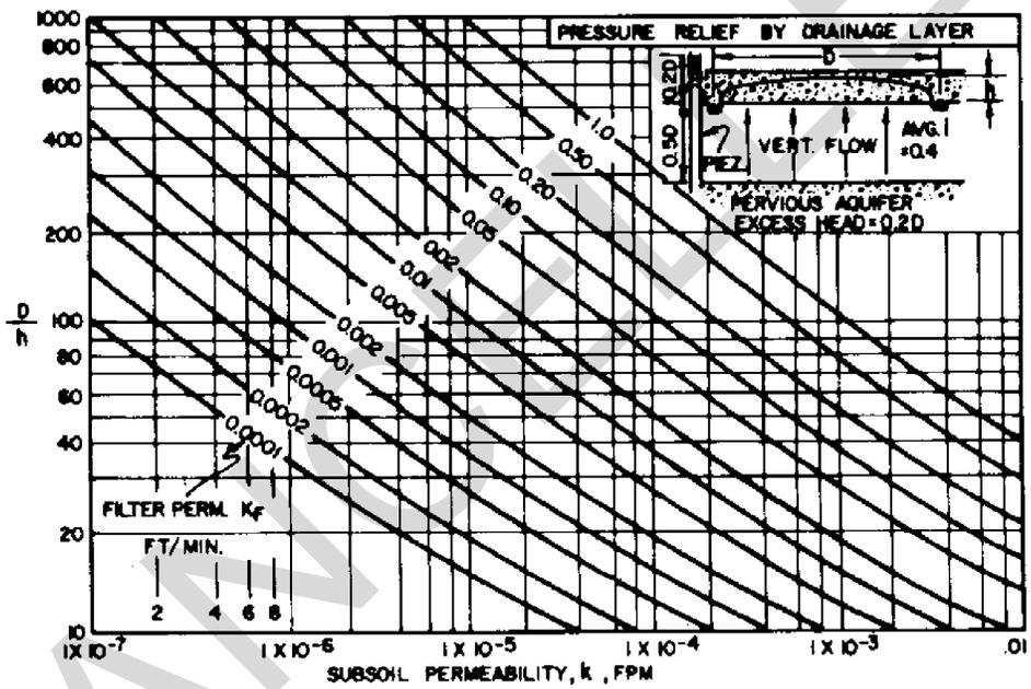
ASSUMPTIONS: STEADY SEEPAGE MOVES VERTICALLY UPWARD FROM AQUIFER AT DEPTH 0.5D WITH AVERAGE GRADIENT = 0.4.
