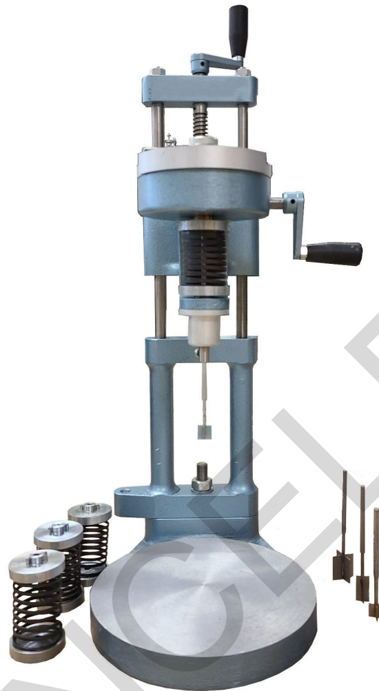
Figure 3-9 Laboratory Miniature Vane Shear Apparatus
