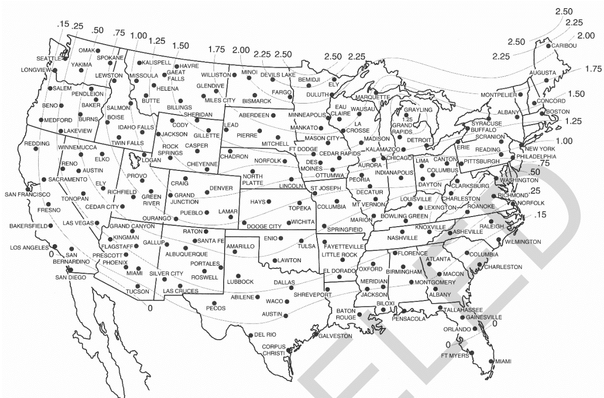
Figure 1-11 Maximum Depths (in meters) of Frost Penetration in the Continental United States (NOAA 1978)
