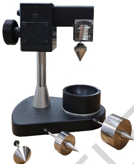
Figure 3-10 Fall Cone Apparatus
