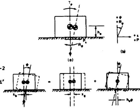
$$P_x = -c_x \dot{x}_b - k_x x_b, \quad R_\psi = -c_\psi \dot{\psi} - k_\psi \psi$$
