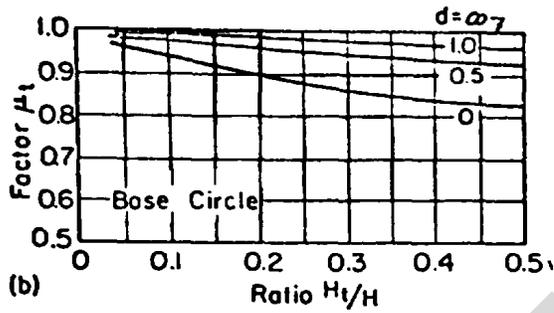
REDUCTION FACTOR FOR TENSION CRACK
