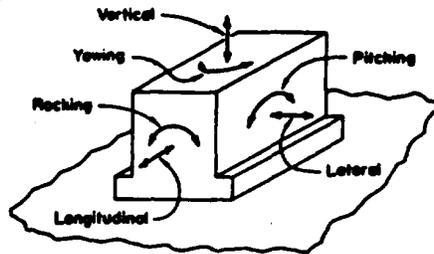
Figure 17-3. Six modes of vibration for a foundation.
