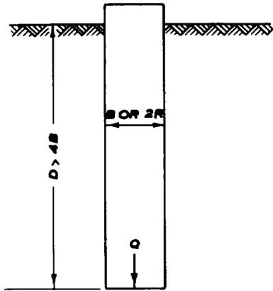
BEARING CAPACITY FACTORS,  $N_c$  FOR FOUNDATIONS IN CLAY ( $\phi = 0^\circ$ )
