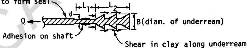
$$Q_u = \pi B L_2 s_u F_1 + \frac{\pi}{4} (B^2 - d^2) N_c s_u + \pi d L c_a$$
