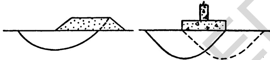
$$(s_U)_{\text{DESIGN}} = \gamma (s_U)_{\text{VANE}}$$
