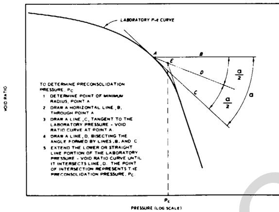
GRAPHICAL CONSTRUCTION OF PRECONSOLIDATION PRESSURE
