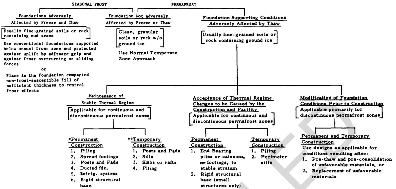
\*Permanent Construction - Construction incorporating the type and quality of materials and equipment, and details and methods of construction, which results in a building or facility suitable to serve a specific purpose over a minimum life expectancy of 25 years with normal maintenance.
