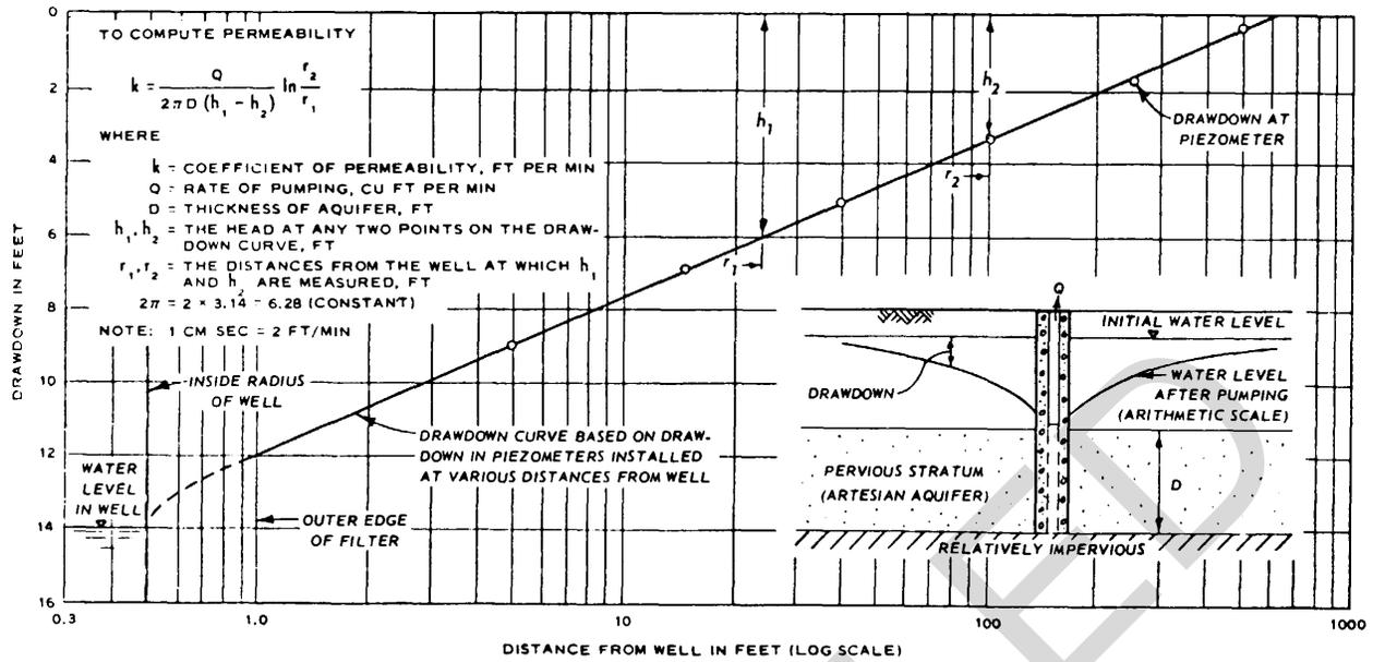
**NOTE. WELL SHOULD BE PUMPED AT A CONSTANT RATE OF FLOW UNTIL THE RATE OF DRAWDOWN IN WELL AND PIEZOMETERS IS ESSENTIALLY CONSTANT.**
