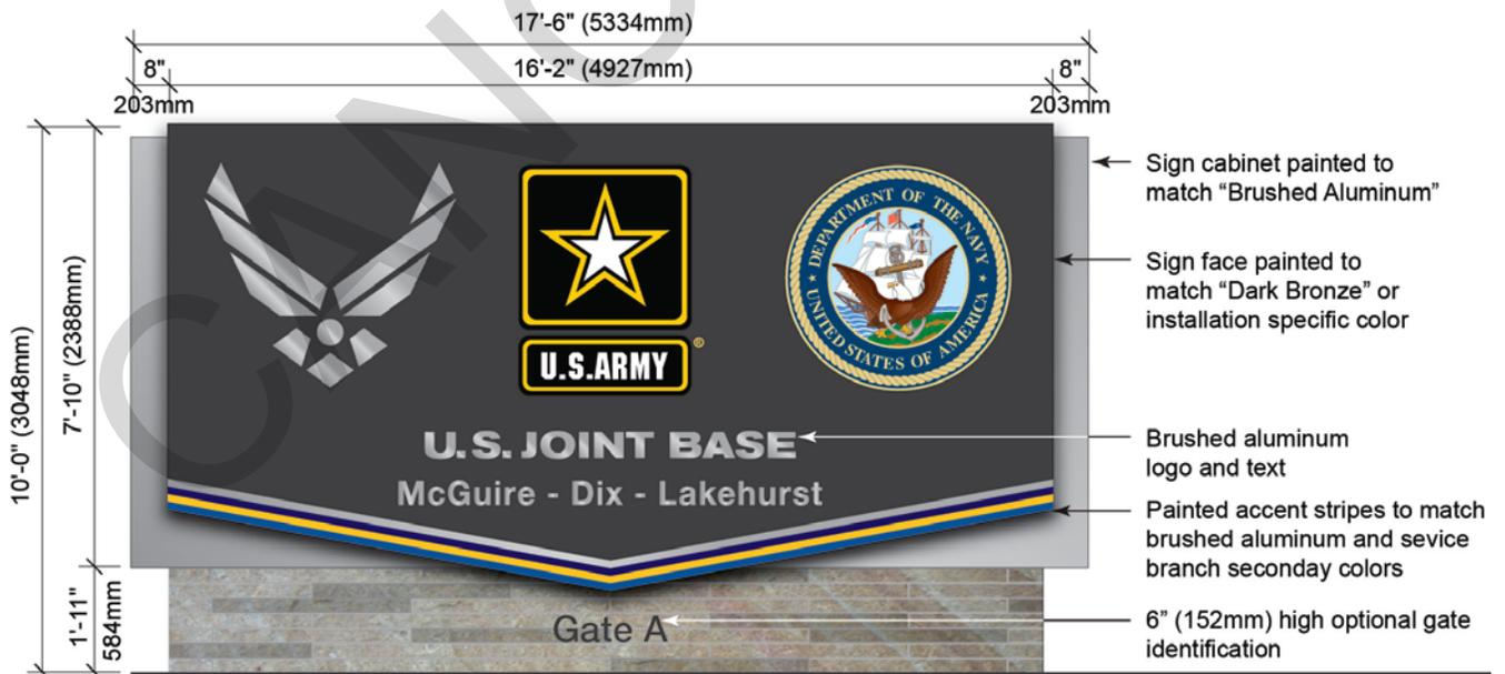
Figure 3-6 Primary Joint Installation Sign Layout Details.
