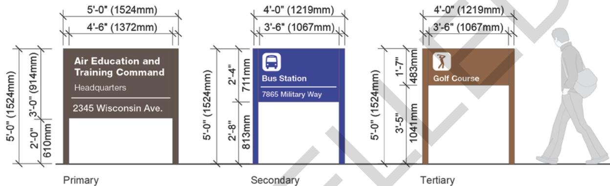
Figure 3-11 Freestanding Building Identification Sign Layouts.
