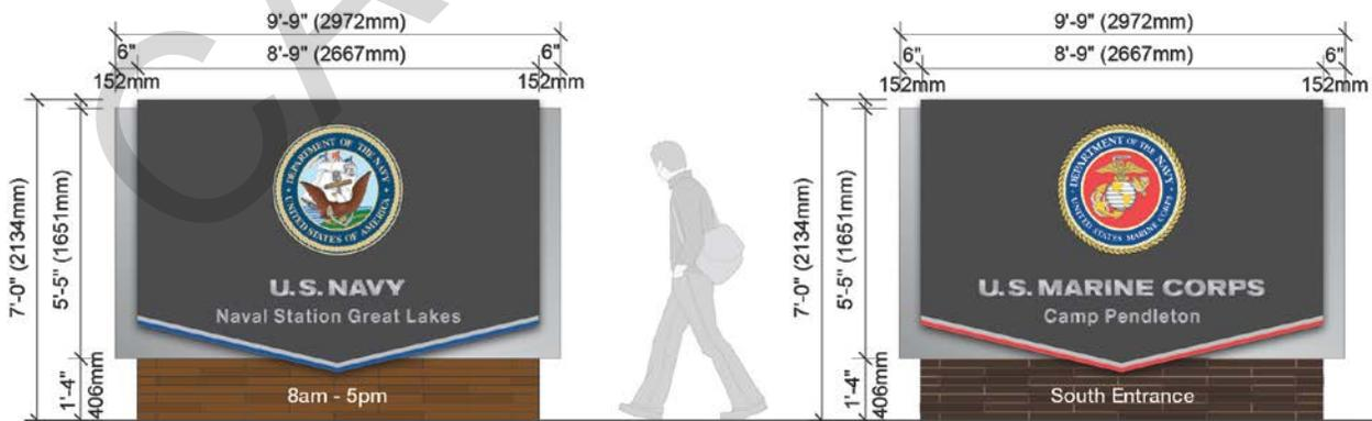
Figure 3-8 Secondary Installation Sign Layout Details.
