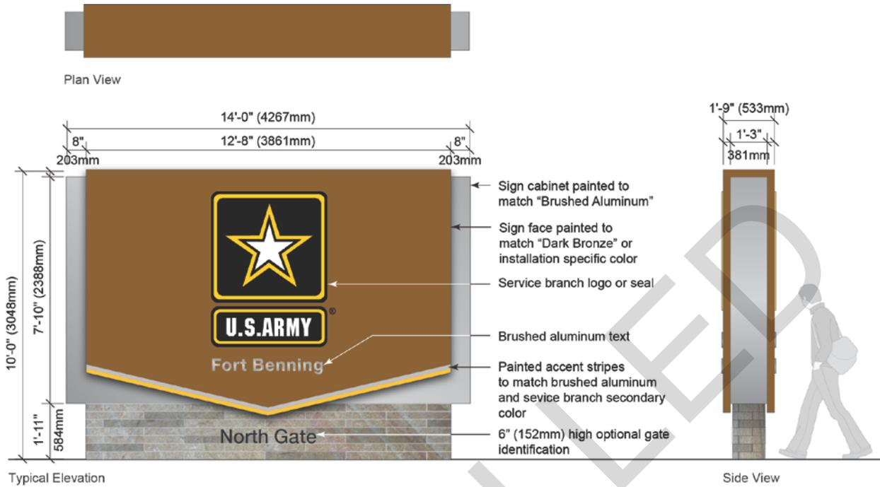
Figure 3-3 Primary Installation and Gate Identification Signs.
