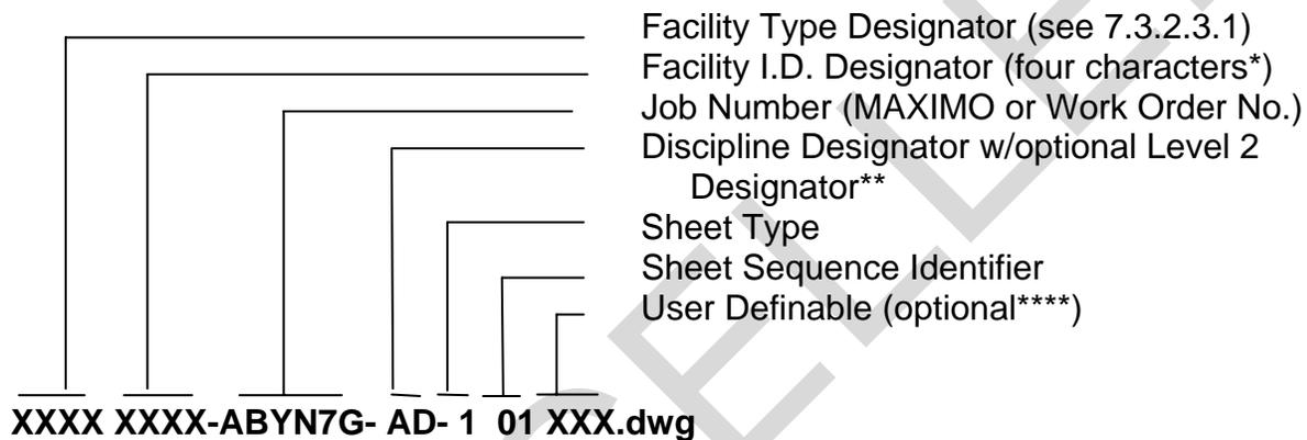
\* If no building designation has been assigned, such as for new construction prior to completion, then utilize the project number (P-number) for the Facility Type and I.D. designators. If installation has an alternate building identification system, that designator may be utilized in lieu of the Facility Type and Facility I.D. Designator.
