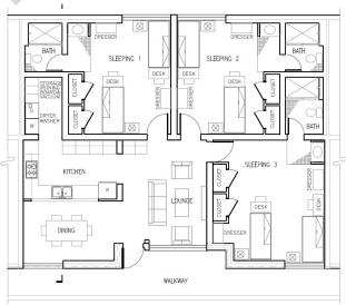
Installations with Welton Becket style buildings, and surplus capacity, should consider re-designs similar to the concept in Figure B-2 above. Note that the re-design provides built-in closets, a separate vanity area for each restroom, in-unit laundry, and space for Market Style furnishings.
