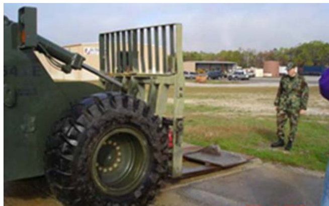
Figure 3-9. Position Plate with Forklift.
