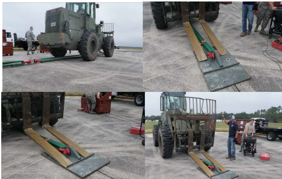
Figure 3-11. Align Slings with Forklift.
