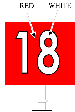
A. HOLDING POSITION SIGN AT RUNWAY THRESHOLD.
