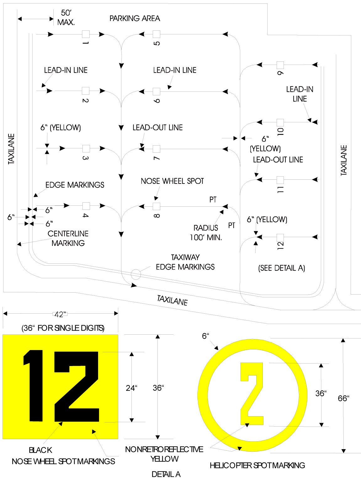
Figure 2. Examples of Parking Area Markings
