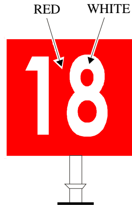
A. HOLDING POSITION SIGN AT RUNWAY THRESHOLD.
