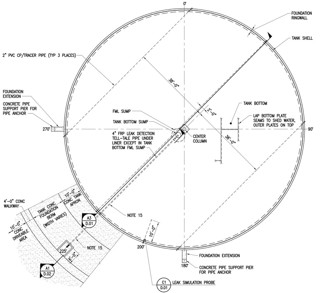
**80K BBL TANK BOTTOM, FOUNDATION, AND INTERSTITIAL PIPING PLAN**
