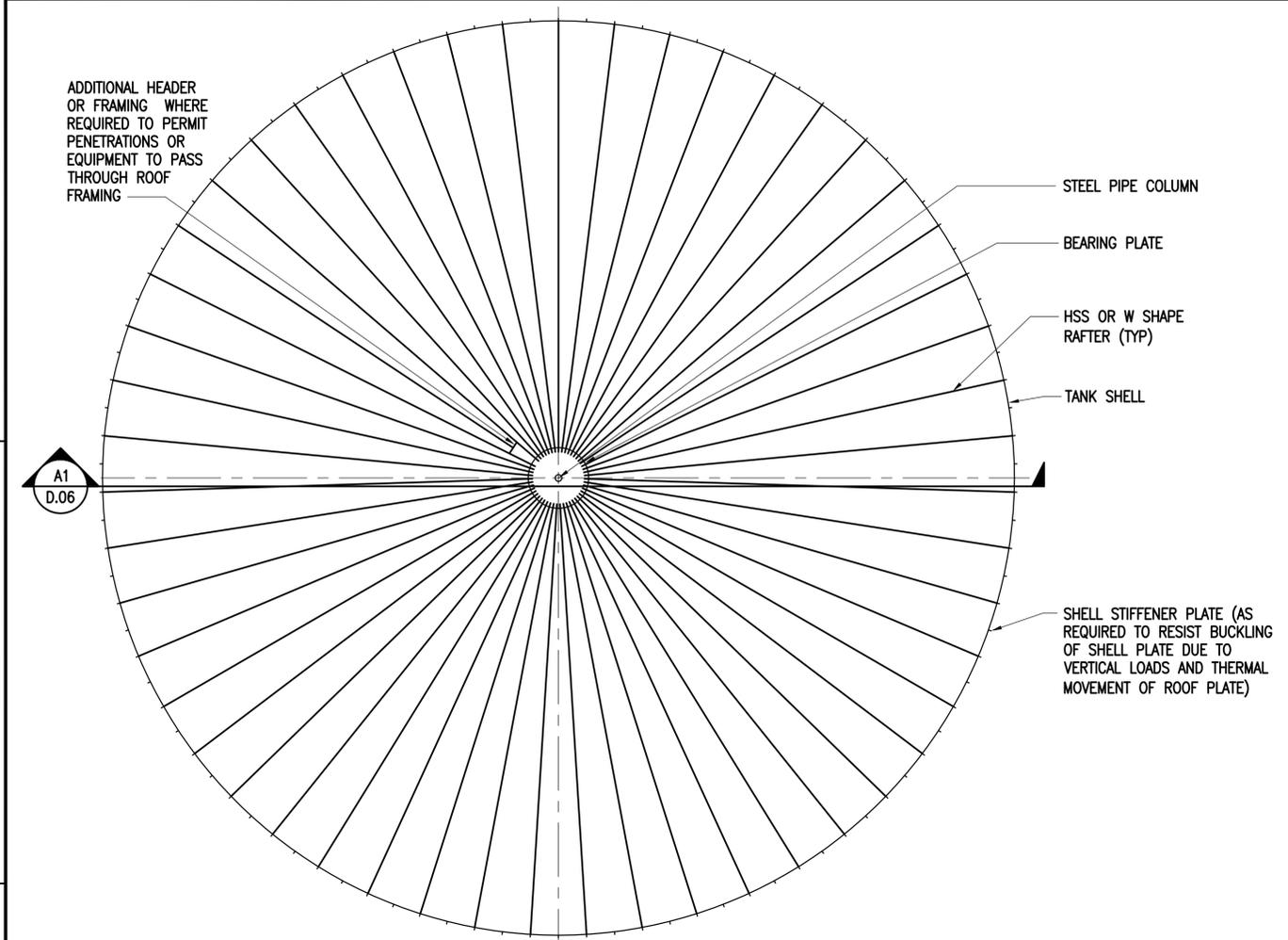
**ROOF SUPPORT PLAN - SINGLE COLUMN TANKS**
