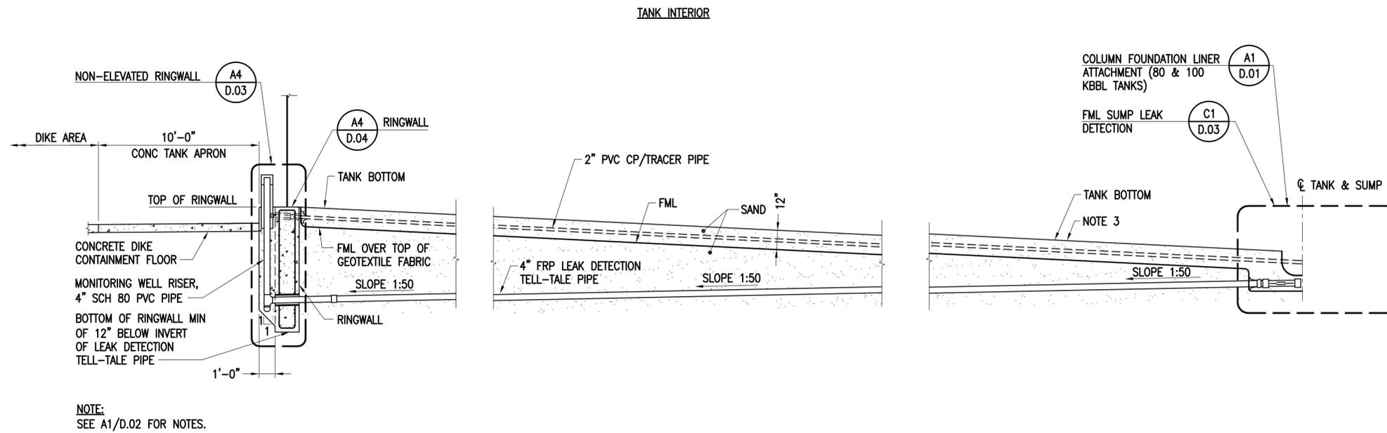
**SECTION - NON-ELEVATED TANK FOUNDATION** (C1)
