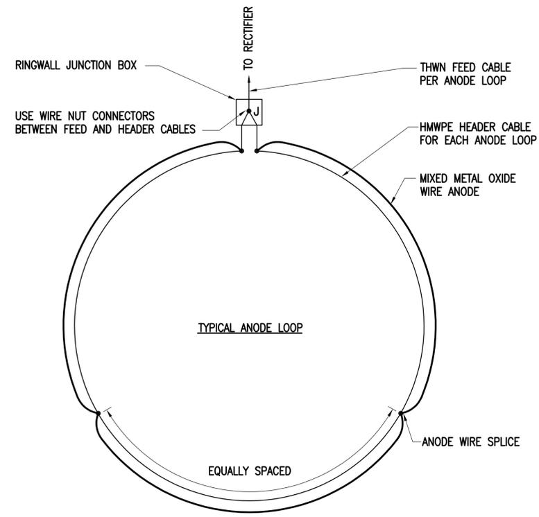
**TYPICAL ANODE LAYOUT AND SPLICING PLAN (C3)**
