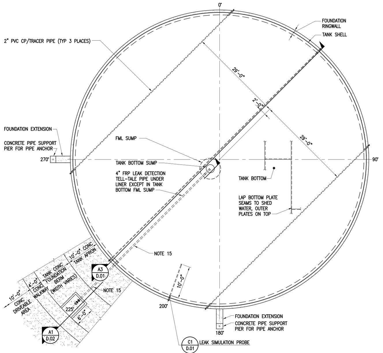
**40K BBL TANK BOTTOM, FOUNDATION, AND INTERSTITIAL PIPING PLAN**
