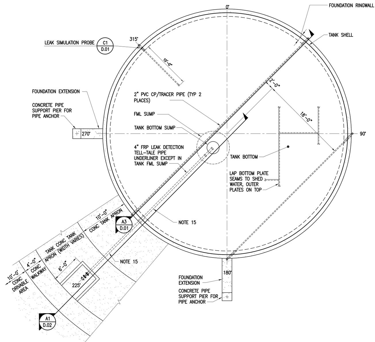
**10K BBL TANK BOTTOM, FOUNDATION, AND INTERSTITIAL PIPING PLAN**
