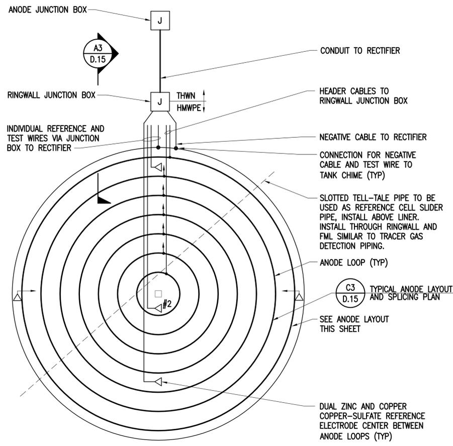
**TYPICAL CATHODIC PROTECTION LAYOUT-EXTERNAL BOTTOM**
