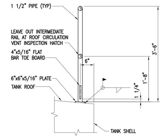
**ROOF PERIMETER GUARDRAIL** (A4)
