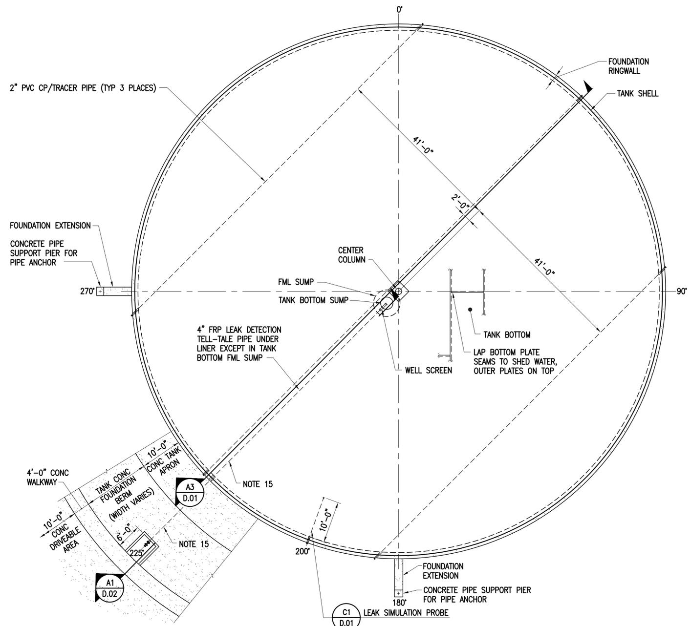
**100K BBL TANK BOTTOM, FOUNDATION, AND INTERSTITIAL PIPING PLAN**
