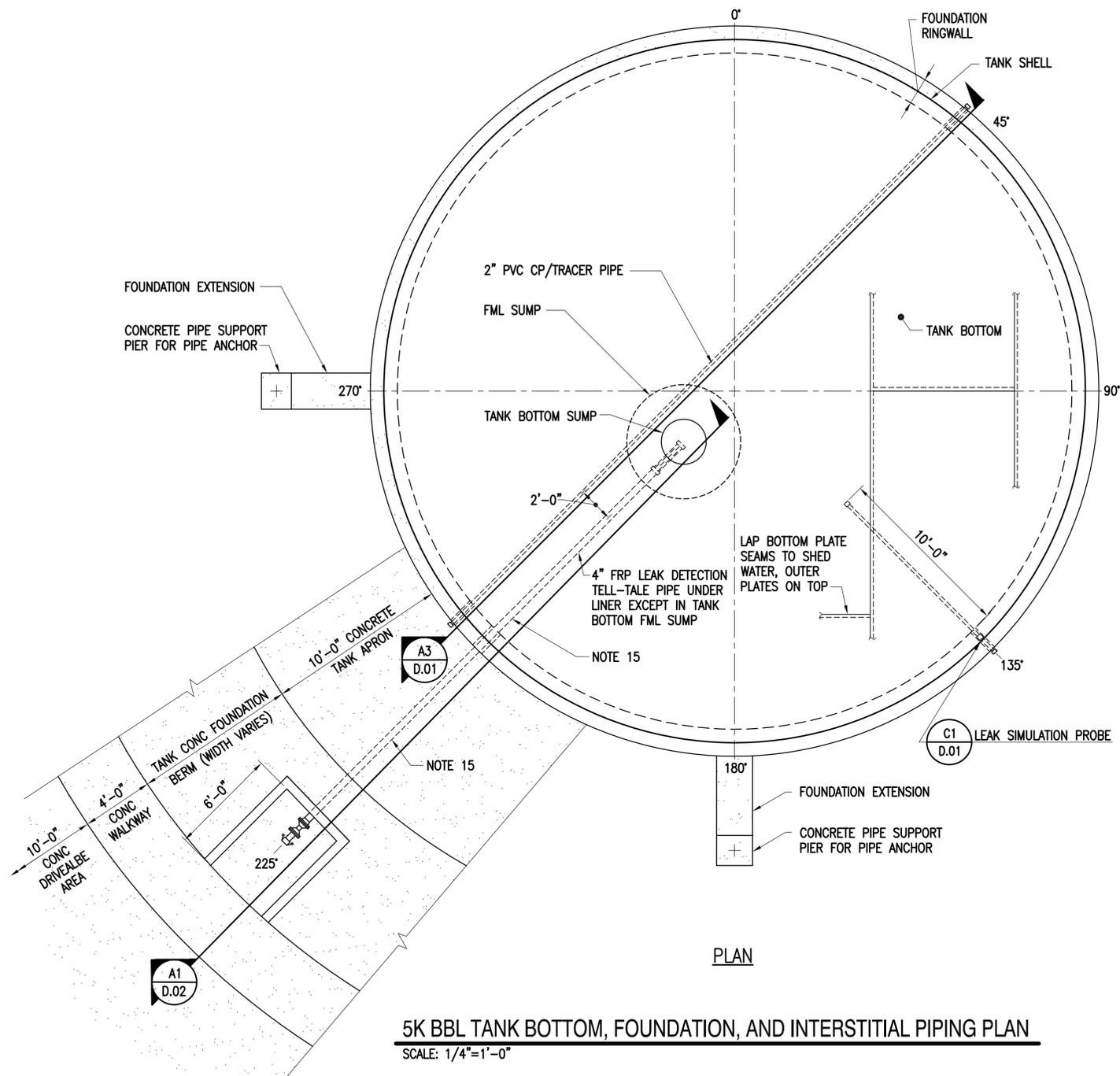
**5K BBL TANK BOTTOM, FOUNDATION, AND INTERSTITIAL PIPING PLAN**
