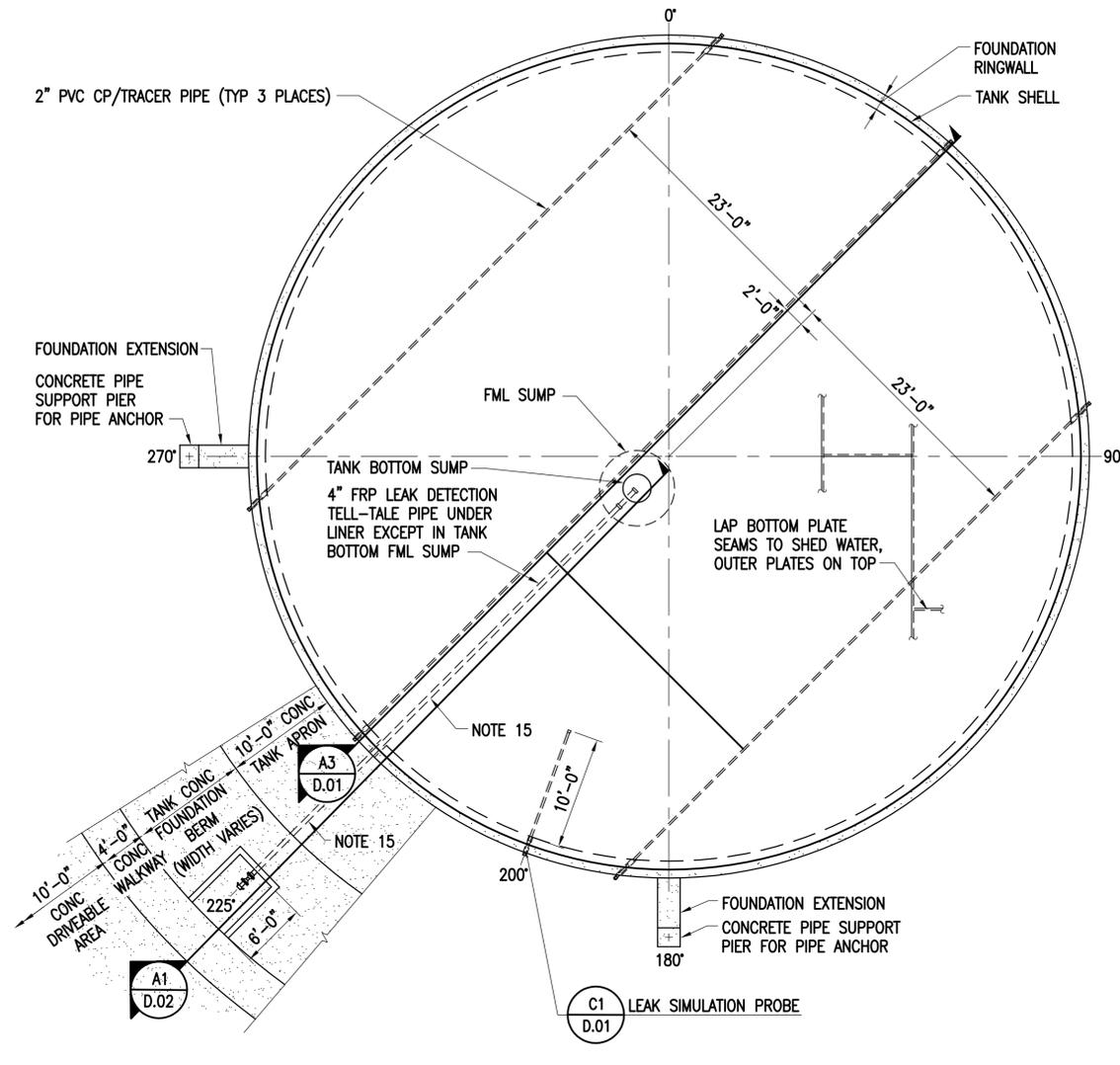
**30K BBL TANK BOTTOM, FOUNDATION, AND INTERSTITIAL PIPING PLAN**
