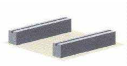
Pour-in-place Strip Footings With Keyway
