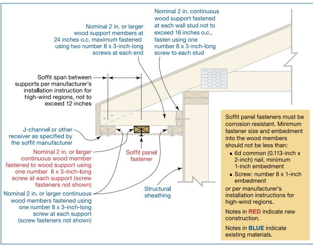
FIGURE 4-12: Typical soffit retrofit using wood supports
