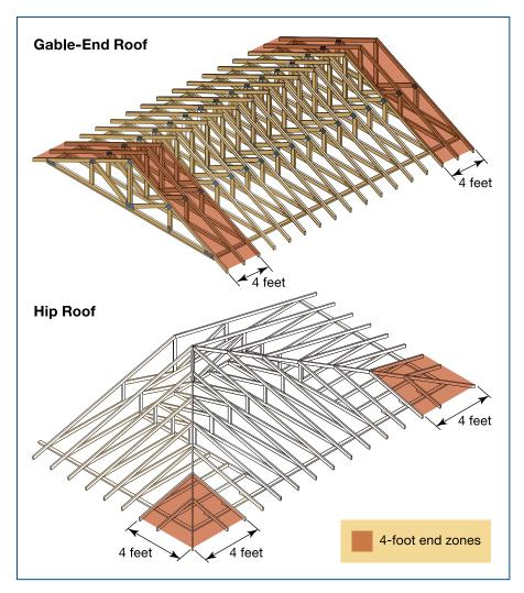
FIGURE 4-3: 4-foot end zones on gable and hip roofs
