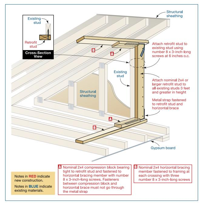
FIGURE 4-15: Conceptual gable end retrofit without overhangs
