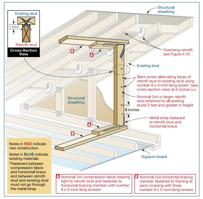
FIGURE 4-16: Conceptual gable end retrofit with overhangs
