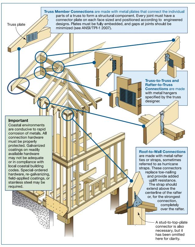
FIGURE 4-19: Load path connections of a roof system (SOURCE: FEMA 499)
