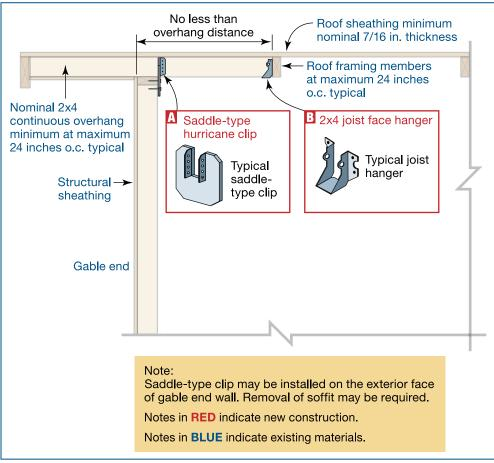
FIGURE 4-13: Bracing gable end overhangs
