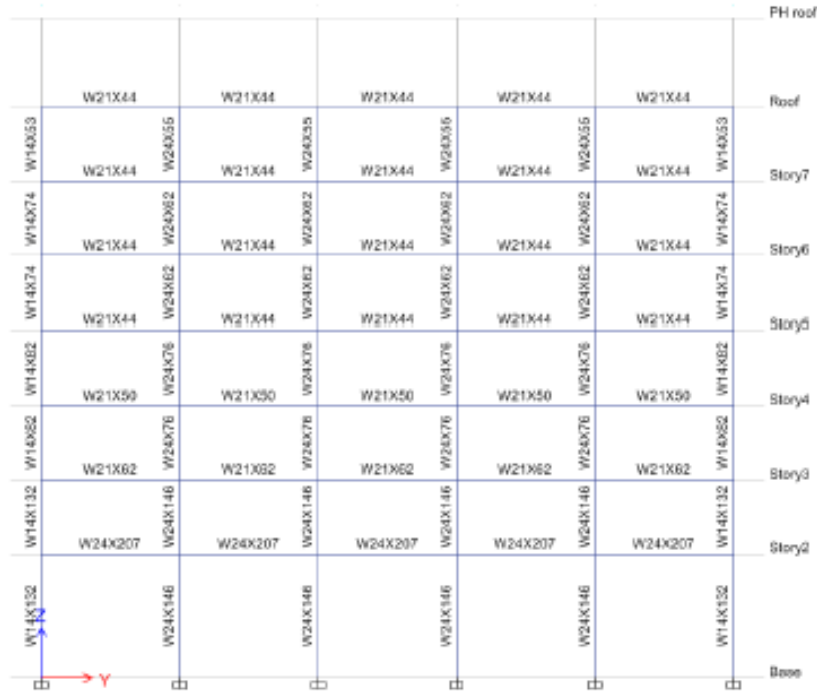
Figure 16.2-4 Steel Special Moment Frame on Gridlines A and H
