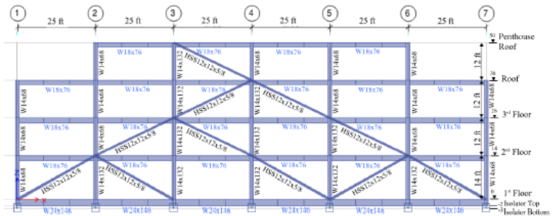
Figure 15.2-4 Longitudinal Bracing Elevation, Gridlines B and D
