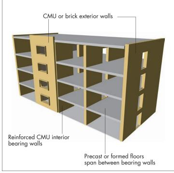
This building consists of reinforced masonry walls and concrete slab floors that may be either cast-in-place or precast. This building type is often used for hotel and motels and is similar to the concrete bearing-wall type C2.
