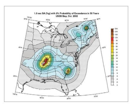
Figure 2-15: 1.0 second (long) period spectral acceleration values in %g with a 2% probability of exceedance in 50 years for central and southern United States.
