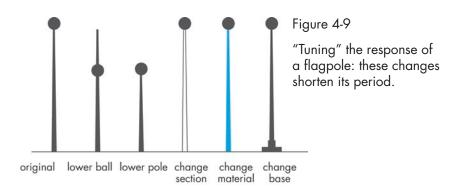
How does one "tune" a building, or change its period, if it is necessary to do so? One could change the natural period of a simple structure such as a flag pole by any or all combinations of the methods shown in Figure 4-9:
