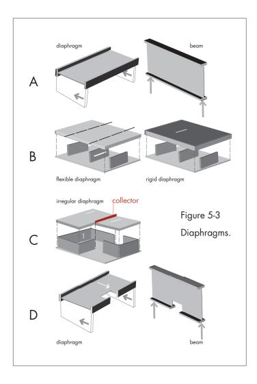
forces it is transmitting, also has a major influence on the nature and magnitude of those forces. With flexible diaphragms made of wood or steel decking without concrete, walls take loads according to tributary areas (if mass is evenly distributed). With rigid diaphragms (usually concrete slabs), walls share the loads in proportion to their stiffness (figure 5-3B).
