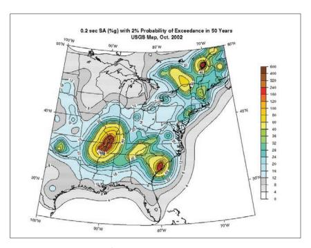
Figure 3-2: USGS Map of 0.2 sec spectural acceleration with a 2% Probability of Exceedance in 50 Years
