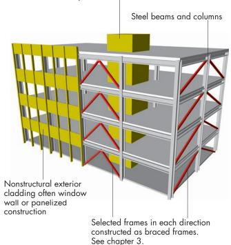
These buildings consist of a frame assembly of steel columns and beams. Lateral forces are resisted by diagonal steel members placed in selected bays. Floors are cast-in-place concrete slabs or metal deck and concrete. These buildings are typically used for buildings similar tos teel-moment frames, although are more often low rise.
