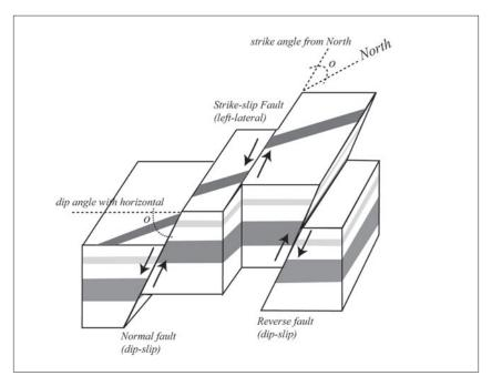
Figure 2-3: The three primary fault types.
