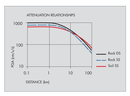
Figure 2-12: Examples of attenuation curves for a Mw7 earthquake obtained by data regression, illustrating the effects of a **site** type: rock (blue dashed) vs. deep soil (red), and **event** type: strike-slip fault (blue dashed) vs. reverse fault (black)
