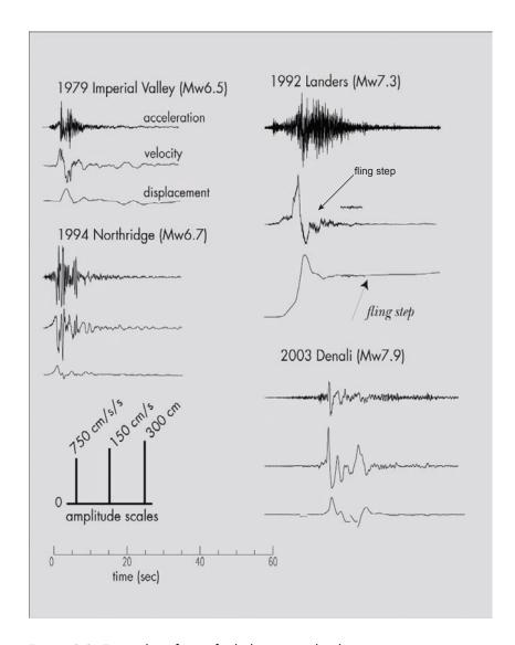
Figure 2-9: Examples of near-fault, large amplitude seismograms (time-histories).
