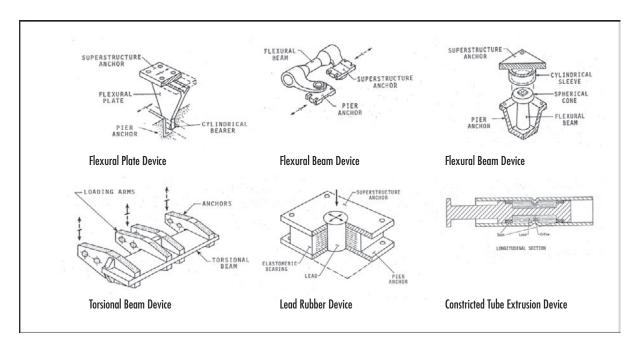
Figure 7-9: A set of energy dissipating devices.
