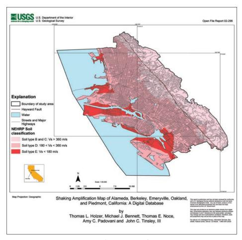
Figure 3-15: USGS Shaking Amplification Map of Alameda, Berkeley, Emeryville, Oakland and Piedmont, California.
