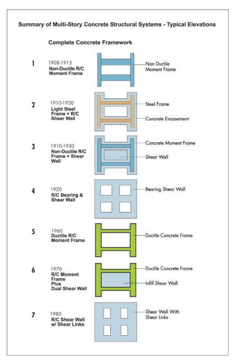
Figure 7-3: Concrete building frameworks
