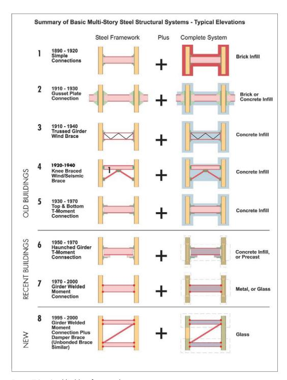
Figure 7-2: Steel building frameworks.
