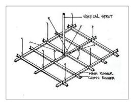
Figure 9-10: Suspended-ceiling seismic bracing.
