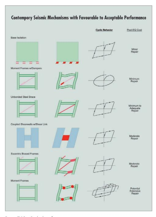
Figure 7-19: Six high-performance seismic structures.
