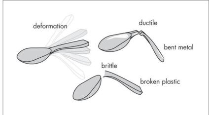
is rather like that of bending a spoon rapidly back and forth: the heavy structure is pushed back and forth in a similar way several times a second (depending on its period of vibration).
