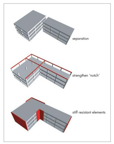
Figure 5-23 Solutions for the re-entrantcorner condition.
