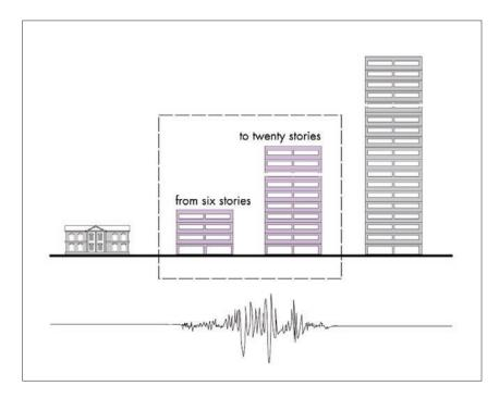
Figure 4-5: The vulnerable group: Mexico City, 1985. The periods of buildings in the 6 to 20 story range resonated with the frequency content of the earthquake.
