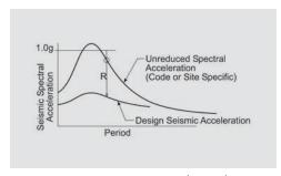
Figure 7-4: Design verses real acceleration.
