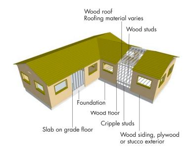
These buildings are generally single-family dwellings of one and two stories. Floor and roof framing consists of wood joists or rafters supported on wood studs spaced no more than 24 inches apart. The first floor may be slab on grade or wood raised above grade with cripple stud walls and post-and-beam supports. Lateral support is provided with shear walls of plywood, stucco, gypsum board, and a variety of other materials. Most often there is no engineering design for lateral forces.
