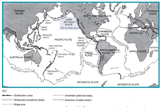
Figure 2-2: The major tectonic plates, midoceanic ridges, trenches and transform faults.
