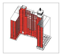
5. **Seismic isolation**, developed in the early 1980s, is a completely different and reliable concept, in which the building structure is supported on isolation bearings and is effectively separated from the ground, significantly reducing seismic response.
