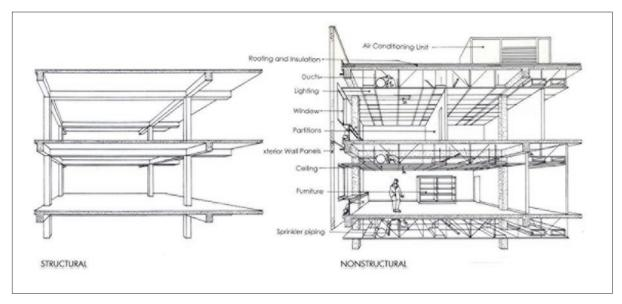
Figure 9-3: The basic structural system (left) and the nonstructural components (right).
