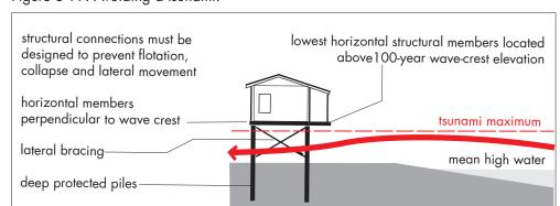
Figure 3-19: Avoiding a tsunami.
