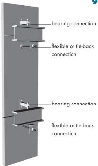
Figure 9-8: Typical push-pull connection for precast panel.
