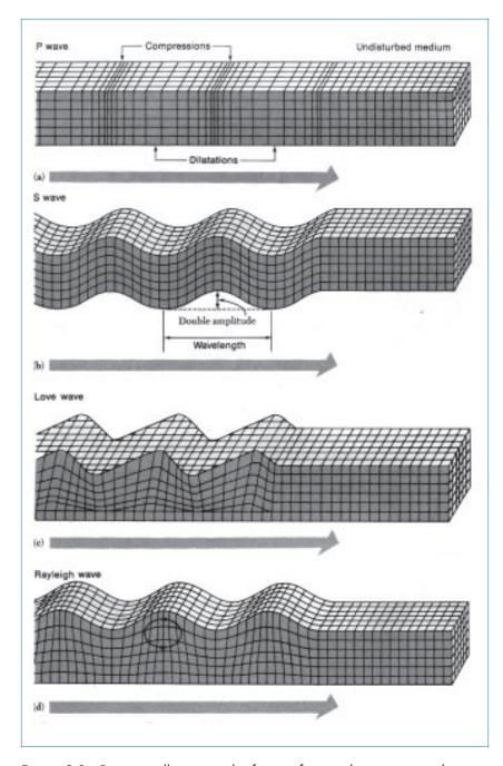
Figure 2-8: Diagram illustrating the forms of ground motion near the ground surface in four types of earthquake waves.
