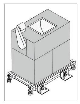
Figure 9-18: Vibration-isolated chiller with snubbers to restrict lateral movement (Mason Industries Inc).
