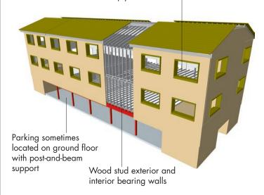
These buildings are framed with the same systems as W1 buildings but are most often multiple-story large residential-type structures, and, unless very old, are engineered. A common seismic deficiency is the tuck-under parking at the ground story that creates a soft or weak story. This building type is also often built on top of a one story concrete parking structure.
