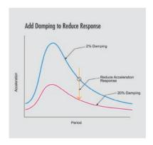
Figure 7-17: Reduction of demand by damping.
