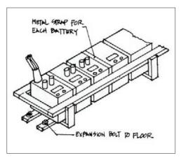
Figure 9-19: Emergency power battery rack support.
