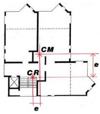
Figure 5-16: Left, the building after the earthquake. Right, typical floor plan showing the Center of Mass (CM), Center of Resistance (CR), and Eccentricity (e) along the two axes. PHOTO SOURCE: EERI
