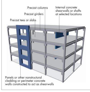
These buildings consist of concrete columns, girders, beams and/or slabs that are precast off the site and erected to form a complete gravity-load system. Type PC2 has a lateral force-resisting system of concrete shear walls, usually cast-in-place. Many garages have been built with this system The building type is most common in moderate and low seismic zones and could be used for many different occupancies in those areas.
