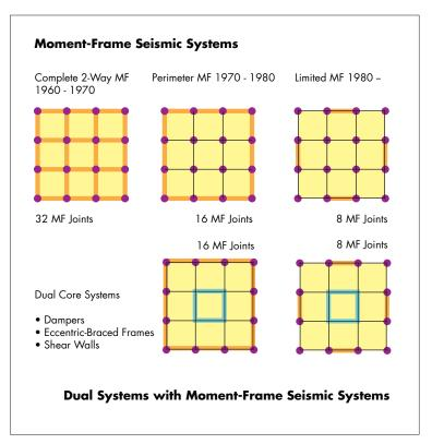
Figure 7-18: Single and multiple system concepts.
