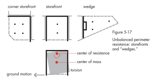
A common instance of an unbalanced perimeter is that of open-front design in buildings, such as fire stations and motor maintenance shops in which it is necessary to provide large doors for the passage of vehicles. Stores, individually or as a group in a shopping mall, are often designed as boxes with three solid sides and an open glazed front (Figure 5-17).
