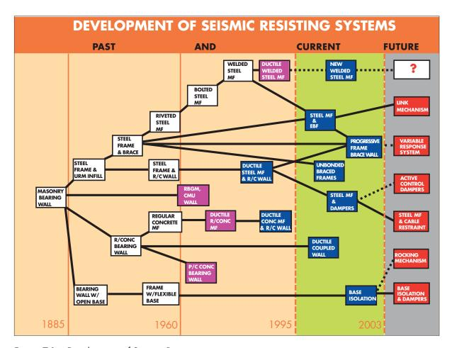
Figure 7-1: Development of Seismic Resisting Systems.
