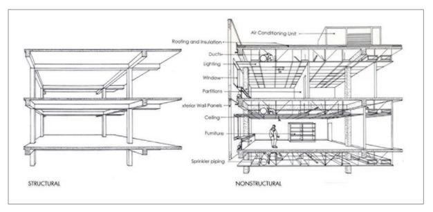
Figure 4-18: Structure (left), nonstructural components and systems (right).
