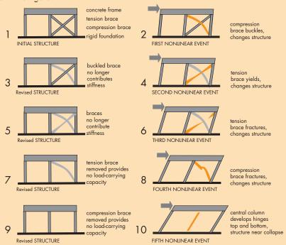
In current engineering practice, pushover analysis is more commonly used to evaluate the seismic capacity of existing structures and appears in several recent guidelines for seismic design concerning existing buildings. It can also be a useful design tool for the performance-based design of new buildings that rely on ductility or redundancies to resist earthquake forces.
