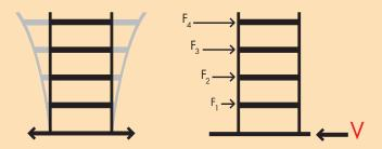
The tendency for the building to sway from side to side in response to ground motion produces greater accelerations in the upper parts of the building. This back and forth motion is called the fundamental mode, which dominates the response of most regular building structures. To model this effect statically, the equivalent lateral force procedure redistributes the load applied to the buildings floors to account for their distance from the base.
