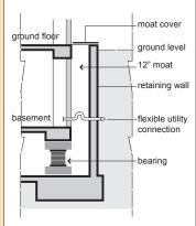
For the bearings to work properly, it was necessary to isolate the building from the ground horizontally. To do this, a retaining wall was constructed around the building perimeter with a 12-inch seismic gap (or moat), so that the building was free to move relative to the surrounding ground.
