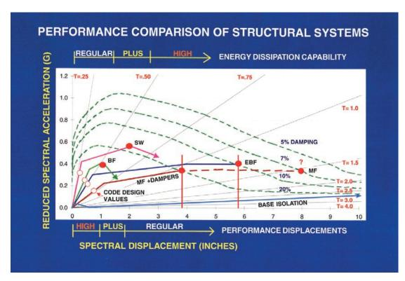
Figure 7-7: Performance characteristics of structural systems.
