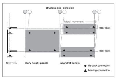
Figure 9-9: Connection types and locations for precast panels.
