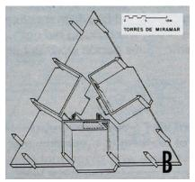
Figure 5-12: This apartment house appears to have a soft first story (Figure 5-12A), but the lateral force-resisting system is a strong internal shear wall box, in which the shear walls act as party walls between the dwelling units (Figure 5-12B). The architect achieved a light and elegant appearance, and the engineer enjoyed an optimum and economical structure.
