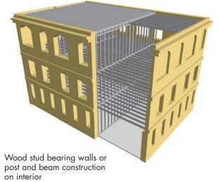
Wood joists bearing on masonry wall
