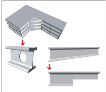
can transfer forces across the intersection area, but only if the design allows for these beam-like members to extend straight across without interruption. If they can be accommodated, full-height continuous walls in the same locations are even more effective. Since the portion of the wing which typically distorts the most is the free end, it is desirable to place stiffening elements at that location.
