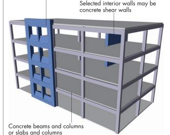
Concrete shear walls are concrete walls in a building design to provide lateral stiffness and strength for lateral loads. There are two main types of shear-wall buildings, those in which the shear walls also carry the gravity loads (with bearing walls), and those in which a column-supported framing system carries the gravity loads (with gravity frame).
