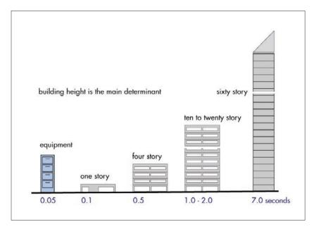
Figure 4-4: Comparative building periods, determined by height. These values are approximations: the structural system, materials, and geometric proportions will also affect the period.
