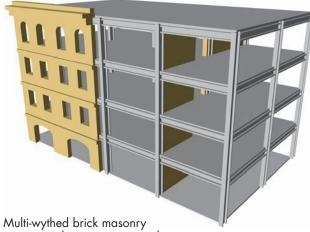
exterior with one or more wythes built within the column/beam envelope as 'infill'
