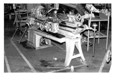
Figure 9-22: This lathe lifted up in the air and came down about four inches from its starting point before sliding another six inches, where it finally came to rest in the 1983 Coalinga earthquake. The initial complete lifting off the floor is evidence of vertical acceleration of more than 1g.
