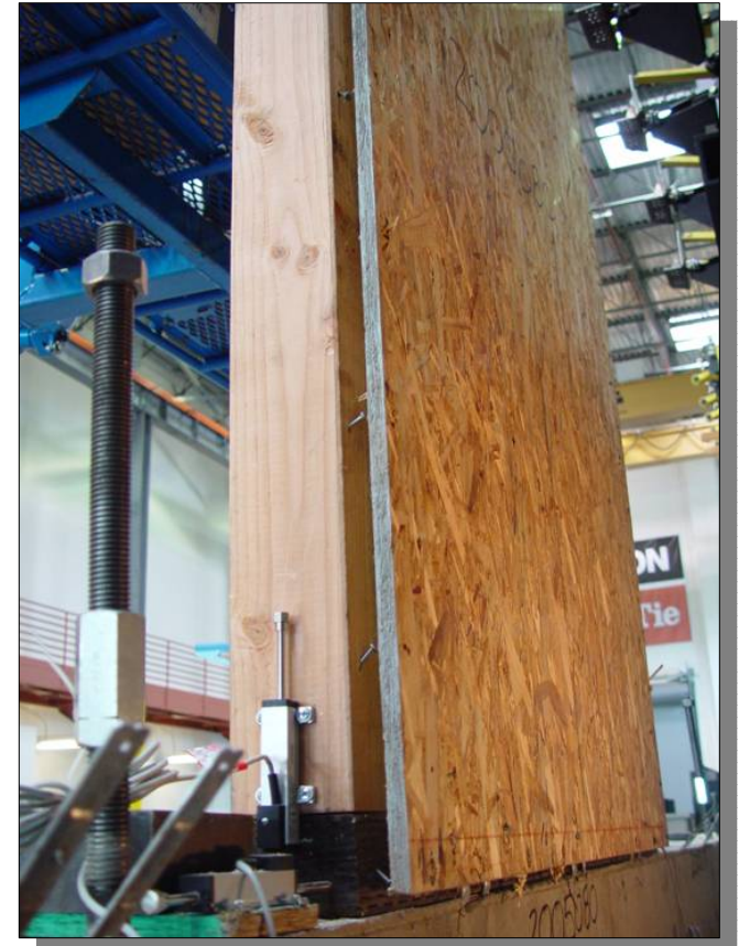
Vertical element: nailed wood structural panel diaphragm
