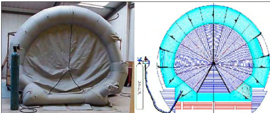
**Figure 4-3:** The “Tunnel Plug” is an example of an innovative fire suppression system under development for tunnels. Funded by DHS S&T, the plug is designed to drop from the ceiling and inflate inside the tunnel, essentially sealing off the passageway and preventing smoke or fire from spreading.
