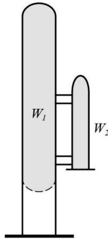
Figure C15.1-7 Torsional irregularity.
