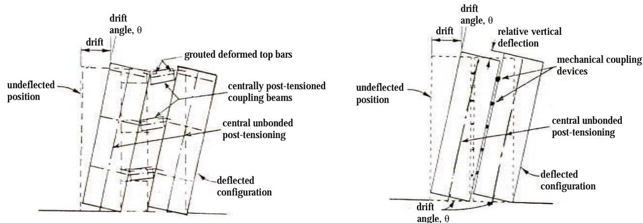
Figure C14.2.4.5.1 (a) Coupled wall test module with coupling beams;
