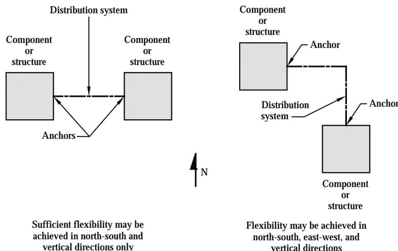
Figure C13.2-1 Schematic plans illustrating branch line flexibility.
