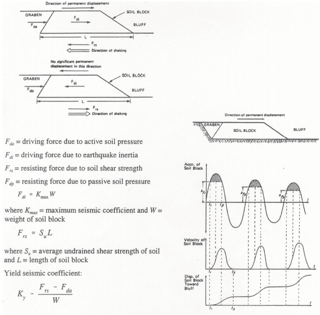
Figure 1 Forces and equations used in analysis of translatory landslides for calculating permanent lateral displacements from earthquake ground motions (National Research Council, 1985 from Idriss, 1985).
