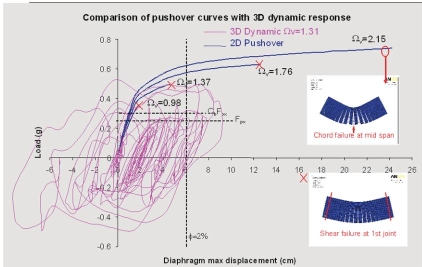
Figure A3-4 Superposition of 3D-FE global E demand results on 2D pushover.
