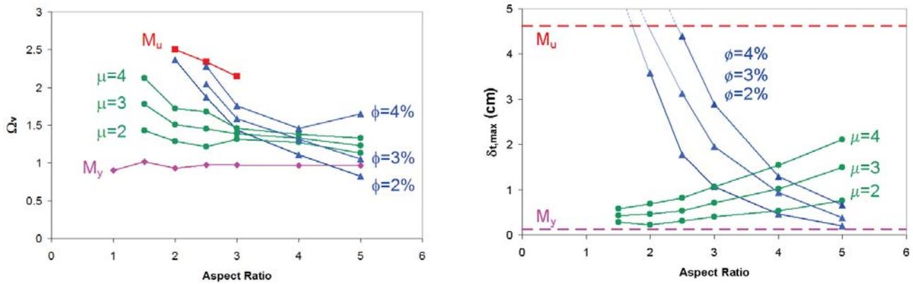
Figure A3-2 Design charts  $\Omega$  vs. aspect ratio (left) and deformation capacity vs. aspect ratio (right).
