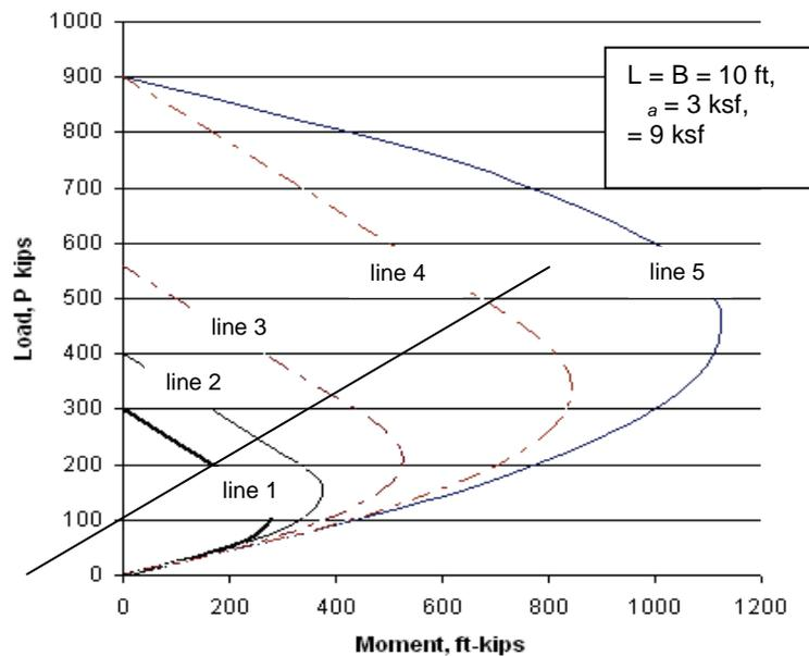
Figure 6 Example interaction curve for a shallow foundation.
