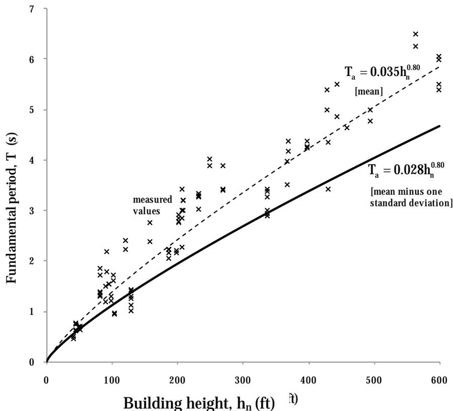
Figure C12.8-2 Variation of fundamental period with building height.
