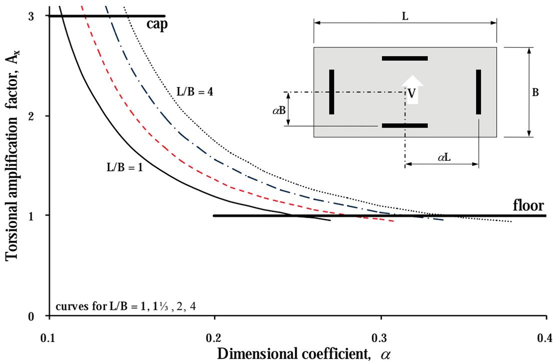
Figure C12.8-5 Amplification factor for symmetric rectangular buildings.
