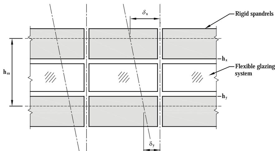
Figure C13.3-3 Displacements over less than story height.
