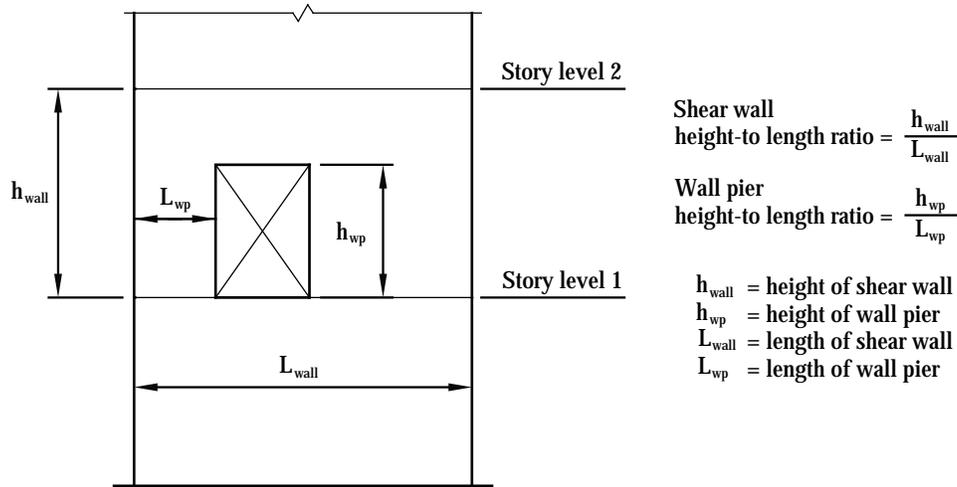
Figure C12.3-4 Shear wall and wall pier height-to-length ratios.
