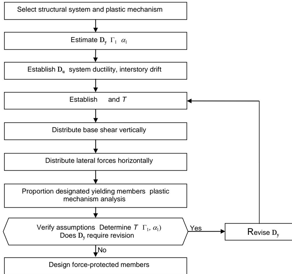
Figure 2 Steps in the design process.
