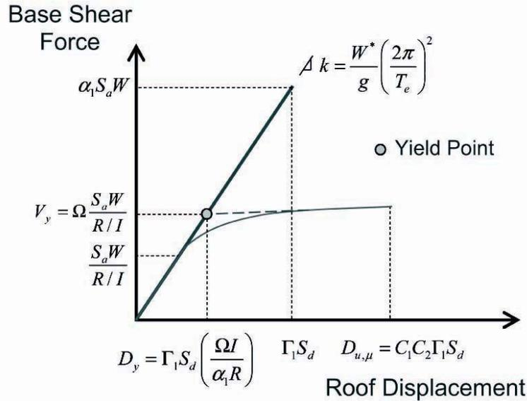
Figure 5 Response of elastic and yielding MDOF systems in the first mode. The yield point identifies the change in slope of a bilinear curve that is fitted to the capacity curve over the applicable range of displacement response.  $\Omega$  represents the actual overstrength factor, not the value  $\Omega_0$  provided in the 2003 R
