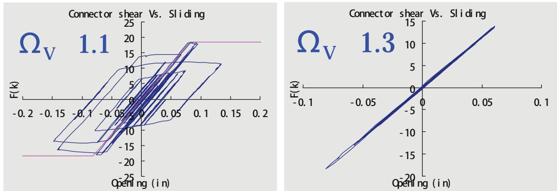
Figure A3-5 Sample results for critical shear connector,  $\Psi = 1.5$  Berkeley MCE (a)  $\Omega_v = 1.1$ , (b)  $\Omega_v = 1.3$ . deformation demand.
