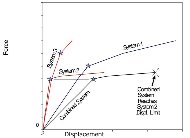
Figure 2 Force versus displacement of series-connected elements.
