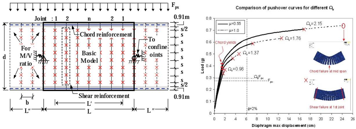
Figure A3-1 Schematic of 2D FE model (left) and sample results for diaphragm shear overstrength factor  $\Omega$ .
