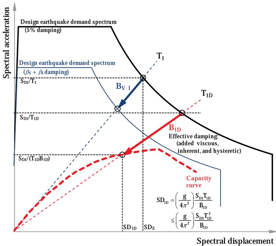
Figure C18.4-1 Effective damping reduction of design demand.
