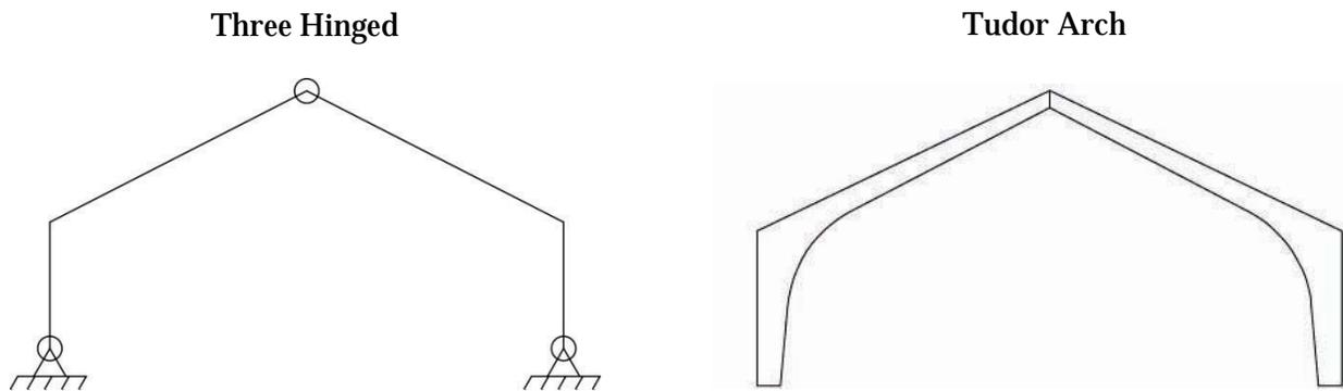
Figure C1.0 Three-hinge arch and Tudor arch configurations.
