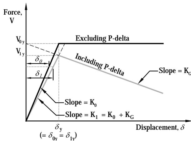
Figure C12.8-7 P-delta effect on a simple structure.
