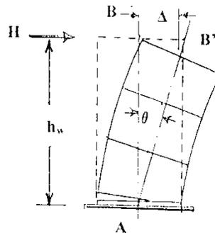
Figure C14.2.4.2.2-1 Definition of drift ratio  $\theta$ .
