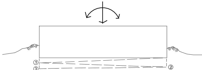
Figure 4 Progressive settlement during repeated cycling.
