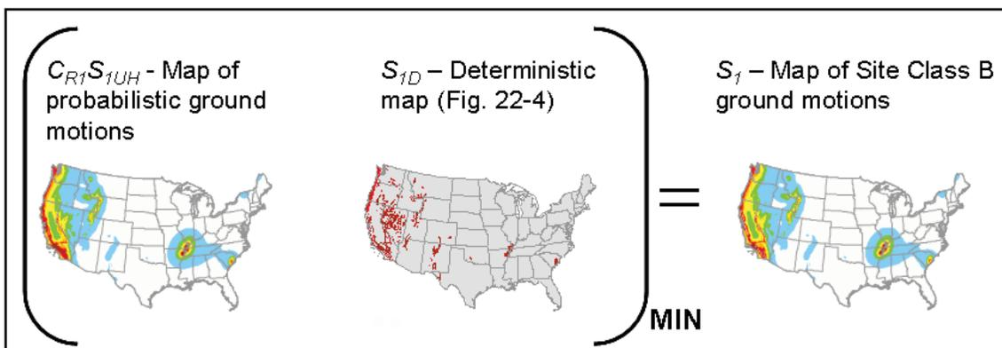
Step 3 – Adjust Site Class B ground motions for site conditions (e.g., Site Class D)
