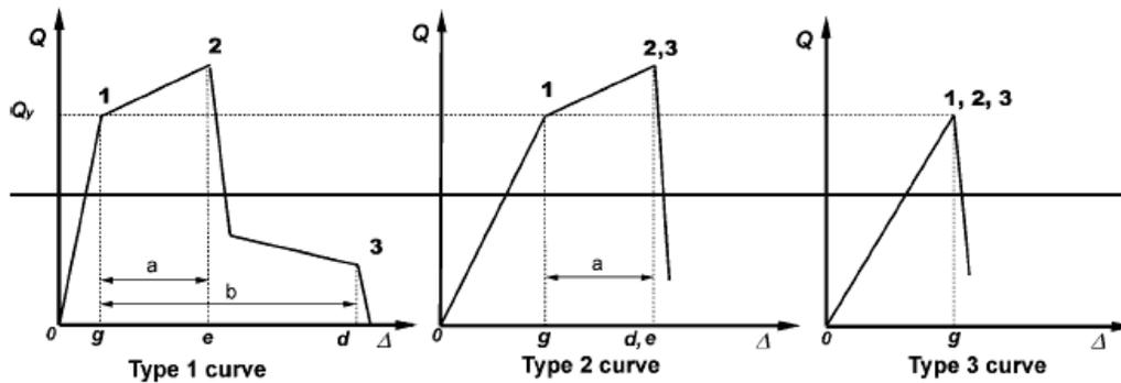
Figure A4-1 Connection classification per ASCE/SEI 41 procedures.
