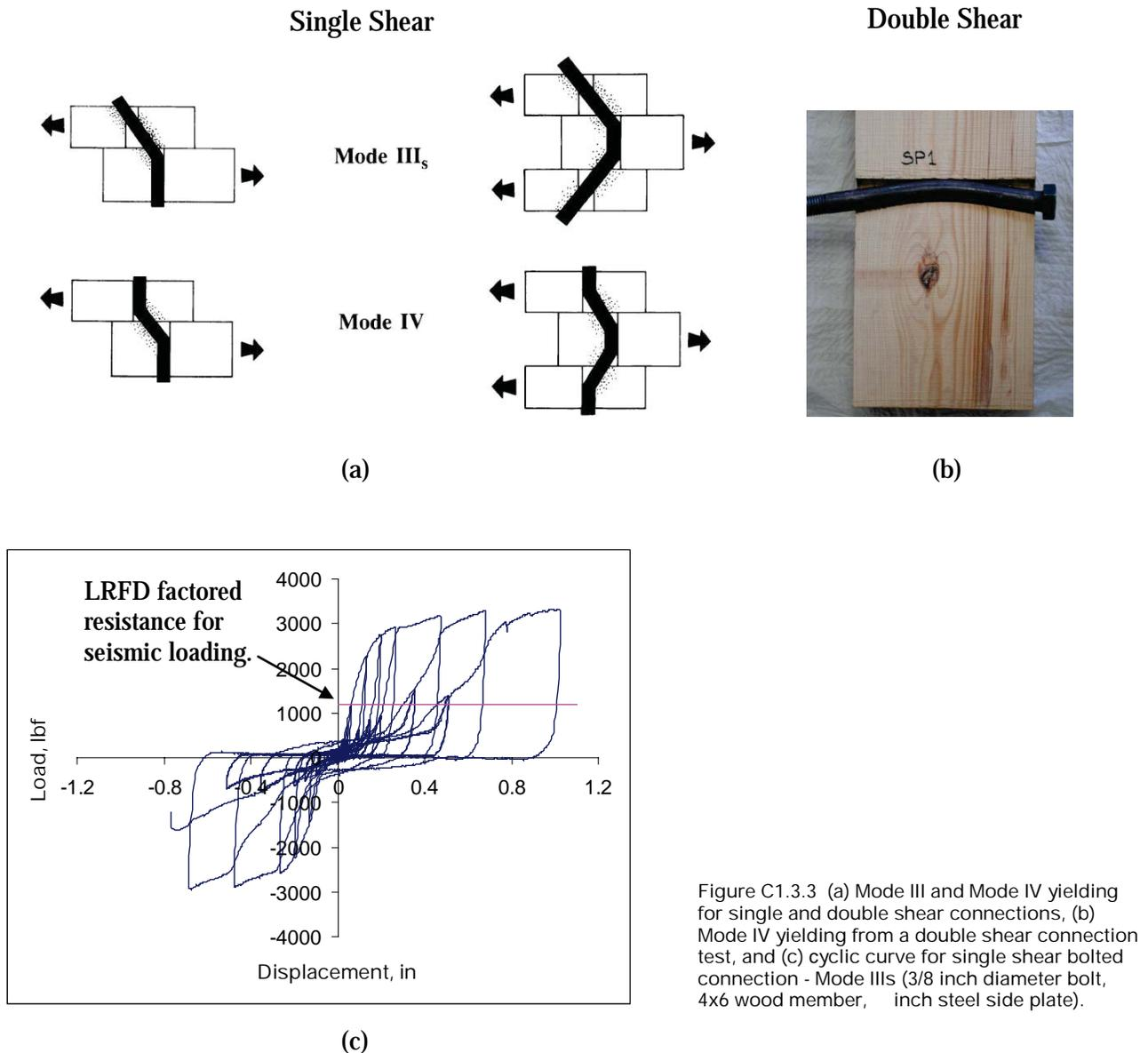
Figure C1.3.3 (a) Mode III and Mode IV yielding for single and double shear connections, (b) Mode IV yielding from a double shear connection test, and (c) cyclic curve for single shear bolted connection - Mode III<sub>s</sub> (3/8 inch diameter bolt, 4x6 wood member, 1/2 inch steel side plate).
