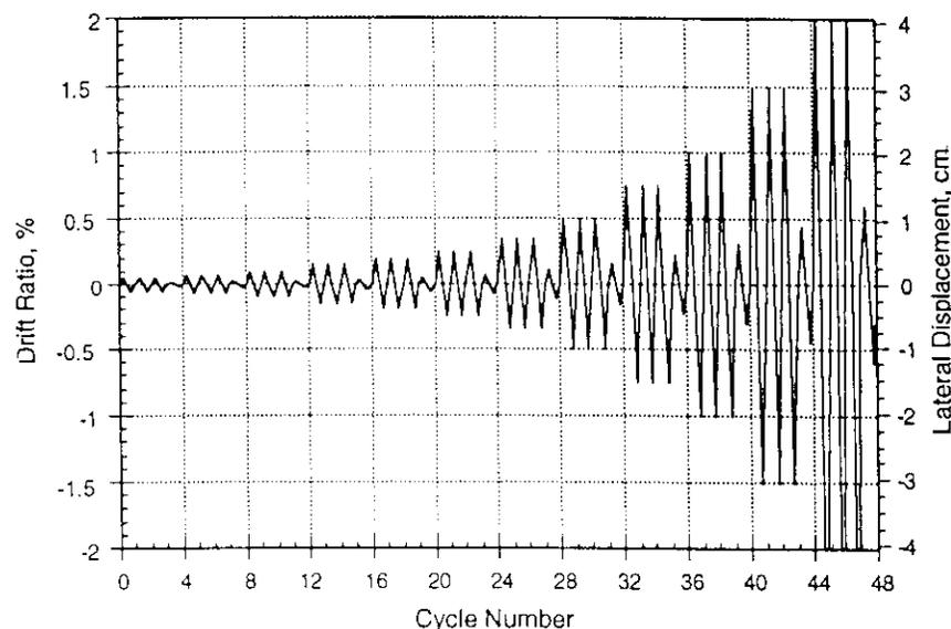
Figure C14.2.4.7 Example of specified test sequence.
