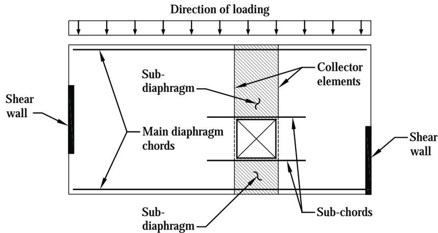
Figure C12.10-1 Diaphragm components.
