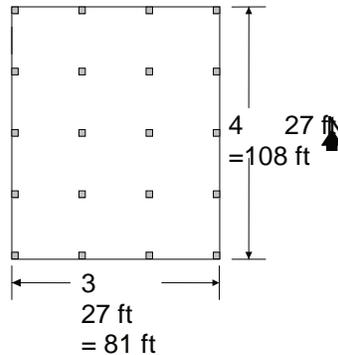
Figure 11 Plan view of reinforced concrete frame building.
