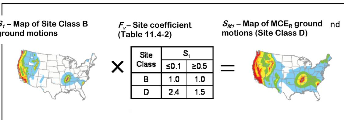
Figure C11.4-1 Illustration of process for developing 1-second MCE<sub>R</sub> Site Class D ground motions using formulas of Section 11.4.3 and associated mapped values of ground motions and risk coefficients of Chapter 22.
