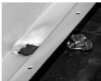
Failure of sheet metal base anchored with standard washer (With permission)
