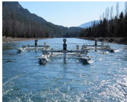
(b) Hydrokinetic free-flowing river application<sup>2</sup>
