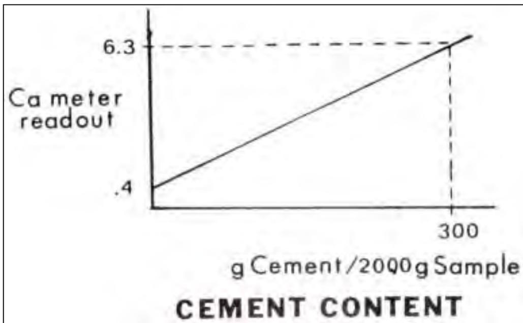
Fig. 5. Calibration Graph for Procedure B
