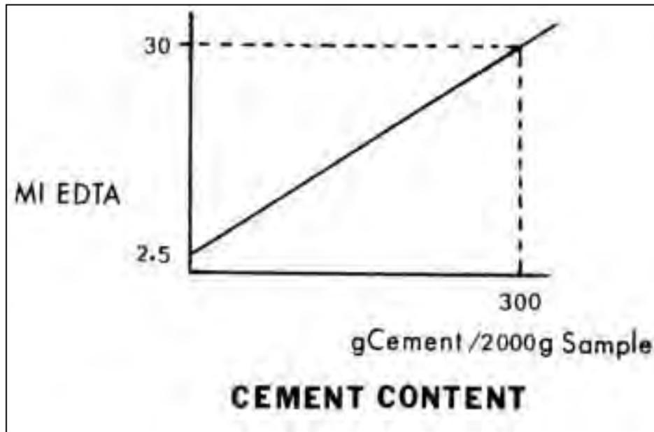
Fig. 3. Calibration Graph for Procedure A
