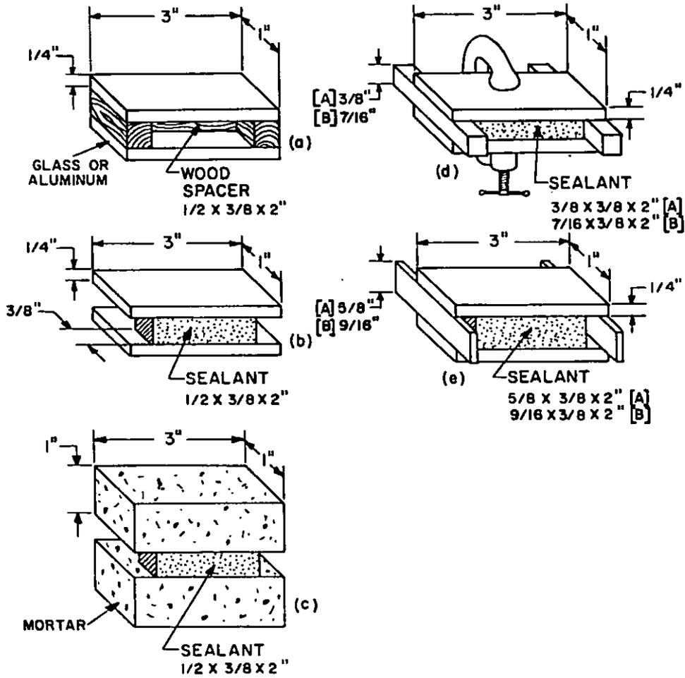
FIGURE 7. Test specimens used in Durability test
