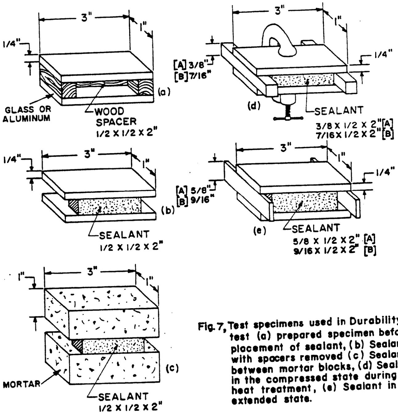
**Fig. 7, Test specimens used in Durability test (a) prepared specimen before placement of sealant, (b) Sealant with spacers removed (c) Sealant between mortar blocks, (d) Sealant in the compressed state during heat treatment, (e) Sealant in the extended state.**
