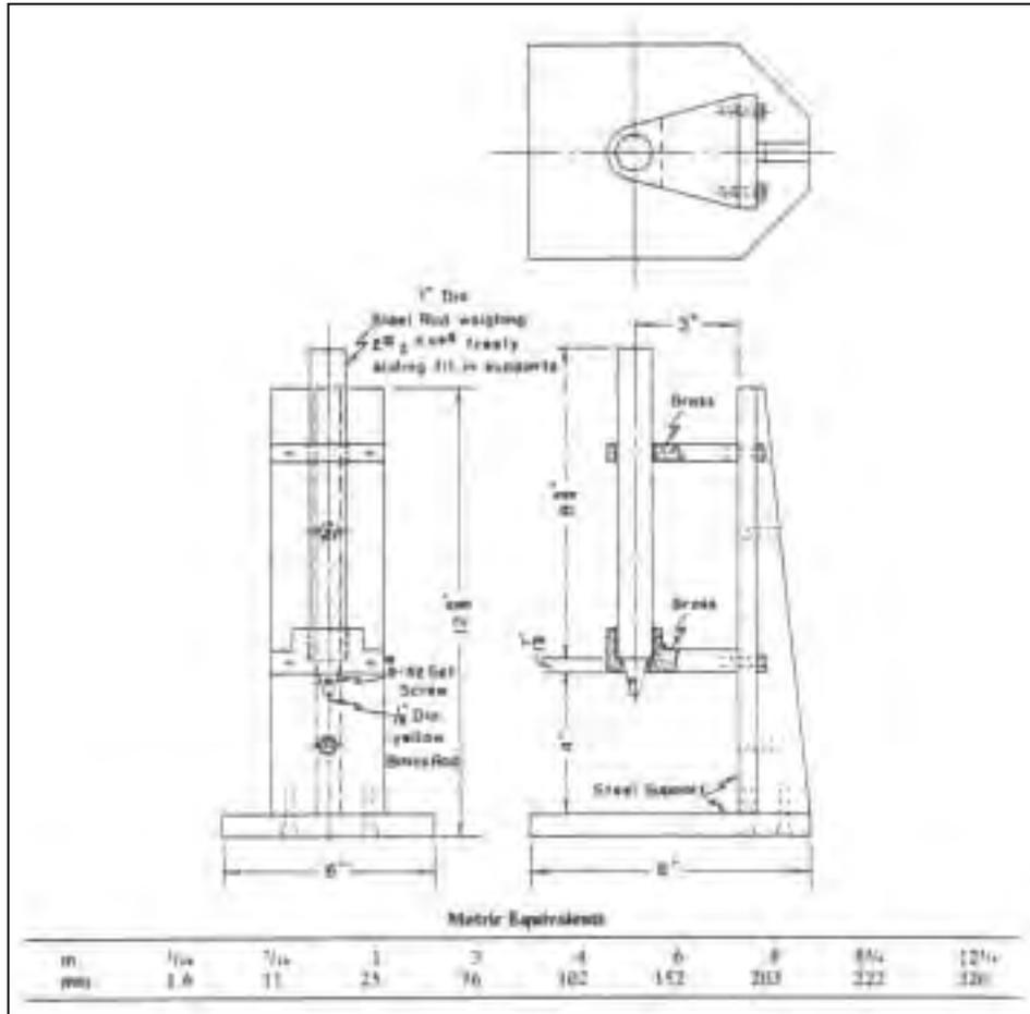
Fig. 1. Apparatus for Scratch Hardness Test
