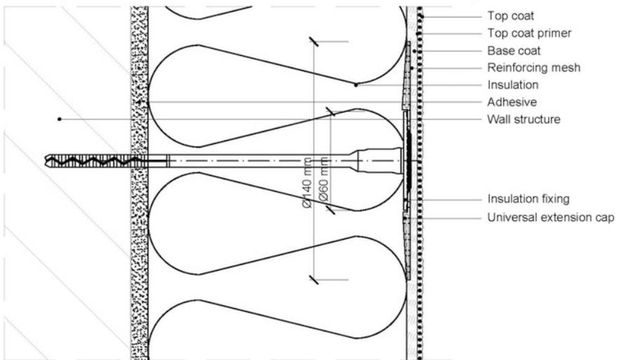
**Bonding of wool boards with laminar (parallel to board surface) arrangement of fibers. Full surface method.**
