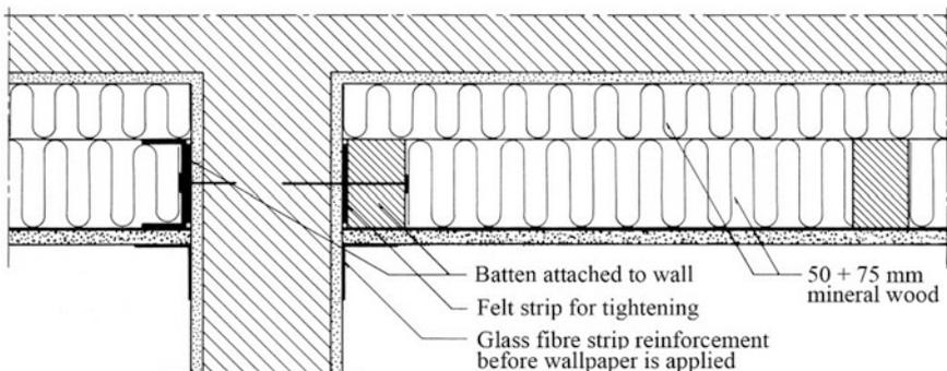
**Fig. 6.3** Detail of internally insulated façade around adjoining partition (perpendicular to façade)
