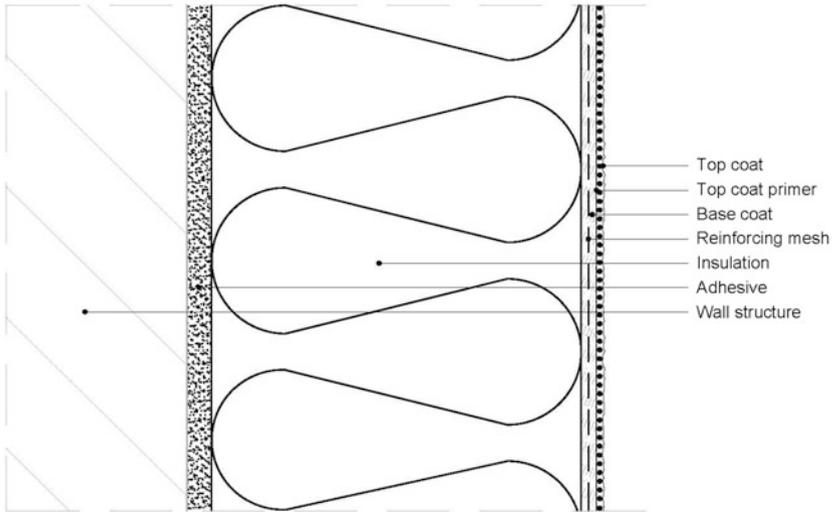
B) Fully bonded ETICS with additional mechanical fixing.
