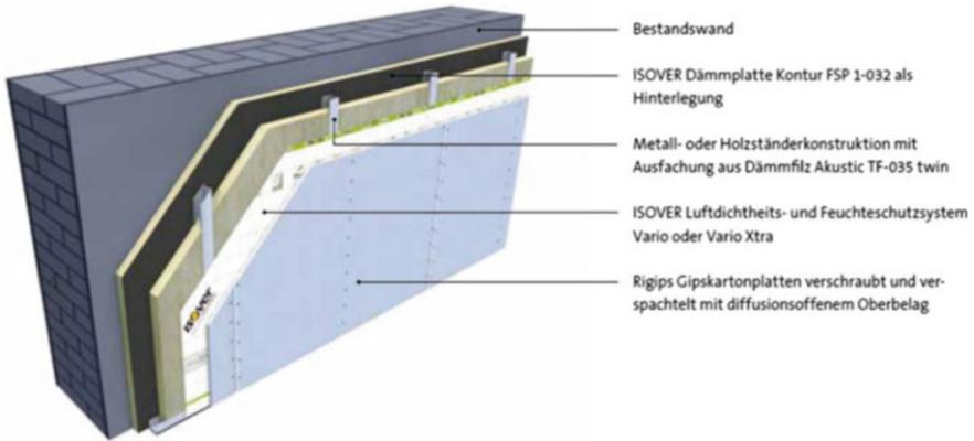
(1) Existing wall; (2) first mineral wool insulation layer (boards) to prevent thermal bridges; (3) metal or wooden studs as substructure, flexible mineral wool batts in between; (4) vapor barrier with flexible density (smart vapor retarder); (5) gypsum boards, open to diffuse
