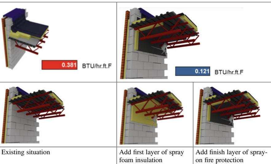
**Parapet with OWSJ and a Deck (Interior Wall Insulation)**
