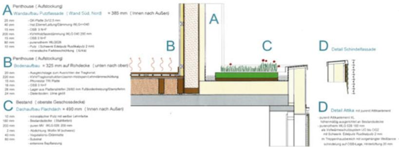
**Cross-section through the roof layout (C)**
