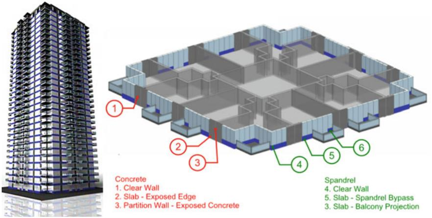
**Fig. 8.14** Example of calculation of the overall heat transmission rate of any specific part of the enclosure by summing the heat transmission from each element
