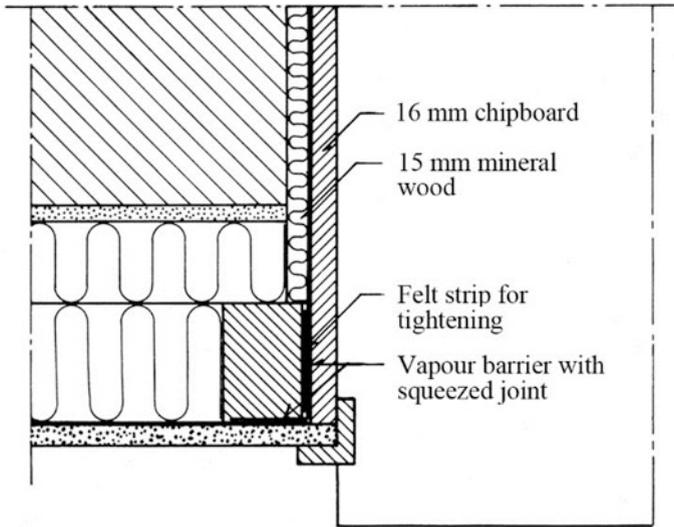
**Fig. 6.4** Additional insulation placed behind new opening reveal linings to reduce cold bridges around windows
