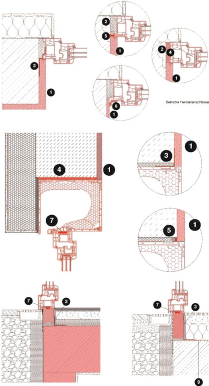
**Fig. F.24** Floor-length windows, French doors in the wall: (1) interior plaster, (2) smooth finish. (If needed) alternatives: (3) foil joint seals, (4) proofed sealant strips, multifunctional sealant strips, (5) spray sealant, (6) bands with sealant strips, (7) sealant for windowsill junction profile for windows, (8) floor recess section, (9) building component sealant
