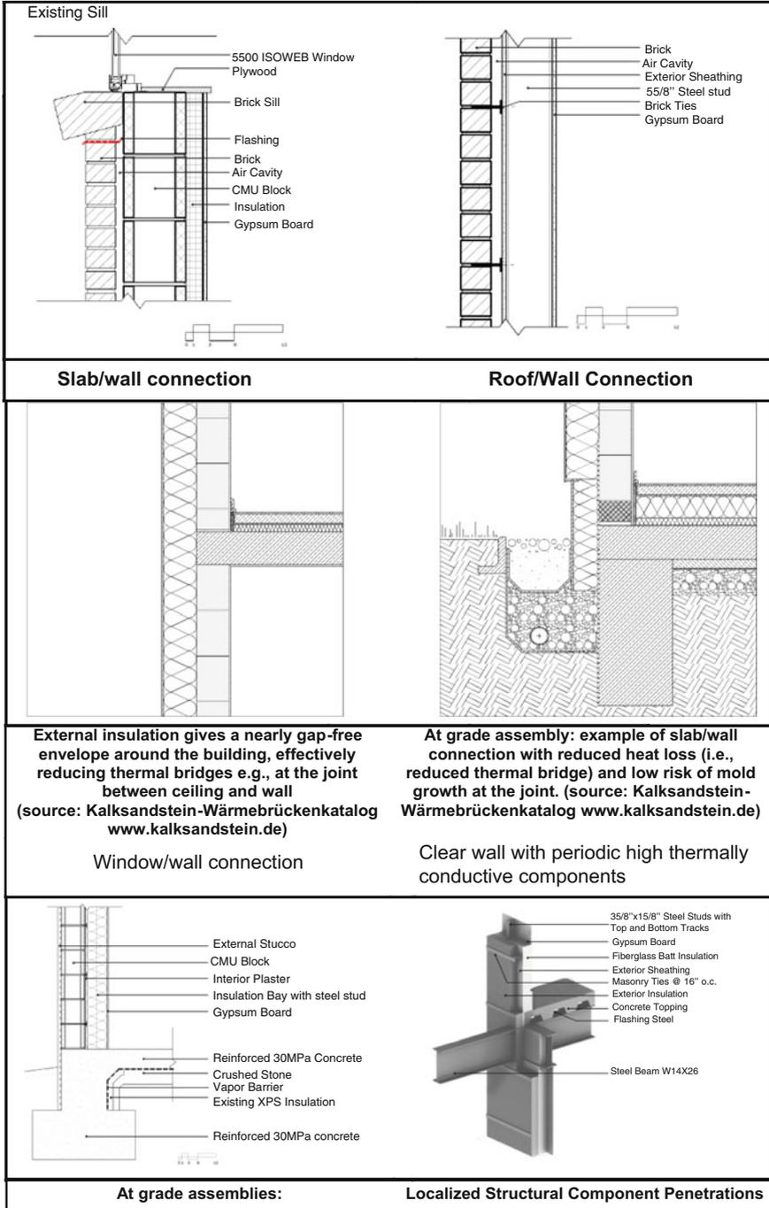
Fig. 8.7 Examples of thermal bridges
