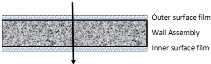
**Fig. 6.1** Simplified schematic of heat transfer through wall (roof) assembly
