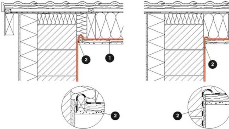
**Fig. F.11** Verge – between-rafter insulation: (1) air barrier, (2) adhesive, adhesive tape, pressure plates if necessary
