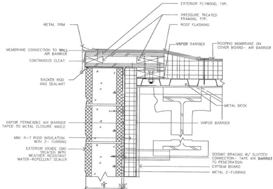
**Fig. F.5** Details of external air barrier single wythe concrete block with R-7 interior insulation. Commercial grade spun-bonded polyolefin air barrier, rigid insulation, vapor barrier, interior drywall: (a) roof edge; (b) parapet; (c) floor slab; (d) single wythe CMU; (e) window jamb; (f) window sill; (g) foundation
