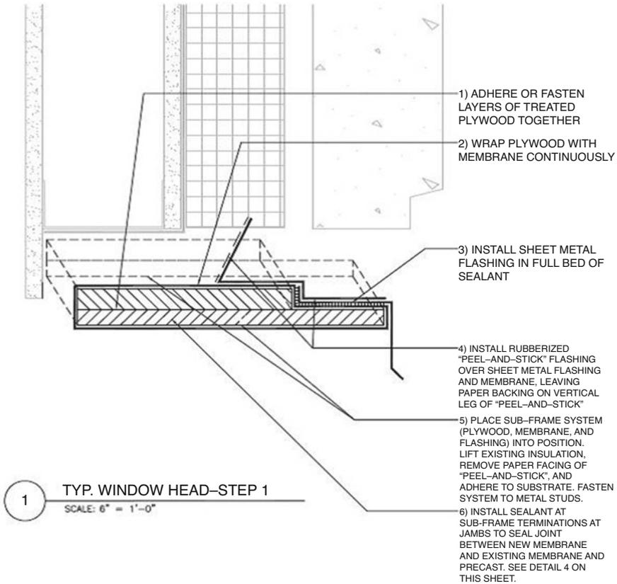
**Fig. E.5** Step-by-step illustration of window head installation (Step 1)
