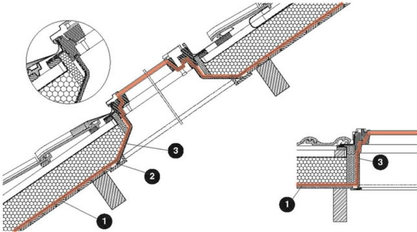
**Fig. F.9** Roof with skylights – above rafter: (1) air barrier, (2) tape, corner tape, (4) skirt board
