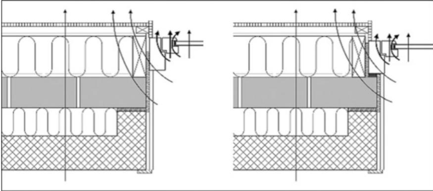
**Fig. 6.8** Example on how a window may be positioned in an externally insulated wall. Cold bridges are reduced by use of a thin insulation layer behind reveal linings and positioning the thermal glazing in plane with the additional insulation. To the right, the window is changed to a slightly larger one allowing more daylight. The arrows in the figure indicate the (reduced) energy loss at cold bridges. (Source: Nørregaard et al. 1984)
