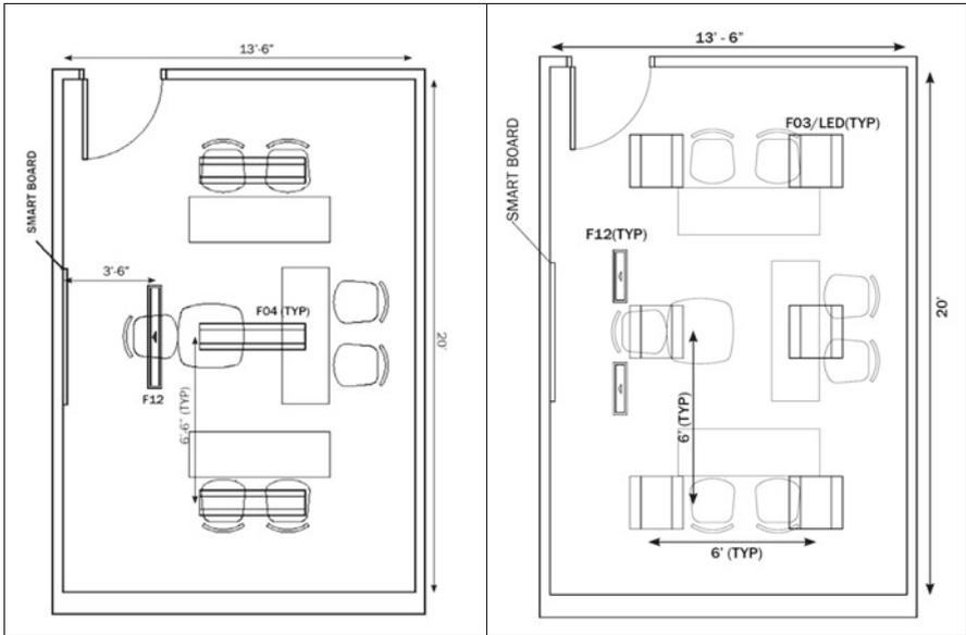
A: SAMPLE SCHEMATIC LIGHTING LAYOUT FOR CEILING HEIGHTS BELOW 9' AFF (NOT TO SCALE)
