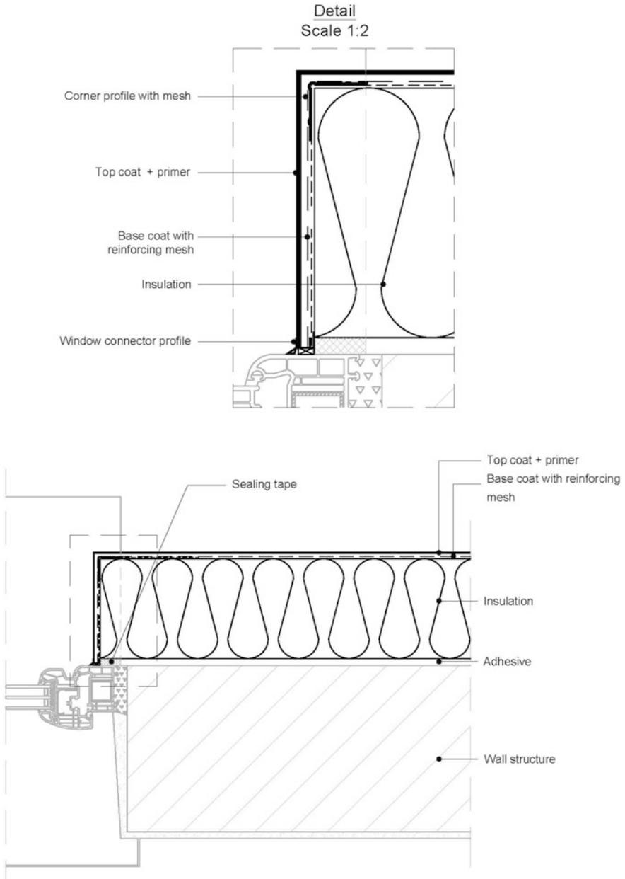
Mounted Equal to the Wall, Cross-Section
