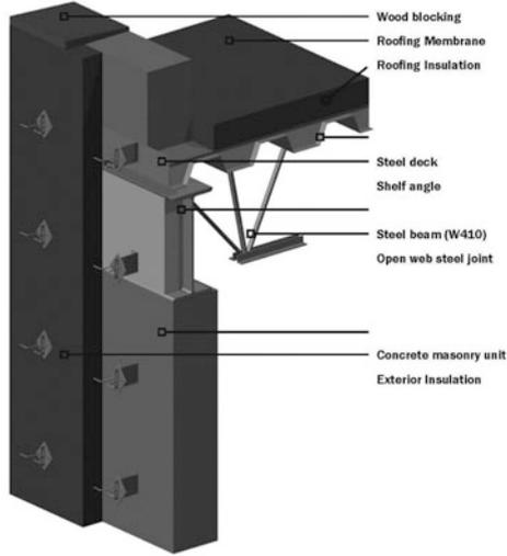
**2b Modeling Values for Parapet (Steel Roof and Joists)**
