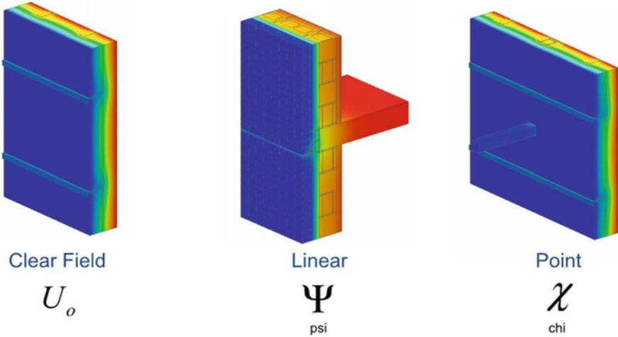
Fig. 8.11 Types of transmittances
