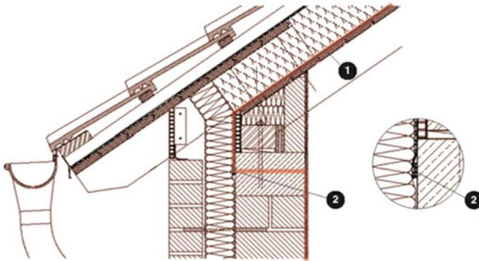
**Fig. F.15** Eaves – above rafter insulation, continuous rafters, lined compartments: (1) air barrier, (2) adhesive
