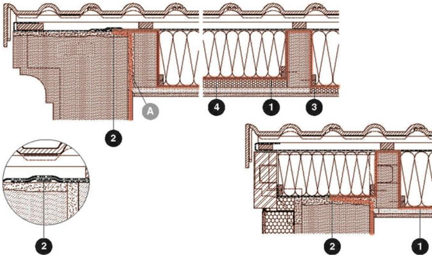
**Fig. F.10** Verge – between-rafter insulation sub-top: (1) air barrier, (2) adhesive, (3) supporting lath, (4) protection layer (optional)
