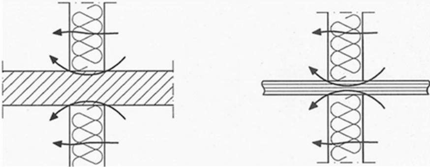
**Fig. 8.5** Constructive thermal bridges. Arrows indicate heat flows. (Source: Olsen and Johannesson 1996)
