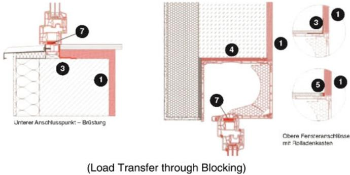
**Fig. F.20** Components of window installed within the wall: (1) interior plaster, (2) smooth finish. (as needed) alternatives: (3) foil seals; (4) sealant strips, multifunctional sealant strips; (5) spray sealant, (6) tapes with sealant strips; (7) seal window-bank junction profile for windows
