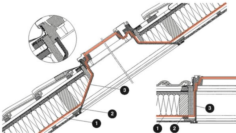
**Fig. F.8** Roof with skylights: (1) air barrier, (2) tape, corner tape, (3) skirt board
