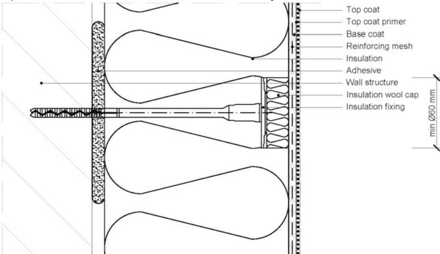
**Bonding of wool boards with random arrangement of fibers. Bead-spot method.**
