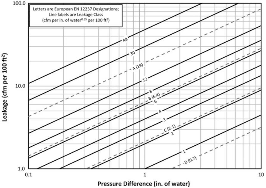
Fig. 12.6 Relationship between ASHRAE leakage classes (solid lines) and European air tightness classes (dashed lines) in IP units
