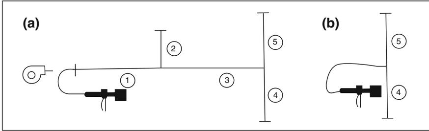
**Fig. 12.9** Ductwork layout and instrumentation, for example: (a) pressurizing entire system; (b) pressurizing sections 4 and 5 combined (note: [ . . . . ] denotes a temporary seal of a duct opening)
