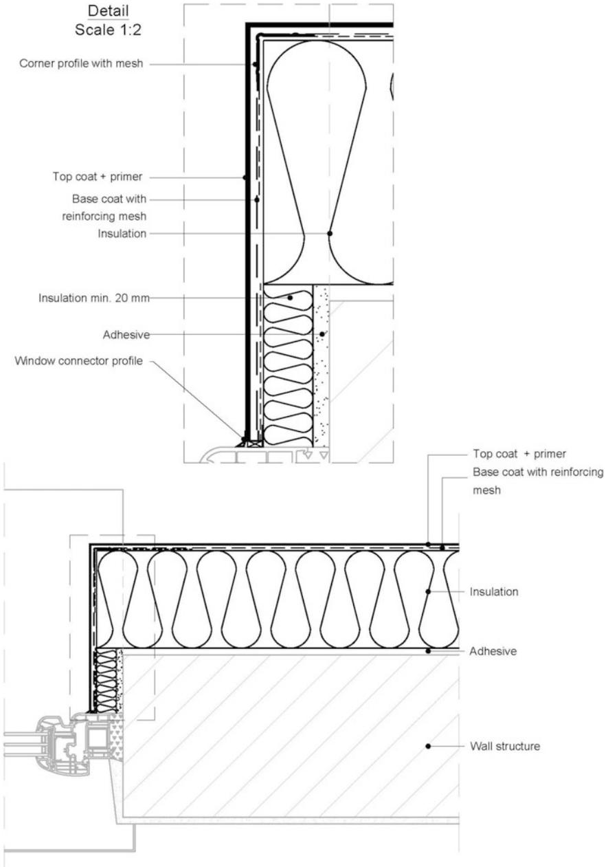
Mounted in the Middle of the Wall, Cross-Section
