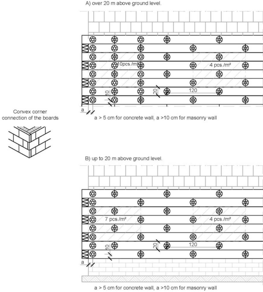
Fig. C.4 Example of mechanical fastening for small mineral wool boards
