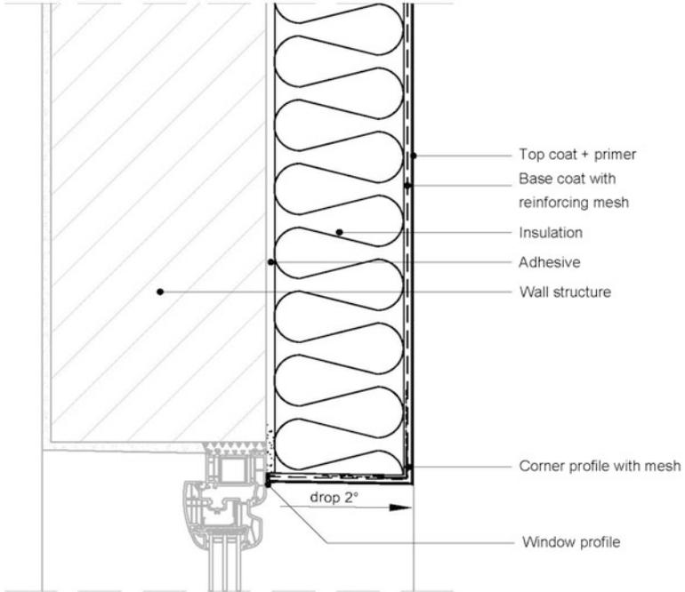
Mounted in the Insulation Layer, Section
