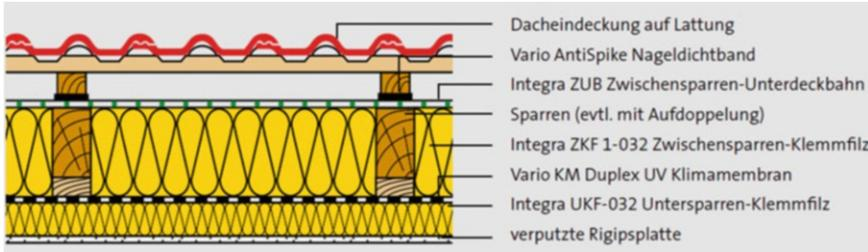
You can fill the existing empty space without losing space inside the building or extend the high of the roof construction to the outside. To minimize thermal bridges from the rafters, a thin additional layer of mineral wool is usually installed between the substructures of the internal finish. Air tightness is a very important parameter for durable function of the roof construction. It is recommended to use air tightness systems with complementary components.
