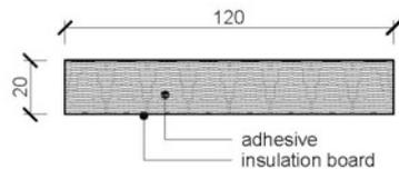
**Fig. C.6** Example adhesive and combined adhesive and mechanical fastening of mineral wool
