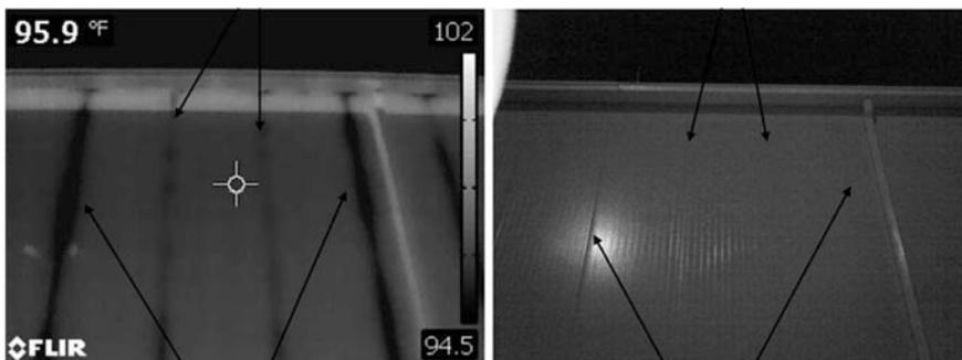
**Fig. H4.2** Loss of thermal barrier continuity due to thermal bridging through metal edges of insulated metal panel joints and air leakage under induced pressure differential through insulated metal panel joints. Note curved/puddle shape anomalies. Source: TMI Air Barrier Testing
