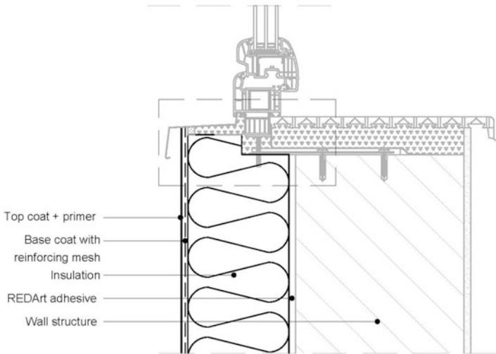
Mounted in the Middle of the Wall, Section
