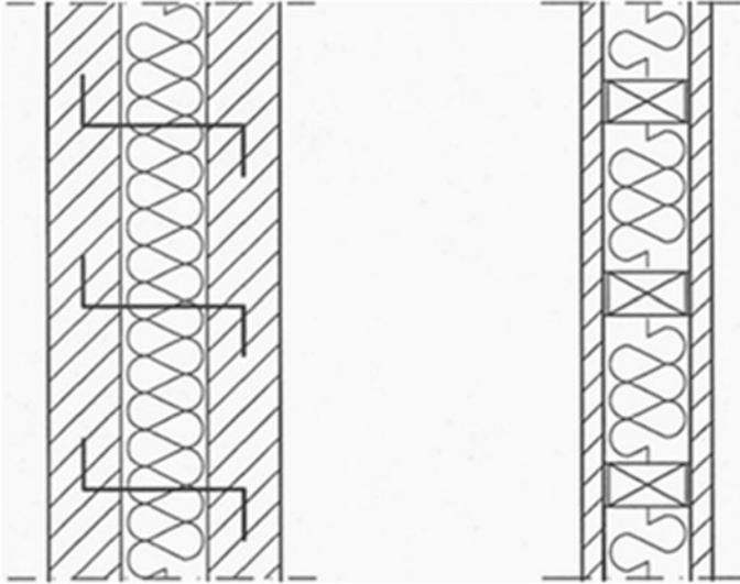
Fig. 8.6 Typical systematic thermal bridges. (Source: Olsen and Johannesson 1996)
