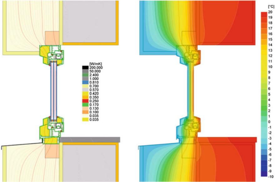
**Fig. 6.9** Example of window installation within exterior finish insulation system (EFIS) (reproduced with permission from PHI)
