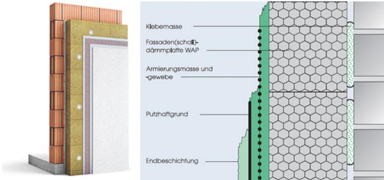
**Picture 1a and 1b** Principle of ETICS construction
