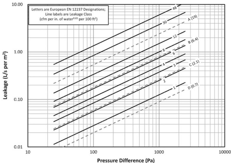
**Fig. 12.5** Relationship between European air tightness classes (dashed lines) and ASHRAE leakage classes (solid lines) in SI units
