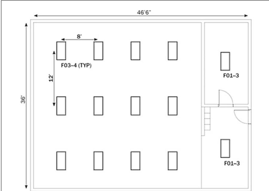
SAMPLE SCHEMATIC LIGHTING LAYOUT (NOT TO SCALE)
