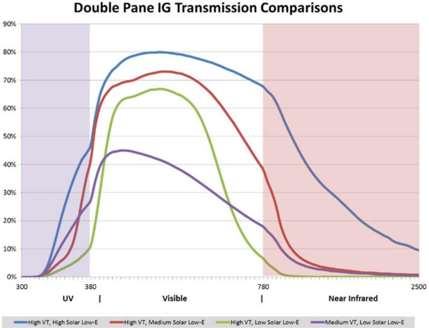
Fig. 7.3 Optical property variations in typical low-e glazing systems
