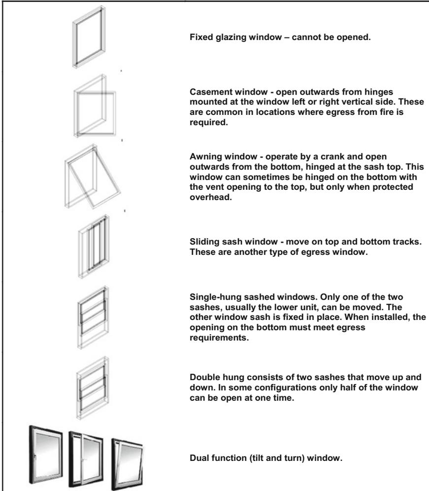
**Fig. 7.2** Different types of unitized windows commonly used in both residential and commercial applications
