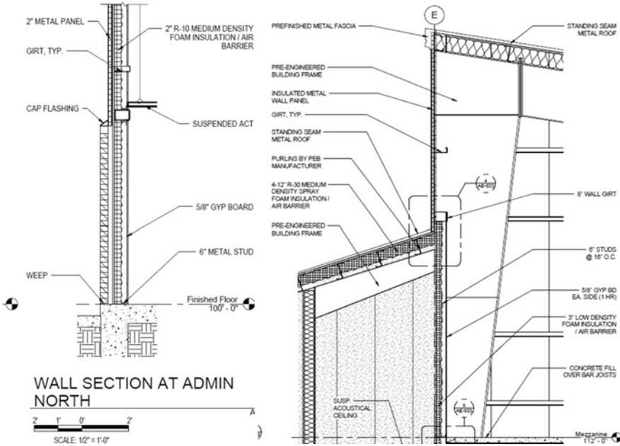
**Fig. F.33** Pre-engineered metal wall systems
