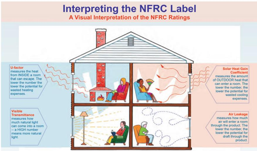
Fig. 7.4 Primary window energy performance elements at work
