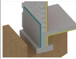
A chase is cut in the mortar joint allowing for the flashing to be added later
