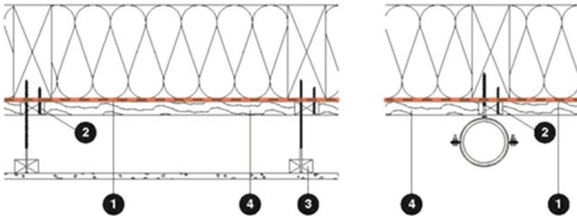
**Fig. F.13** Suspension: (1) air barrier, (2) laths, (3) ceiling suspension, (4) loadbearing lath
