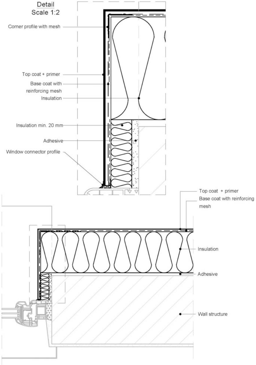
Mounted Equal to the Wall, Section
