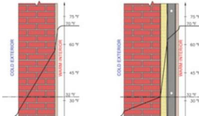
Adding interior air barrier and insulation results in a wall that is colder in winter. Condensation within the brick wall must be controlled so that freeze-thaw cycles do not harm the softer brick that is in the middle of the wall
