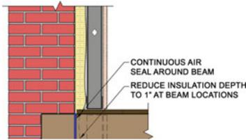
Structural members penetrating the wall are vulnerable to added wetting. Reduce insulation thickness around existing structural members and seal around the member
