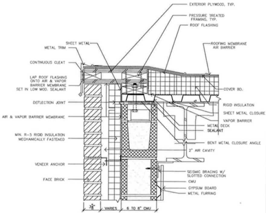
**Fig. F.4** Details of external air barrier design of brick veneer wall, cavity, rigid insulation, air and vapor barrier, concrete block backup, gypsum board: (a) roof edge; (b) parapet; (c) floor slab; (d) wall detail; (e) window head; (f) window jamb; (g) window sill; (h) foundation
