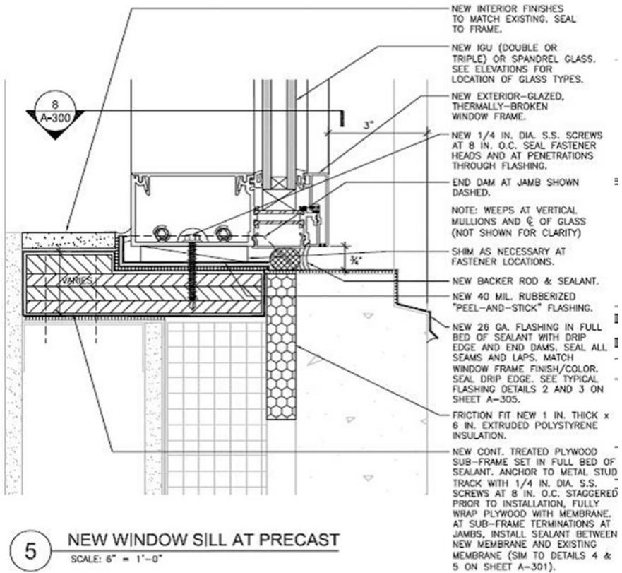
Fig. E.8 Illustration of window sill installation
