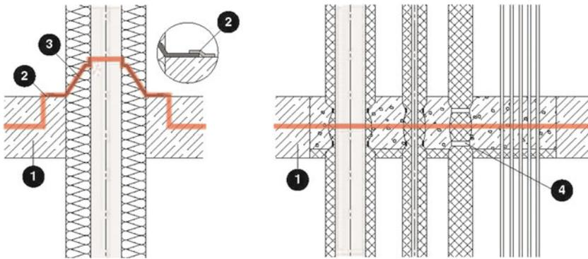
Fig. F.27 Pipe penetration: (1) ceiling, (2) tape, (3) sleeve, molded part, (4) cable tie
