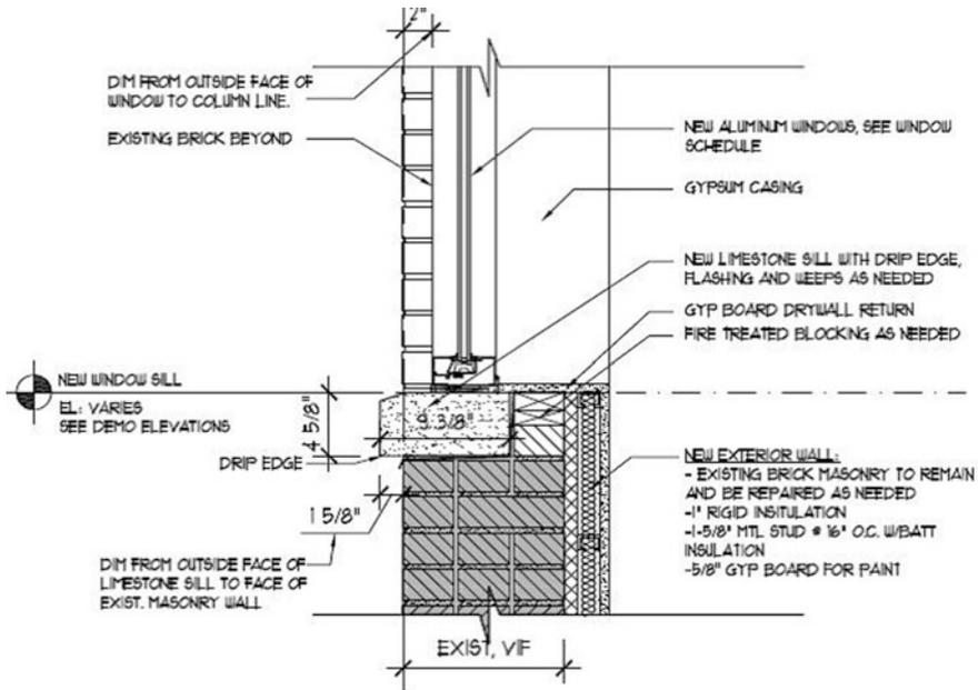
Fig. E.4 Example of thermal bridge in wall construction
