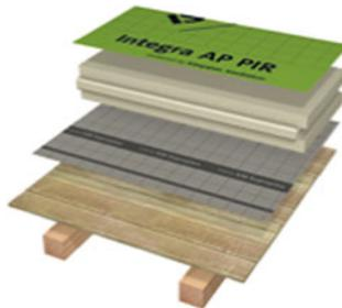
In this option the insulation layer is installed above the rafters, without thermal bridges. The rafters are visible from inside. For static and optical reasons, it is recommended to have a wooden construction as a first layer. On a first rain protection, the insulation boards have to be fixed by screws in the rafters beyond. Then the substructure and the roof covering follow.
