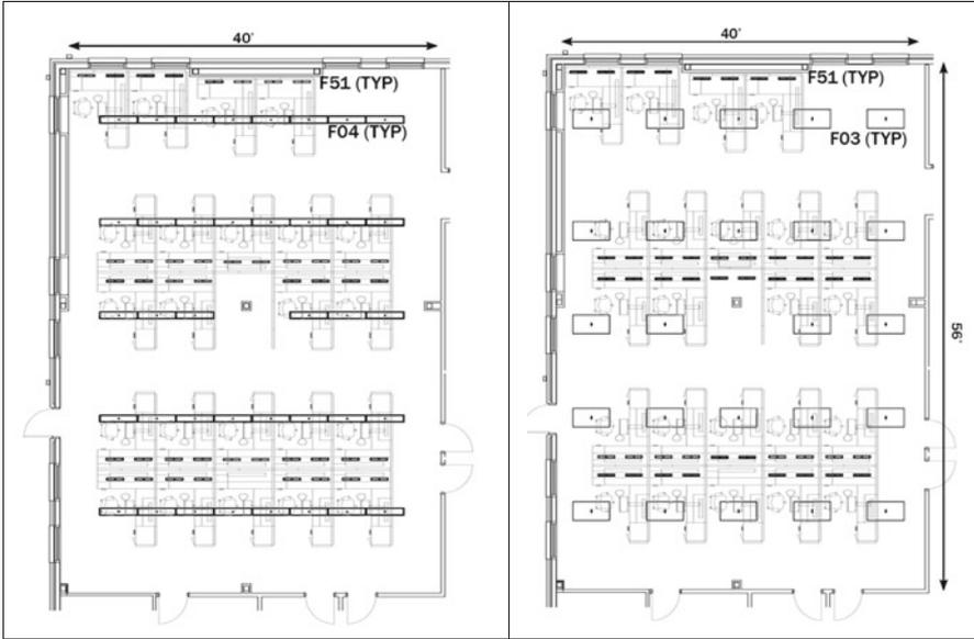
A: SAMPLE SCHEMATIC LIGHTING LAYOUT FOR CEILING HEIGHTS AT OR BELOW 9 FT, 0 IN. (NOT TO SCALE)
