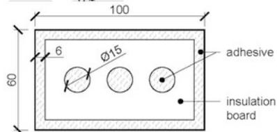
**Fig. C.5** Example combined adhesive and mechanical fastening of mineral wool boards with random arrangement of fibers
