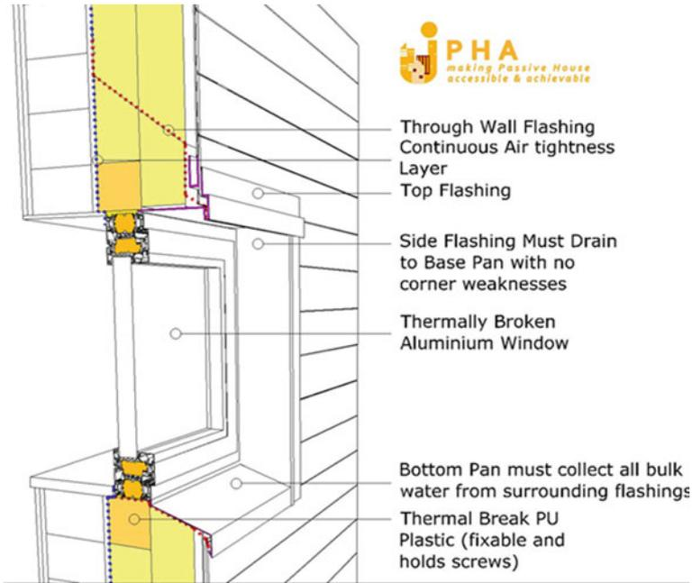
**Fig. E.9** Passive House detail of window installation (provided by the Passive House Academy)
