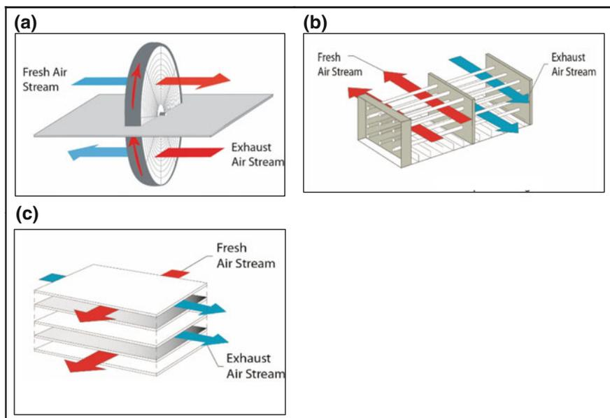
**Fig. 12.2** Typical heat recovery components: (a) rotary air-to-air energy exchanger, (b) heat pipe heat exchanger, and (c) fixed plate cross-flow heat exchanger
