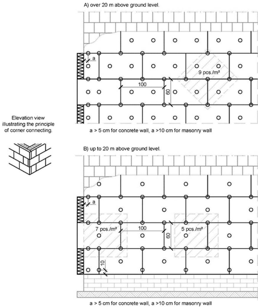
Fig. C.3 Example of mechanical fastening patten for large mineral wool boards
