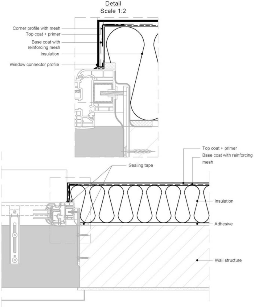
Mounted in the Insulation Layer, Insulation of the Windowsill, Cross-Section
