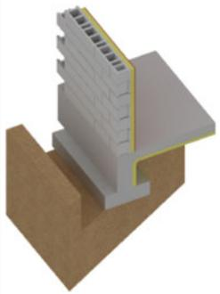
If the slab edge cannot be retrofit, then insulating the external perimeter can help to contain heat within the ground and raise internal surface temperatures
