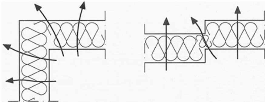
**Fig. 8.3** Geometrical thermal bridges. Arrows indicate heat flows. (Source: Olsen and Johannesson 1996)
