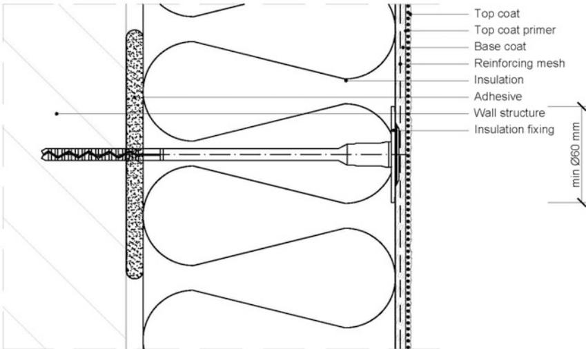
B) Mechanical fixation - countersunk assembly
