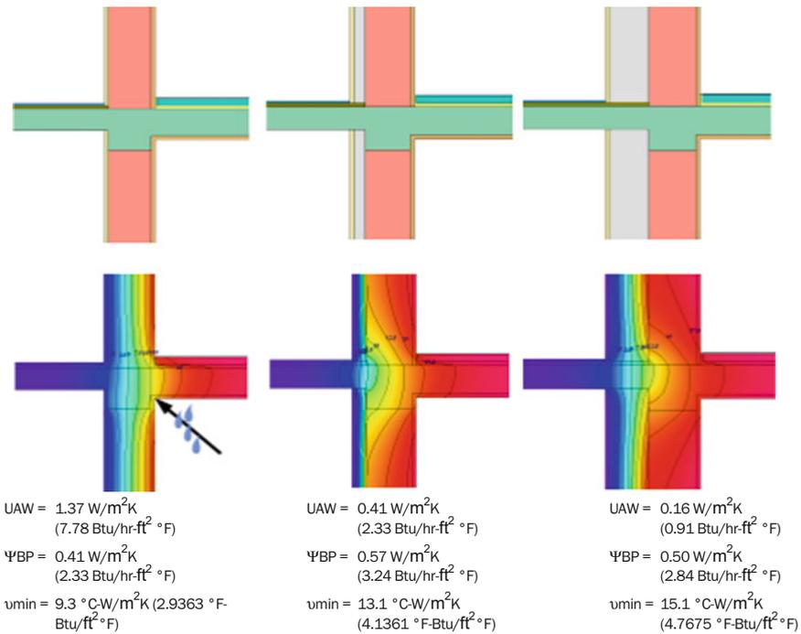
**Fig. 8.13** Example of thermal bridge created by a balcony. Left: prerenovation situation; middle: conventional insulation thickness; right: well-insulated wall with  $\geq 20$  cm of insulation
