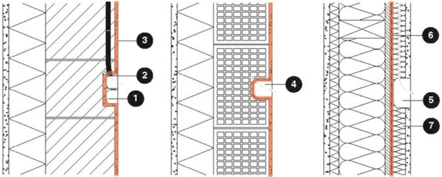
**Fig. F.26** Electrical conduits: (1) electrical installation box, (2) sealing plugs, (3) plaster, (4) airtight electrical installation box, (5) installation housing, (6) air barrier, (7) installation level
