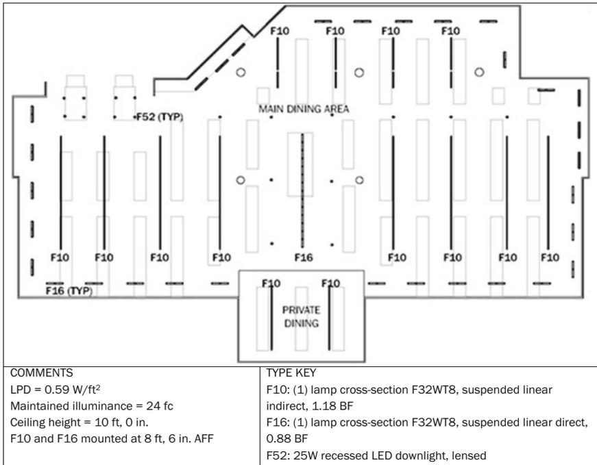
**Fig. G.1** Sample schematic lighting layout (not to scale)
