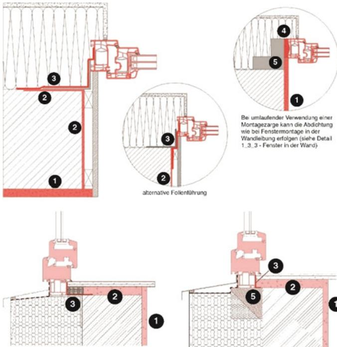
**Fig. F.21** Window installed within the wall: (1) interior plaster; (2) smooth finish (if needed); (3) foil joint seals; (4) deviation from the standard installation, e.g., multifunction adhesive strips; (5) subframe
