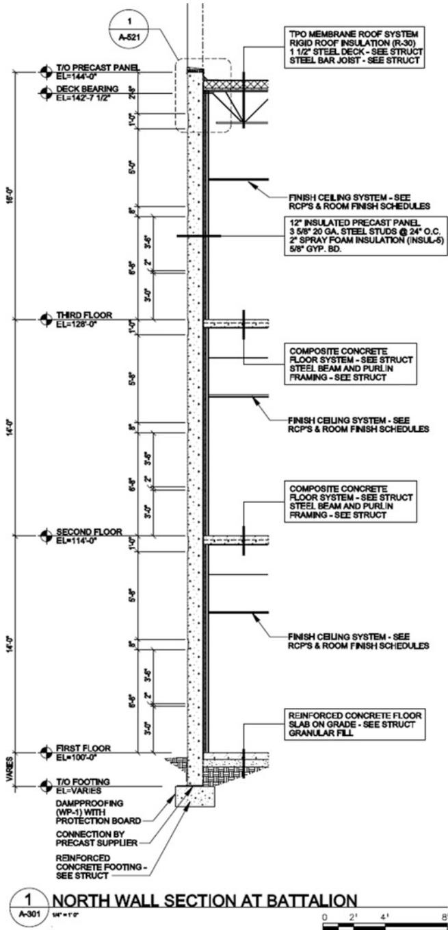
Fig. F.30 First of two sections for a precast concrete wall assembly
