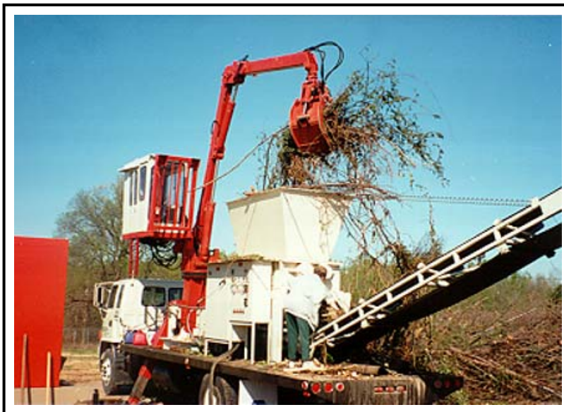
Figure A-17. Shearing shredder.
