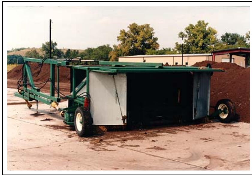
Figure A-19. Towed windrow turner.
