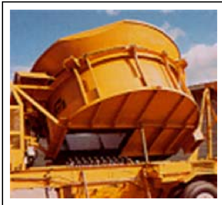
Figure A-11. Tilted tub grinder.
