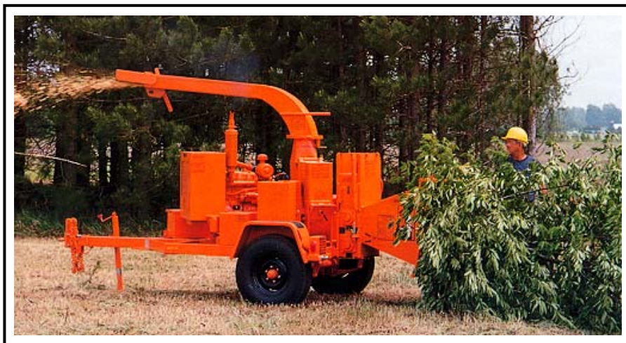
Figure A-16. Chipper-shredder.
