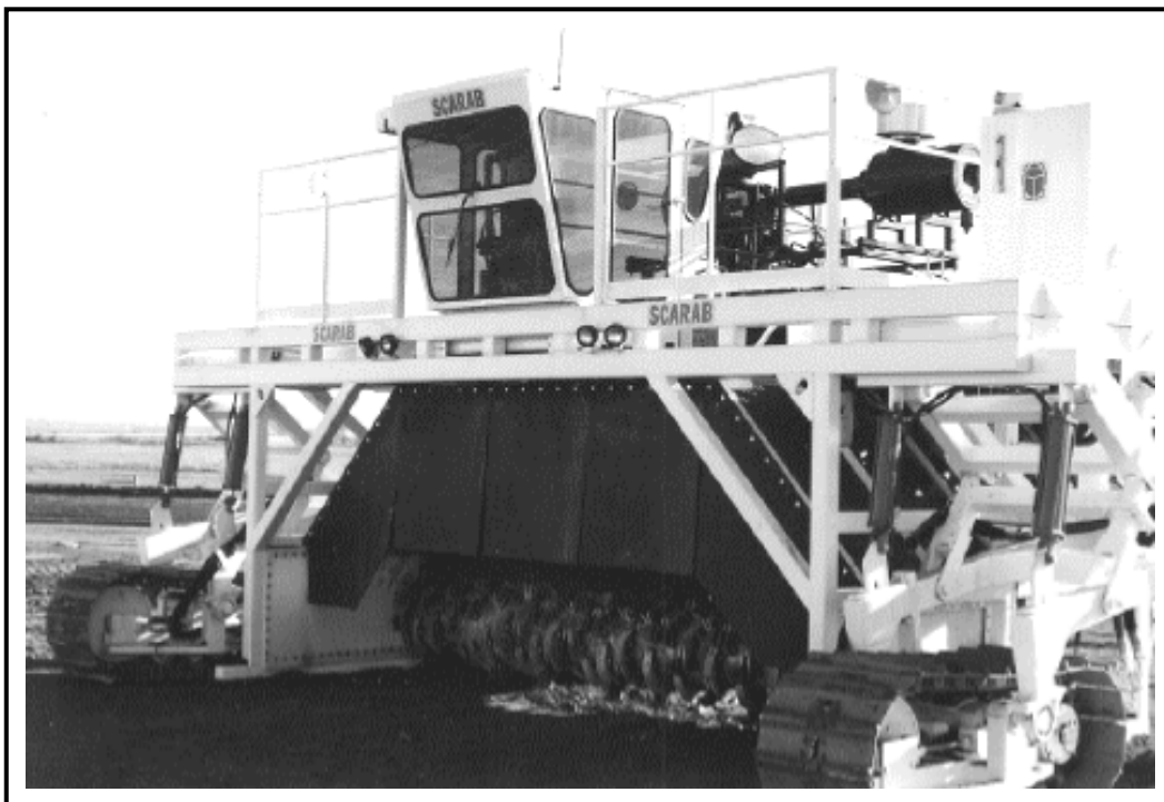
Figure A-21. Straddle type windrow turner.
