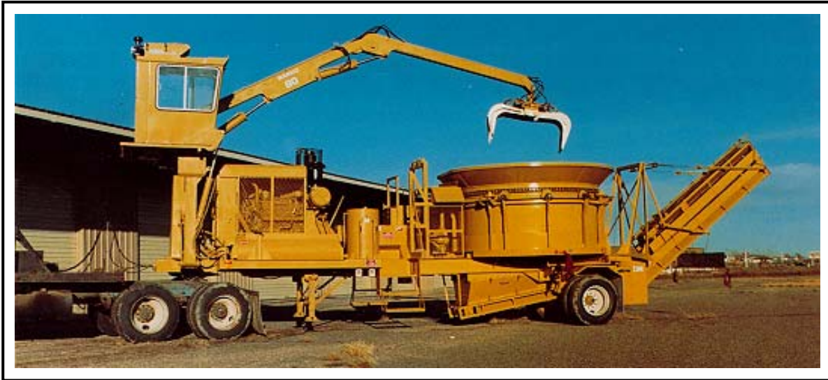
Figure A-10. Tub grinder.
