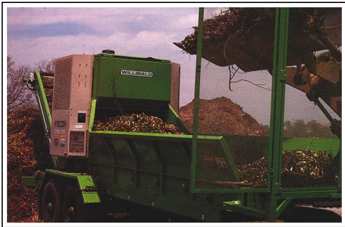
Figure A-14. Grinder with in-feed conveyer.
