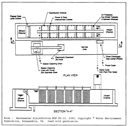
Figure A2. Lamp Modules Relative to Inlet and Outlet Structures; Lamp Modules Are Placed Far Enough Away From Flow Structures to Ensure Uniform Flow at the Entrance to and Exit From the Irradiated Zone.
