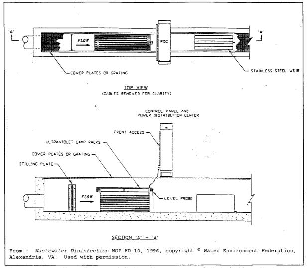
Figure A3. Ultraviolet Disinfection System with Stilling Plate for Flow Conditioning and Elongated Weir for Level Control.
