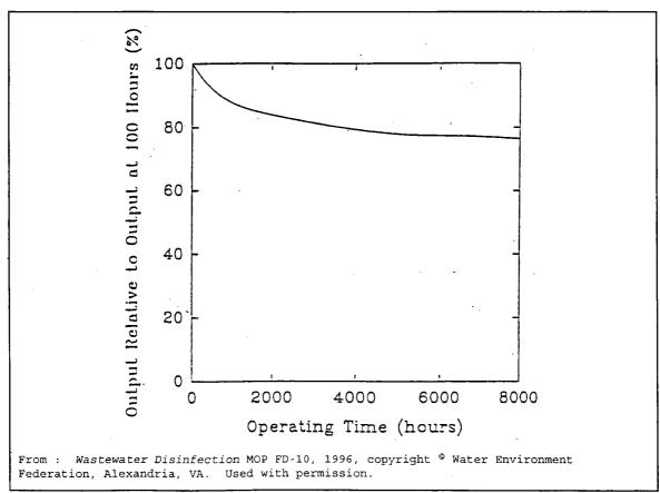
Figure A4. Typical Ultraviolet Lamp Output as a Function of Time.
