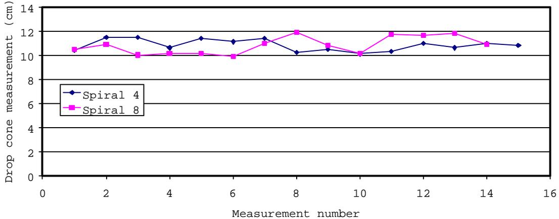
Figure D7. Sand field drop cone measurement.
