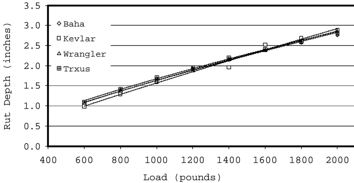
Figure C28. Rut depth at 20 psi.
