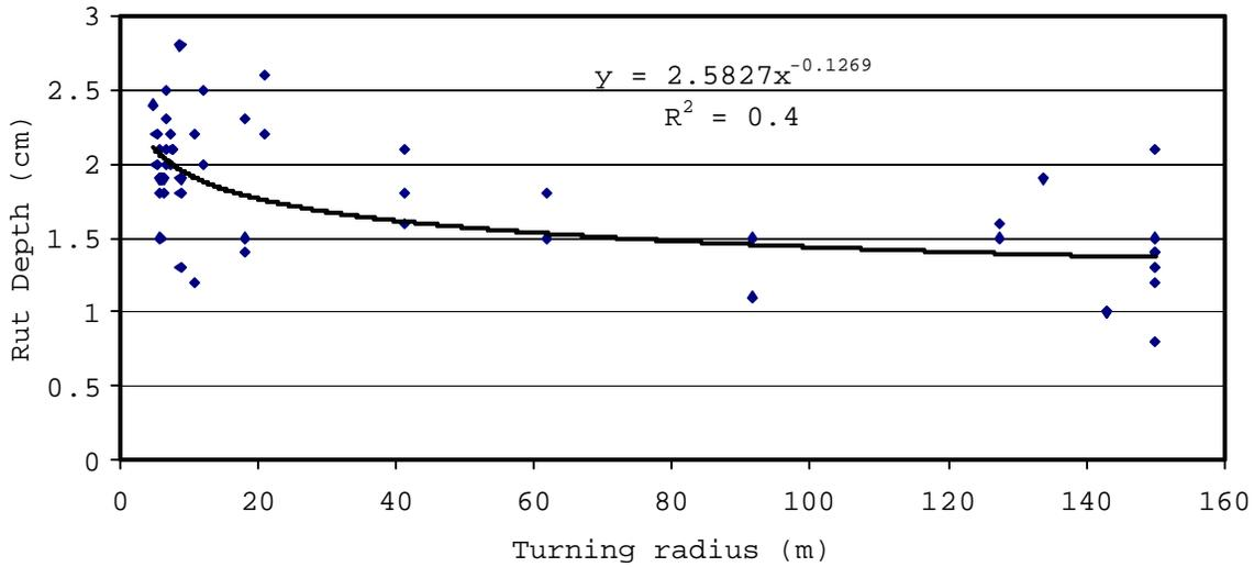
Figure D14. Rut depth of Kevlar tire at low speed.
