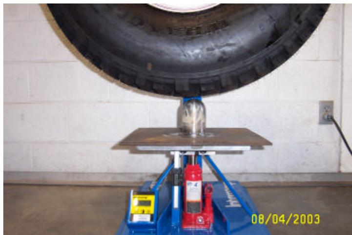
Figure C31. Plunger test.
