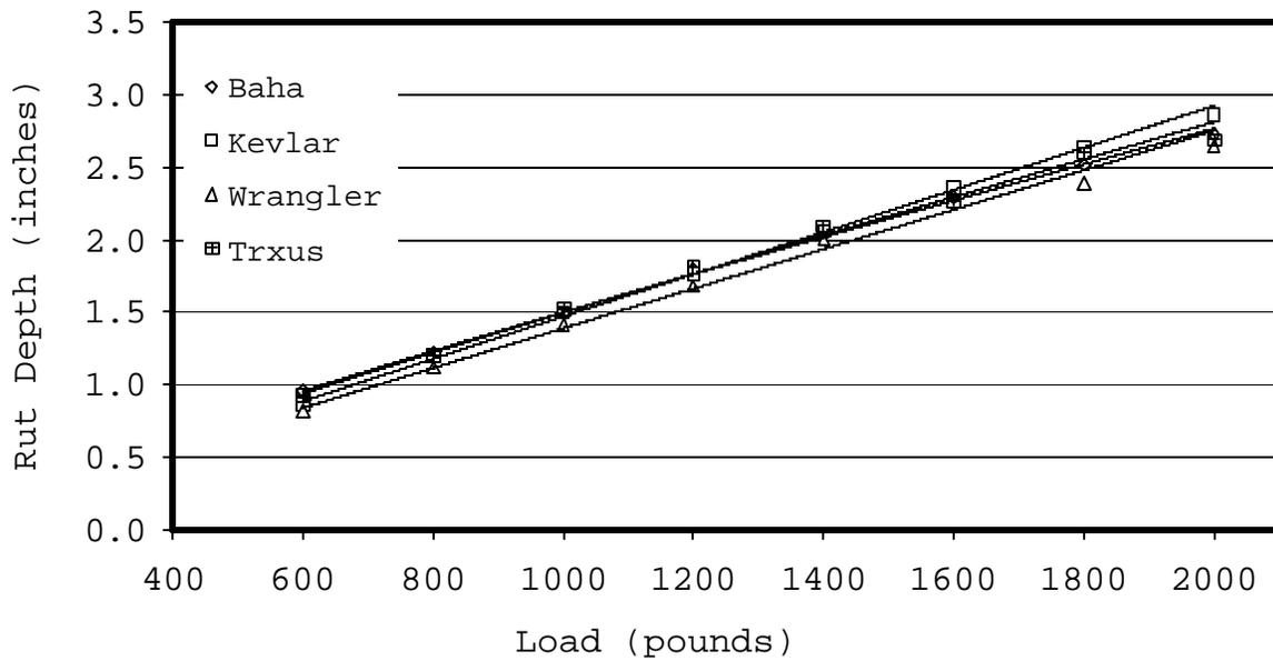
Figure C26. Rut depth at 10 psi.
