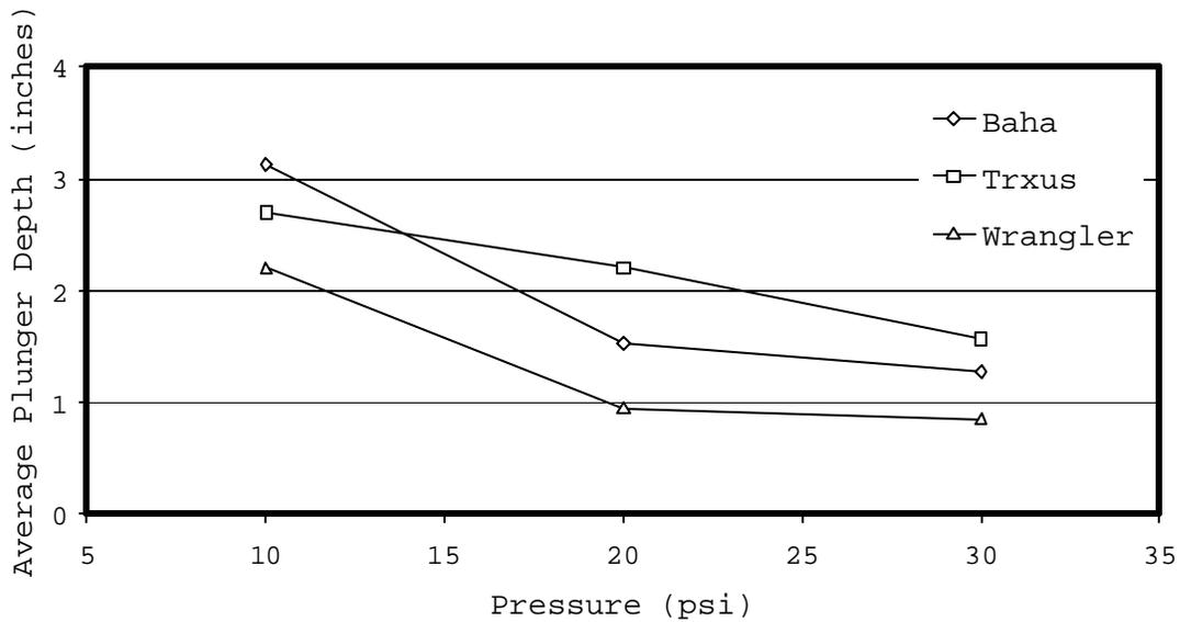
Figure D2. Plunger depth for each tire. **Rutting Field Tests**
