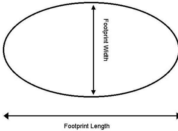
Figure C2. Diagram of measured tire footprint area.
