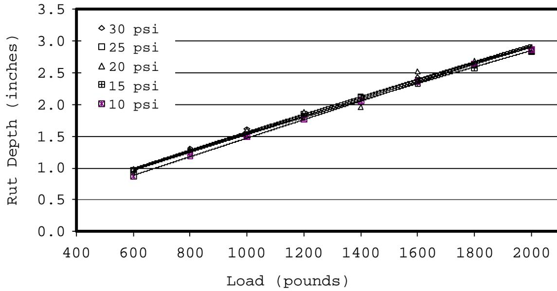
Figure C23. Kevlar tire rut depth.
