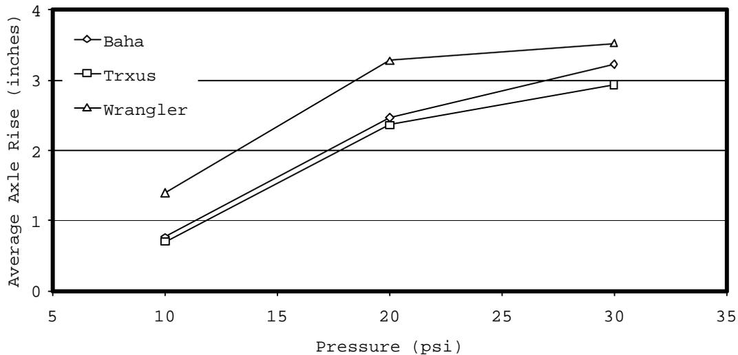
Figure D1. Axle rise for each tire.
