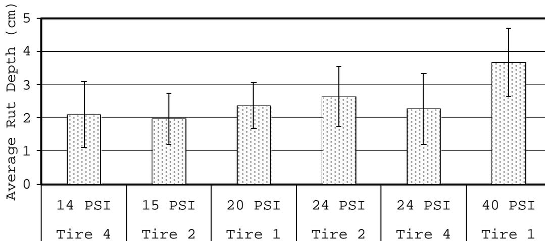
Figure D5. Average rut depth with increasing tire pressure.
