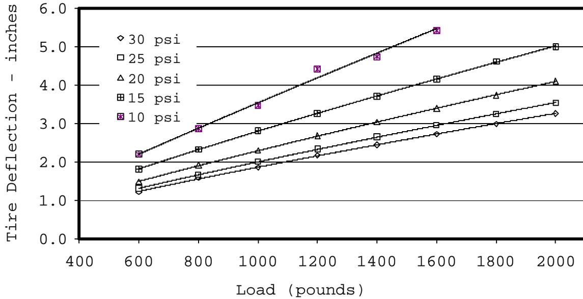
Figure C34. Wrangler tire plunger deflection.
