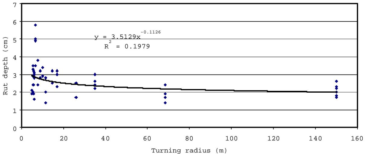
Figure D17. Rut depth of Goodyear at high speed.
