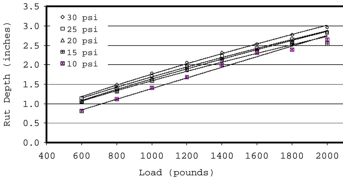
Figure C24. Wrangler tire rut depth.
