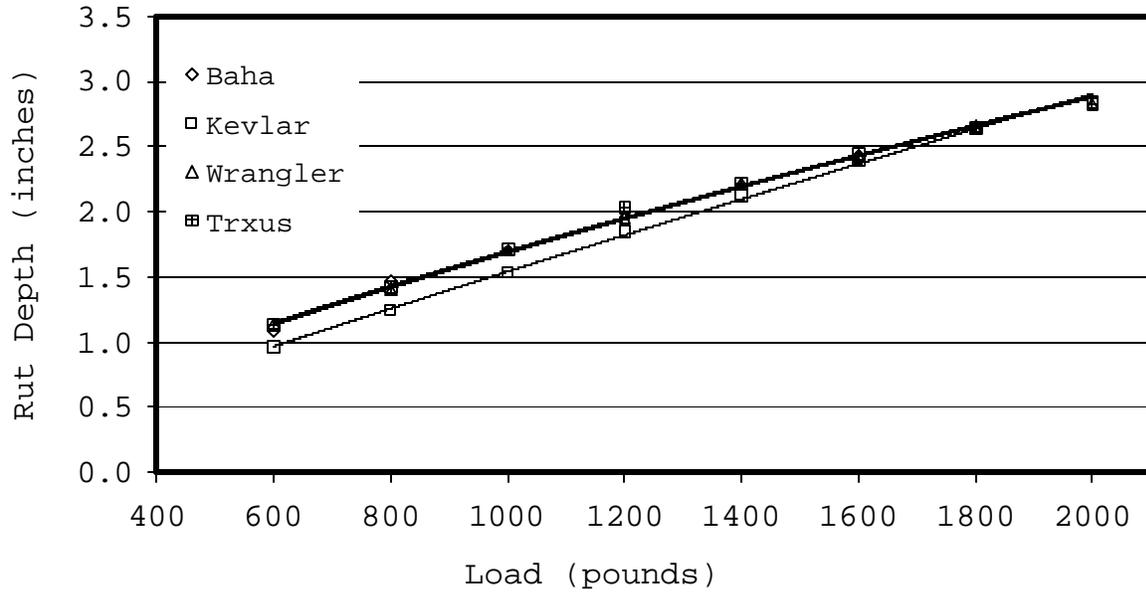
Figure C29. Rut depth at 25 psi.
