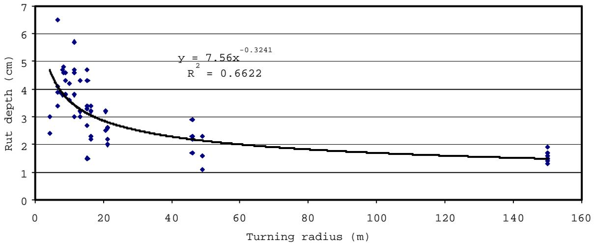
Figure D16. Rut depth of Kevlar tire at high speed.
