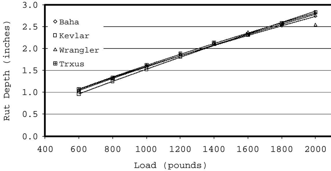
Figure C27. Rut depth at 15 psi.
