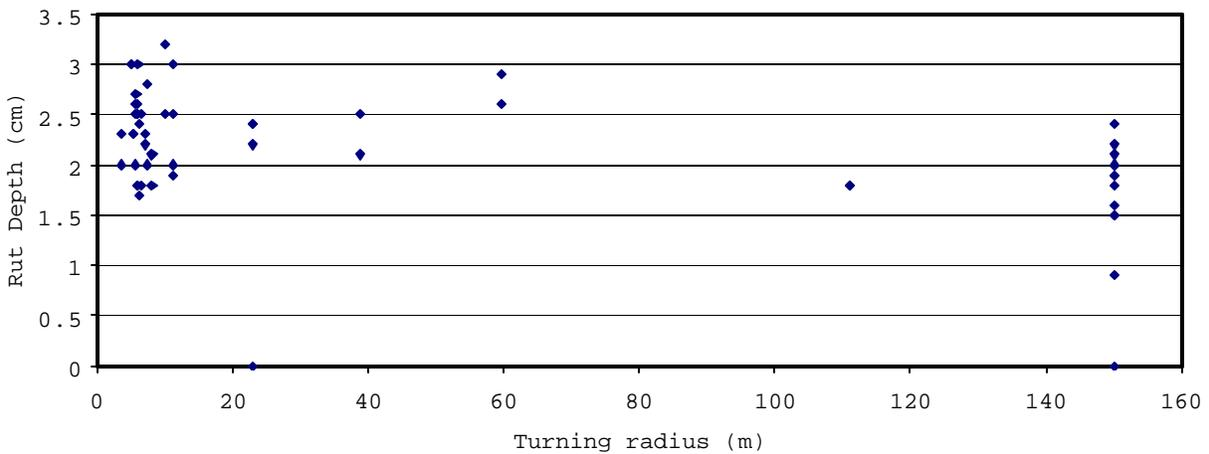
Figure D15. Rut depth of Goodyear tire at low speed.
