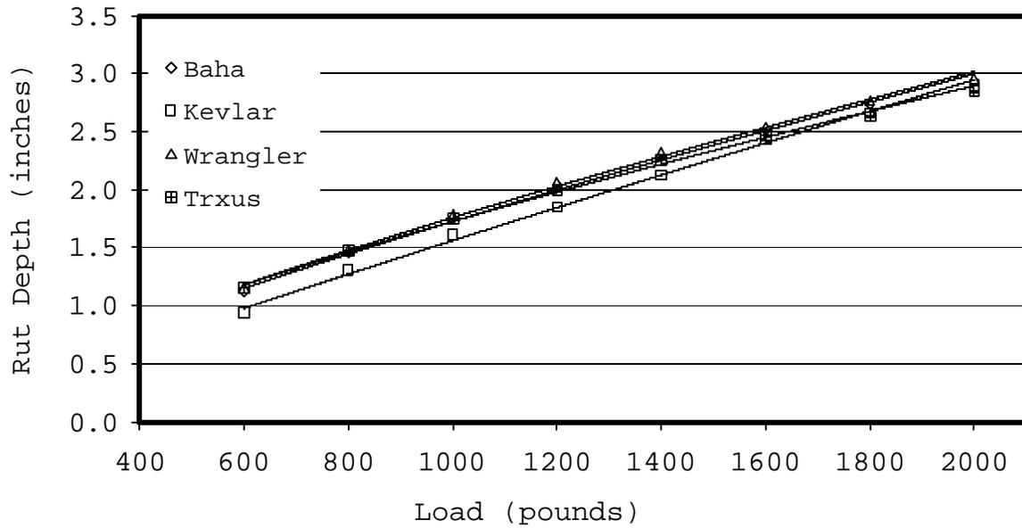
Figure C30. Rut depth at 30 psi.
