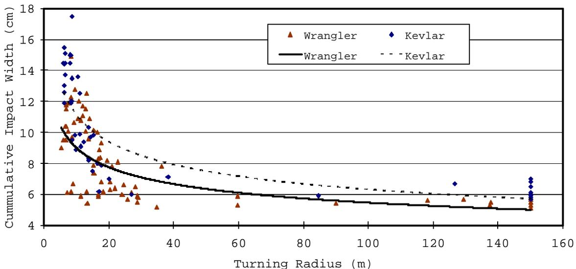
Figure D24. Tire impact comparison.
