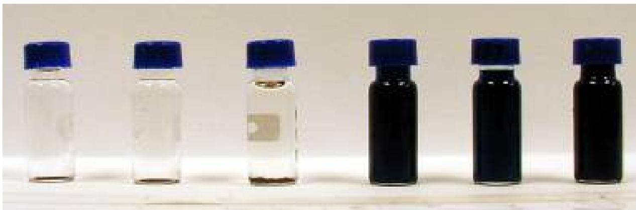
Figure 6: Extracted samples from deposition of seven green signaling grenades. From left to right, the collection media were oxidized ACF, basic ACF, ACF-15, foil, GFF, and ACF-7.
