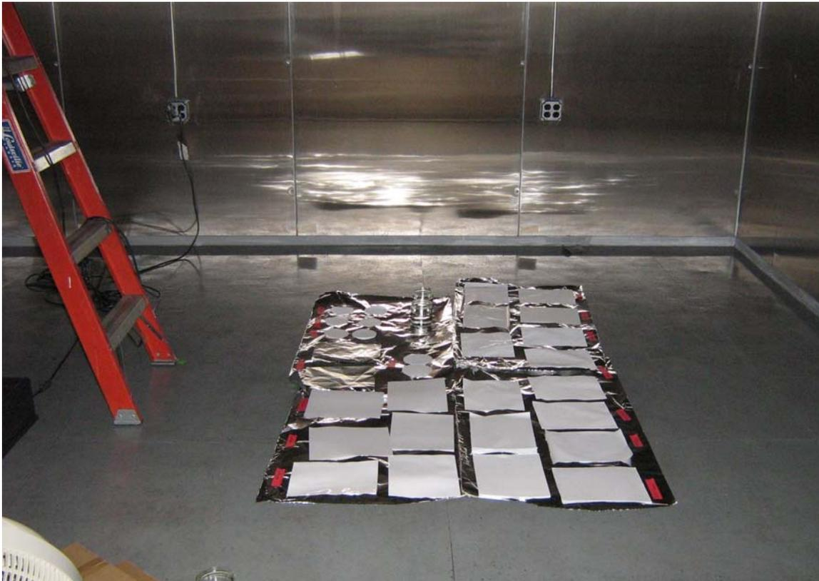
Figure 14: Filters placed on the floor of the chamber for a fogging event.
