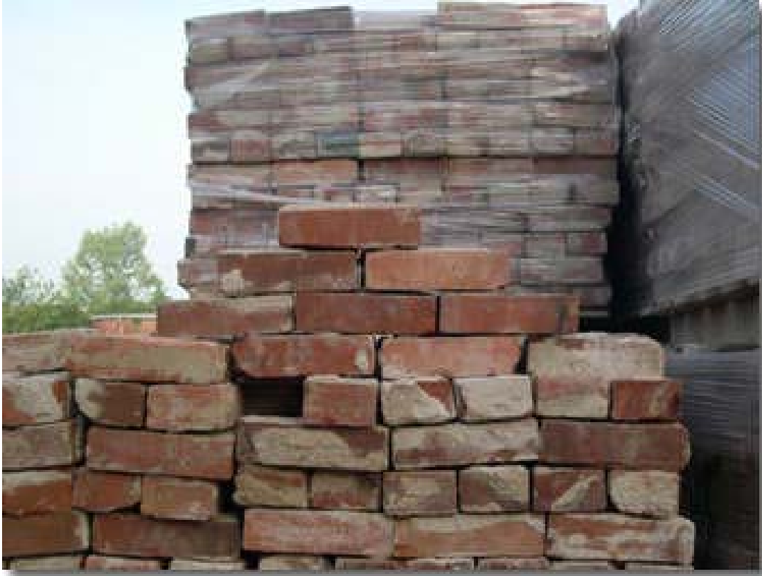
Figure 10. Pallets of salvaged bricks.
