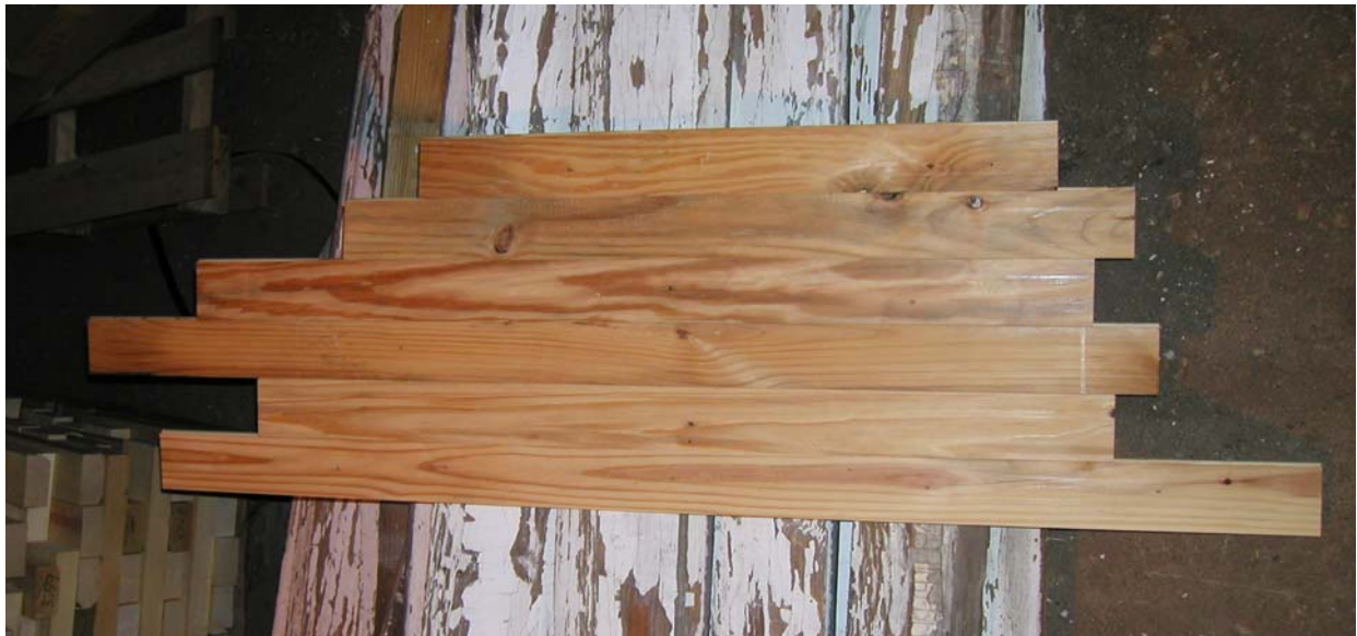
Figure 9. Tongue and groove flooring produced from siding.
