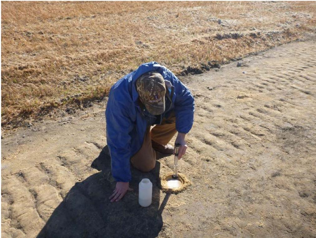
Figure B-6. Bioswale infiltration testing.
