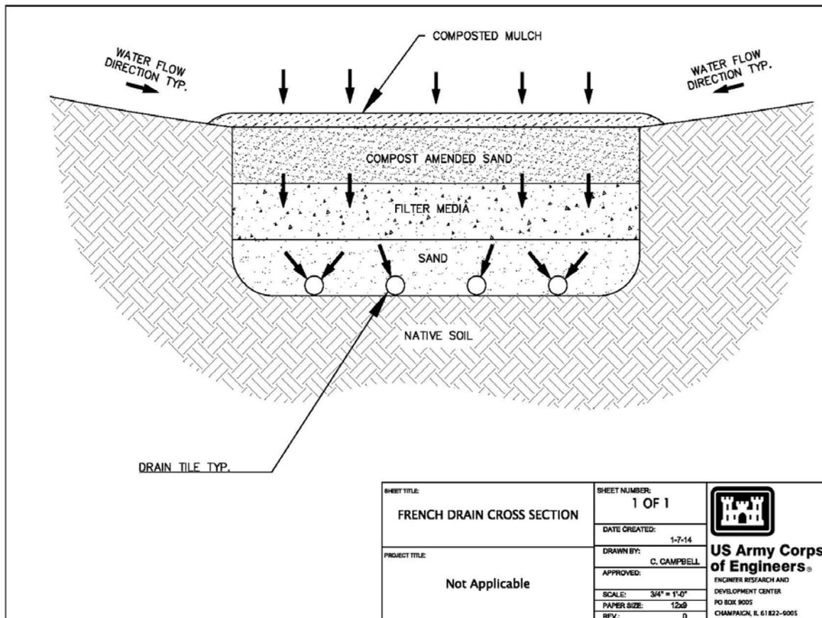
Figure B-5. Cross section of subsurface drainage system.
