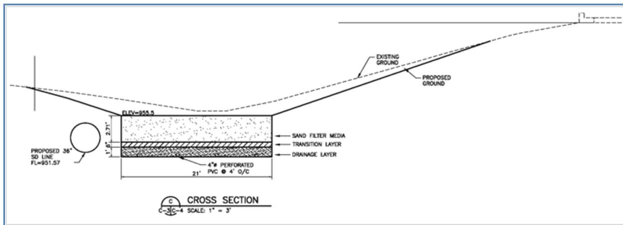
Figure B-2. Cross section of bioswale showing subsurface drainage and filter media layers.
