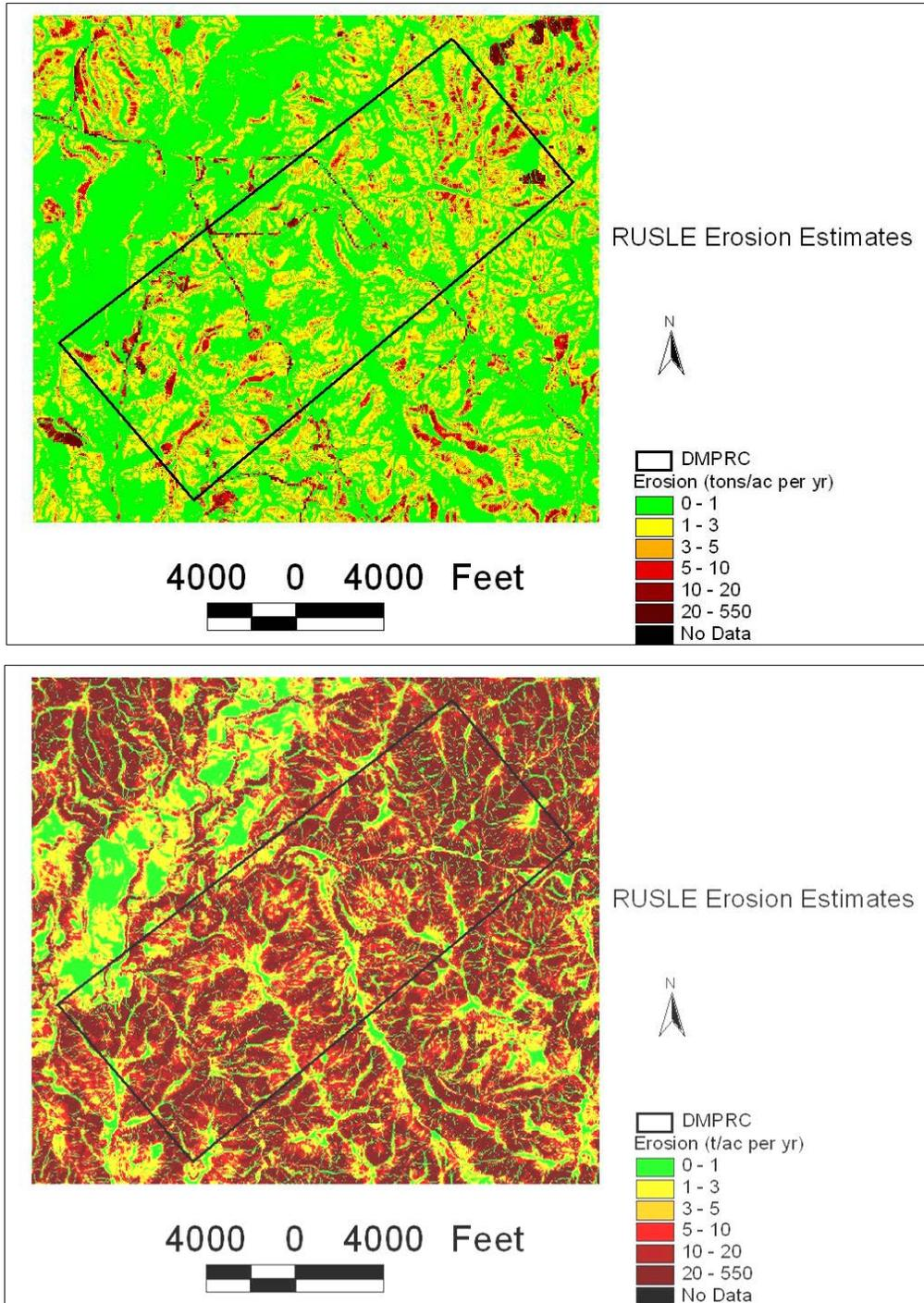
**Figure A-4. DMPRC erosion potential (top) before and after construction (bottom).<sup>1</sup>**
