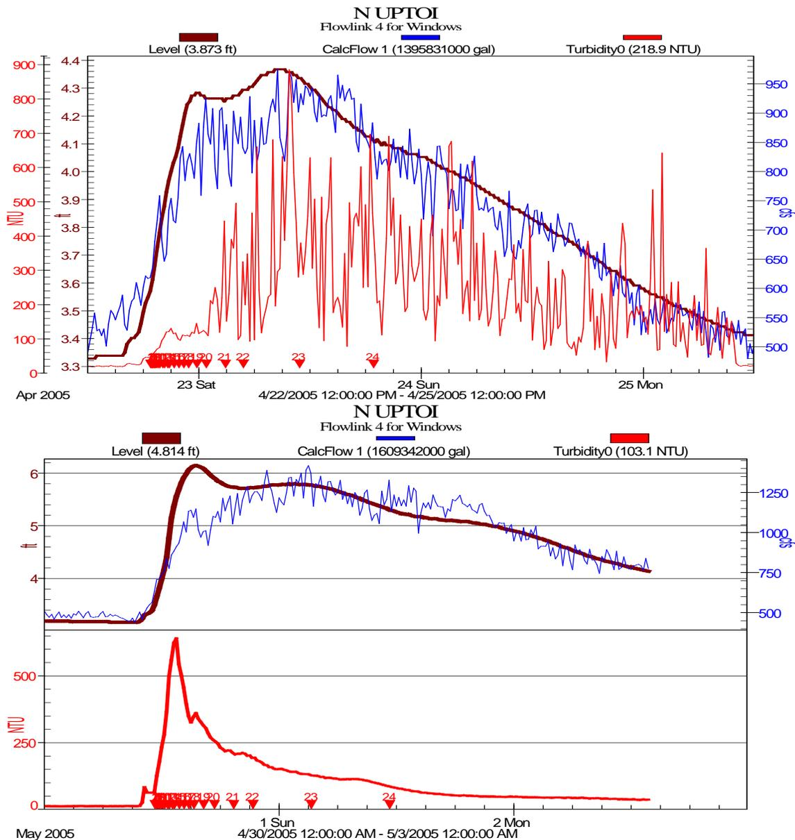
Figure C-7. Typical stream turbidity, stream level, and flow data collected and stored in Isco samplers.
