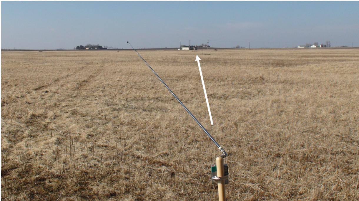
Figure B-1. A static position test is shown with the transmitter positioned at 45 degrees from vertical. The transmitter was ~389 m from the receiving towers seen in the background near the Monticello Road Field Station.
