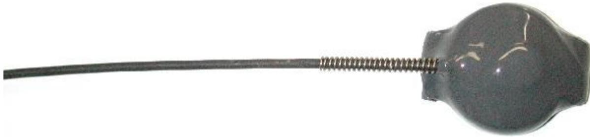
**Figure A-1.** An example of a standard 15-g whip antenna transmitter showing the transmitter and battery enclosed in a protective weatherproof casing (gray part) that is roughly the size of a quarter.
