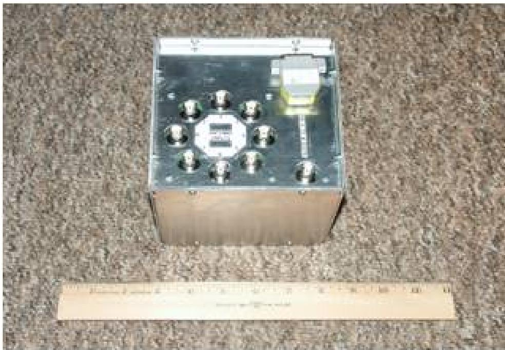
Figure A-3. An example of one of the radio telemetry receivers tested, which is part of the Automated Recording Unit (ARU) system.
