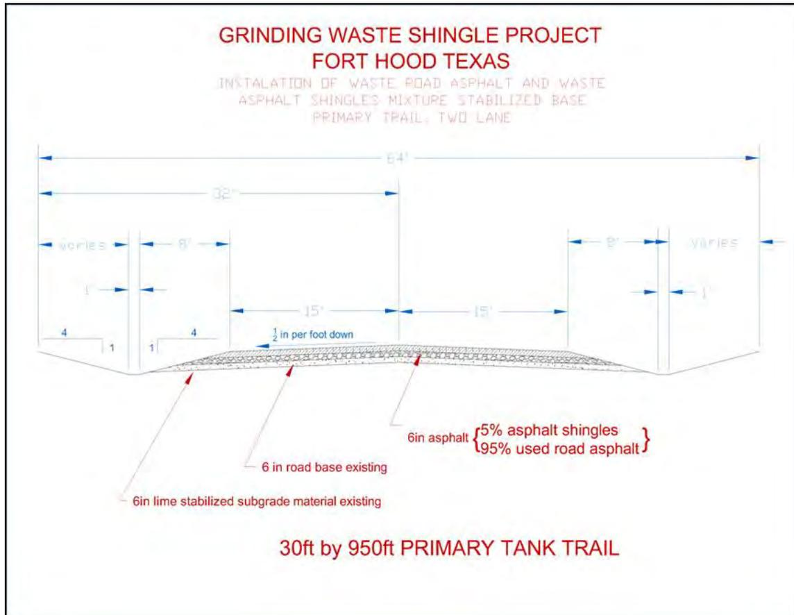
**Figure A-3. Cross-section diagram of a typical primary tank trail.**
