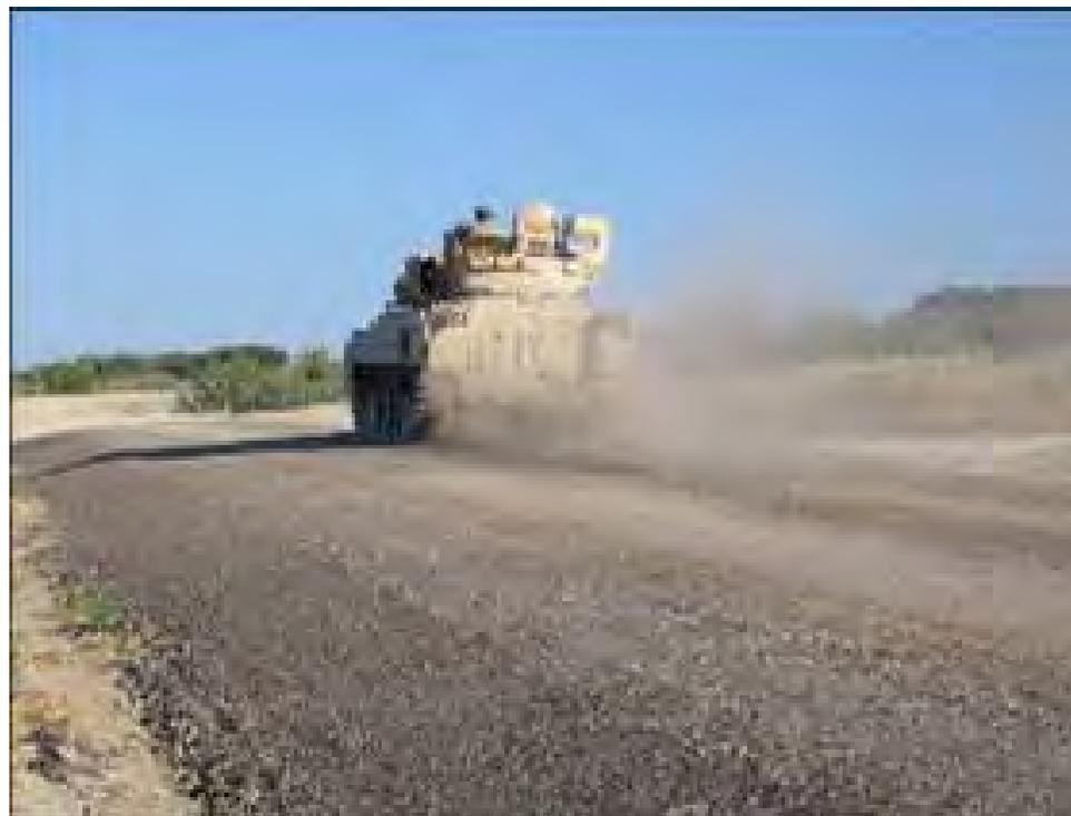
Figure A-9. Bradley tank traveling on asphalt shingle mix.
