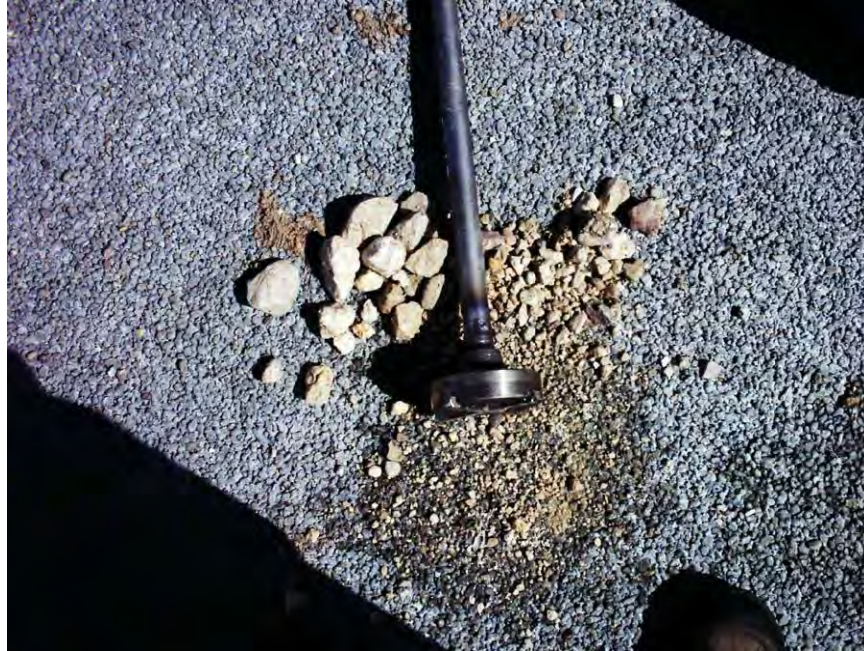
Figure A-7. Poorly washed gravel removed from a sample port.
