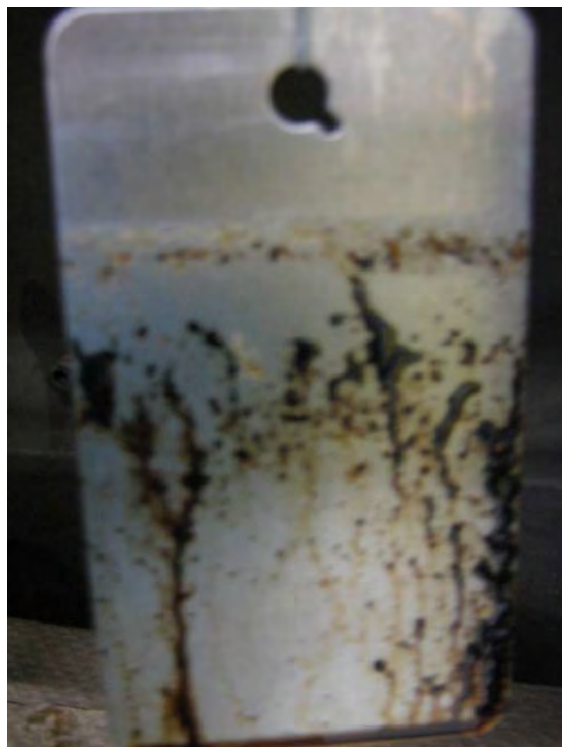
Figure C-14. Asphalt-coated coupon submerged in Simple Green at 80 °C for 90 min.
