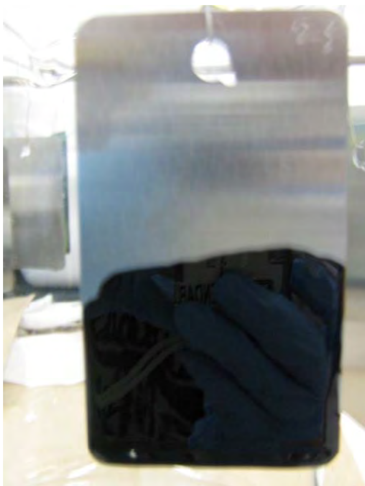
Figure C-8. Asphalt-coated coupon submerged in Simple Green for 30 min at room temperature.
