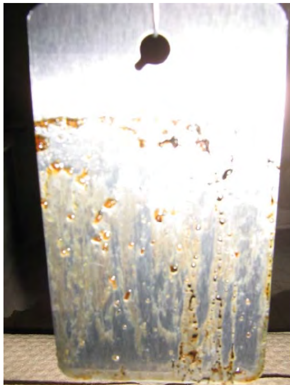
Figure C-13. Asphalt-coated coupon submerged in Simple Green at 80 °C for 60 min.
