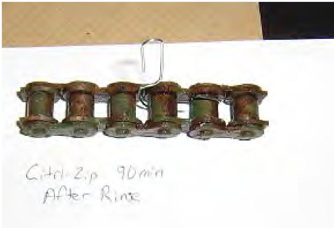
Figure C-16. Chain after immersion in Citri-Zip for 90 min and after rinse.
