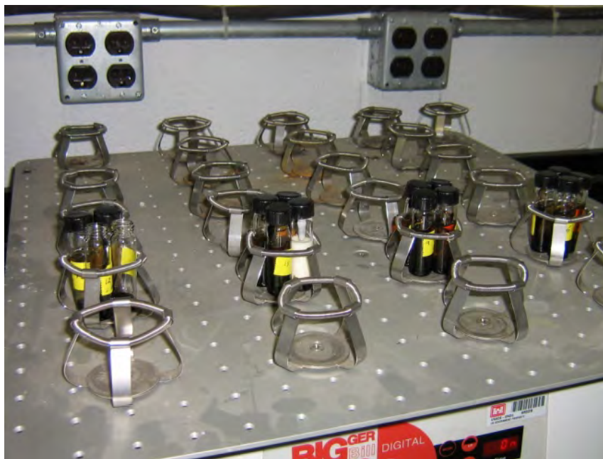
Figure C-1. Vials with tar and solvent on rotating shaker.
