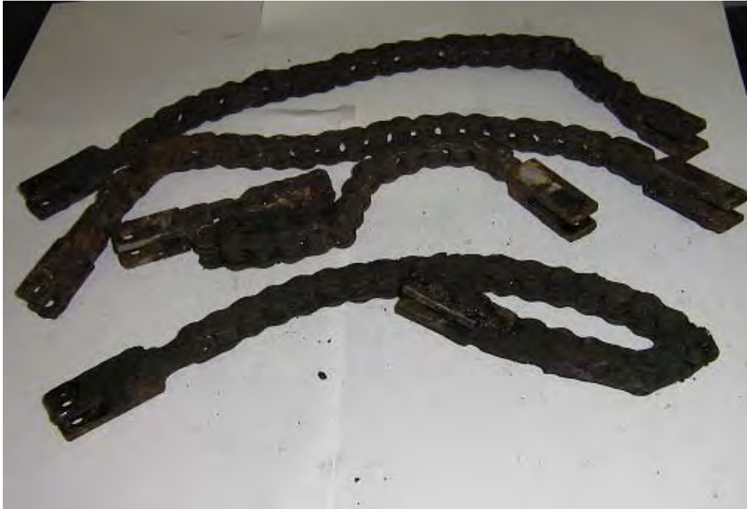
Figure C-15. Dirty chains before immersion in Citri-zip solvent.
