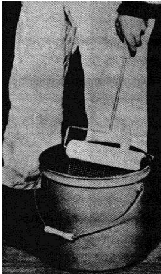
FIGURE 4-33 Roller and Wire Screen Attachment to Can
