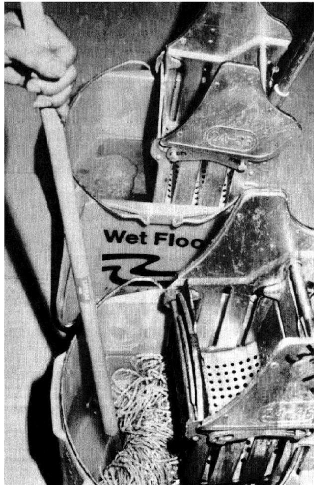
Figure E-25. Wet mop, mop bucket and down pressure type wringer.
