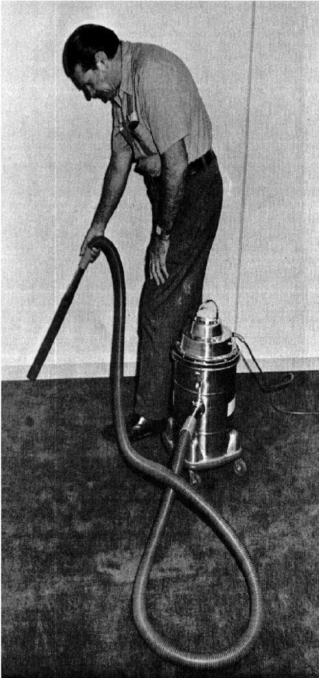
Figure E-7. Wet/dry tank vacuum.
