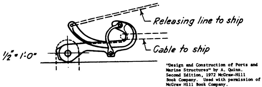
Figure 10-7. Typical releasing hook.
