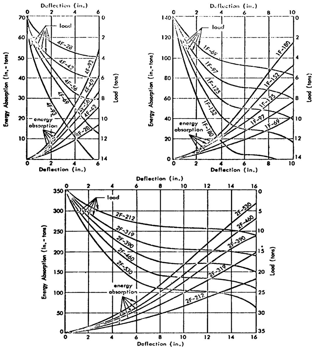
Note: The part number IF-69 is defined as a Lord rubber fender having an energy-absorption capacity of 6,900 foot-pounds at full deflection of 10 inches (for IF series). Full deflection for other series are: 2F series - 16 inches; 4F series - 6 inches.
