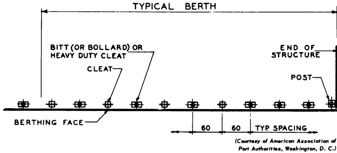
Figure 10-8. Typical layout of mooring devices.
