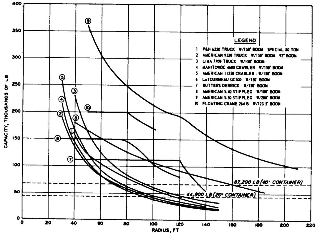
Figure 12-6. Crane capacity.
