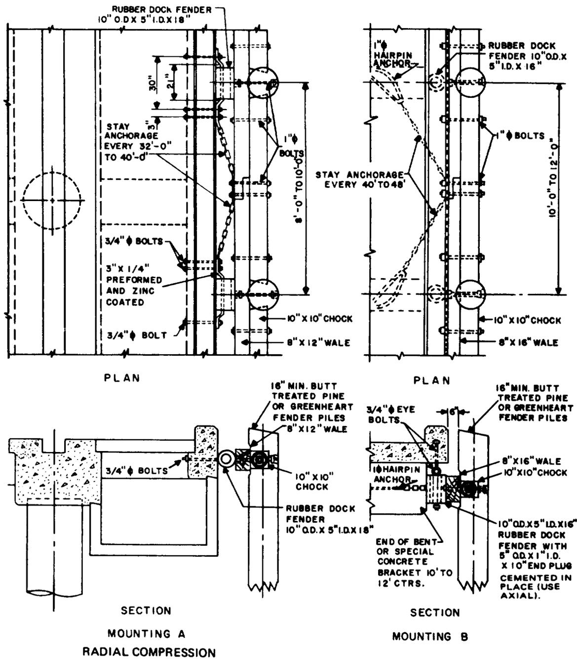
Figure 9-6. Resilient Fender System (rubber-in-compression).
