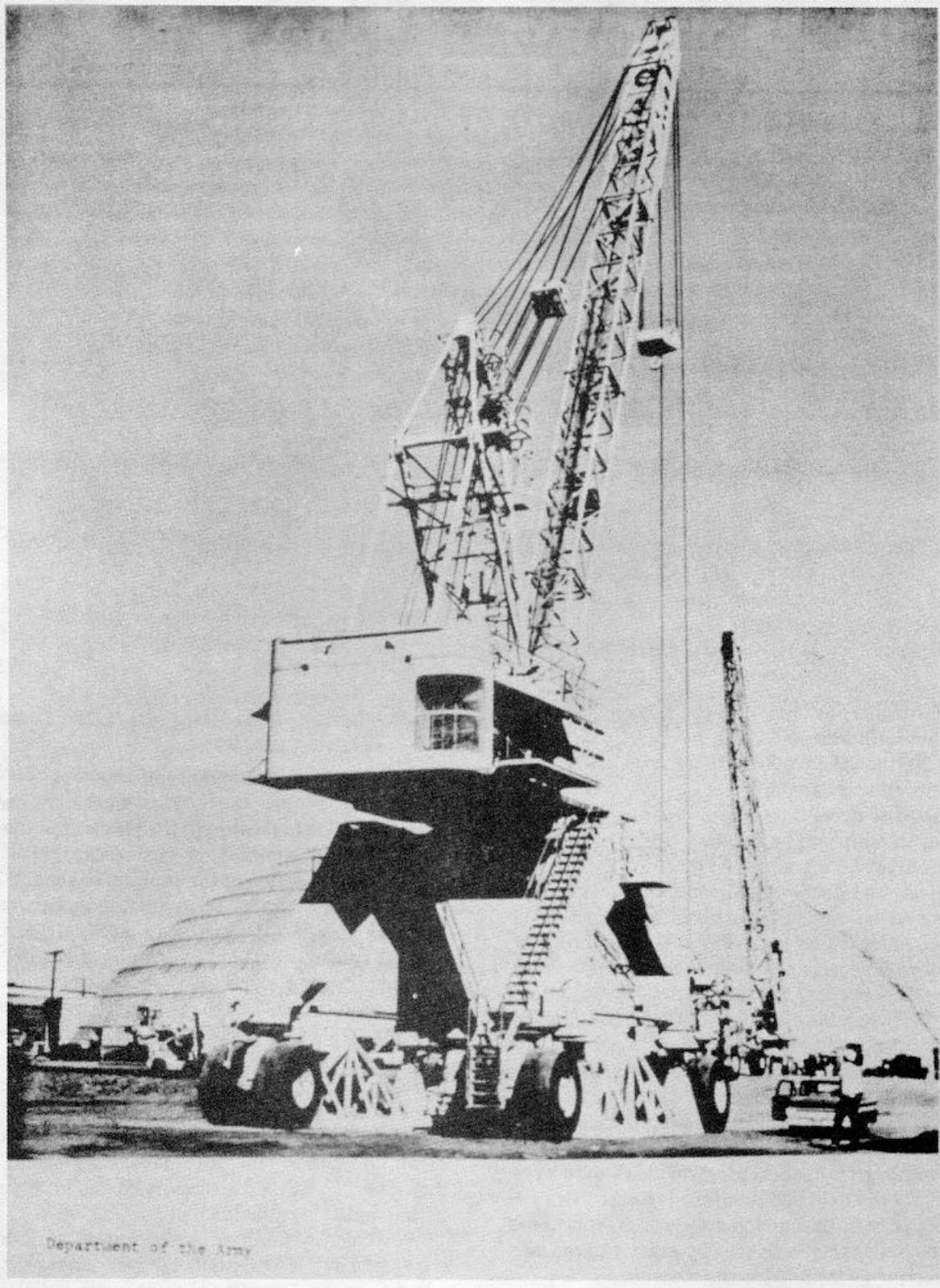
*Figure 12-2. Typical heavy duty, rubber-tired gantry crane.*
