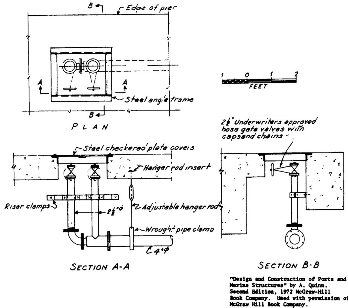
Figure 11-1. Typical water-supply connection in deck of pier
