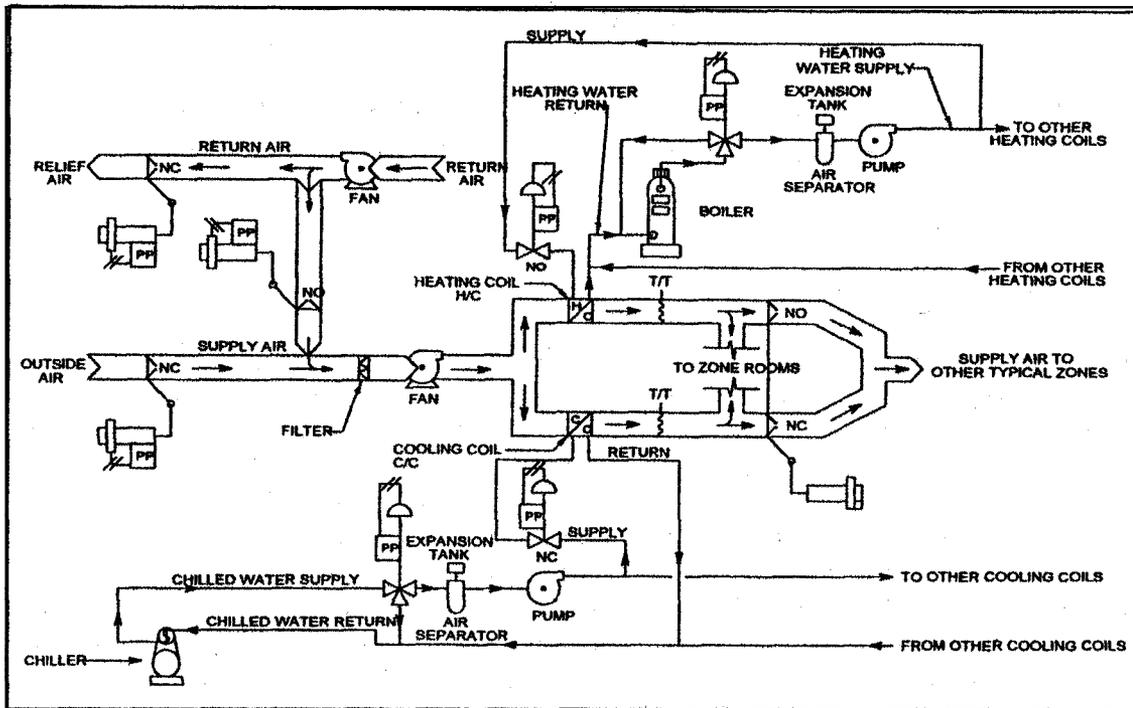
Figure 4-1. Schematic of a typical HVAC system
