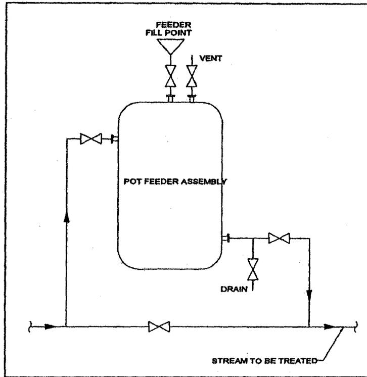
Figure 10-2. Schematic of a process water treatment system
