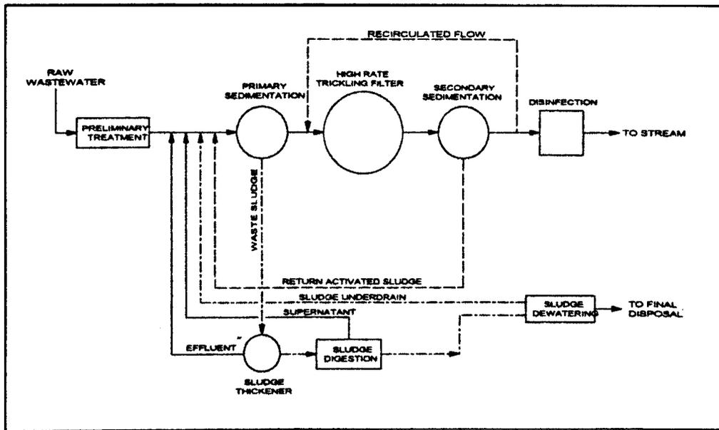
Figure 10-4. Sewage trickling filter process
