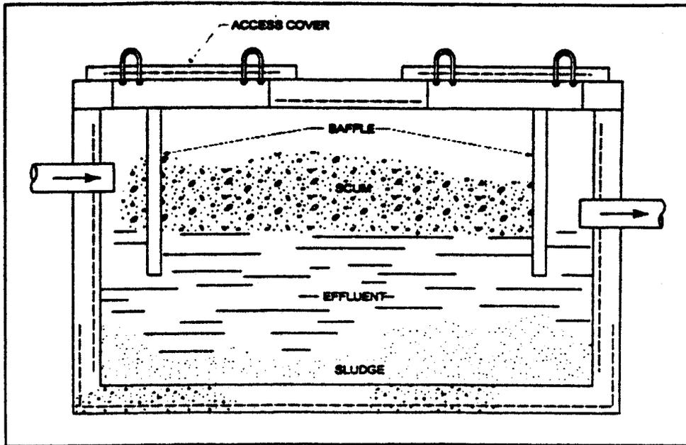
Figure 10-3. A cross section of a septic tank
