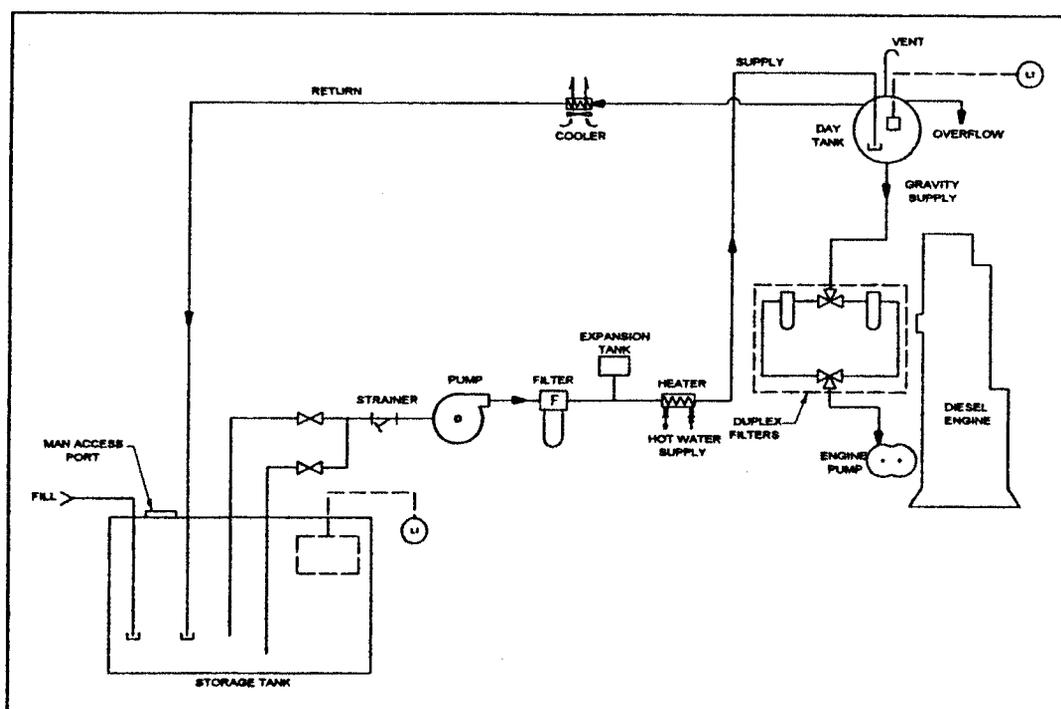
*Figure 5-1. Schematic of a typical diesel fuel system*
