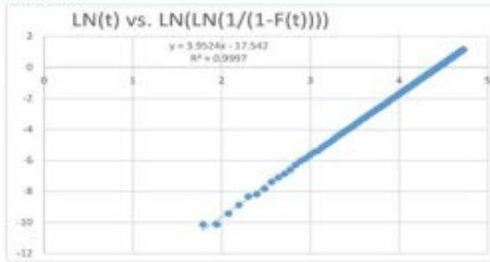
Parameter estimation via ordinary least square using Weibull plot with trendline using linear best-fit regression.
