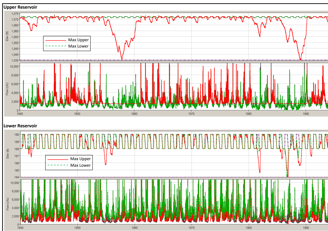
Figure A-60. Time-series plots of reservoir storage and inflow/outflow for two reservoirs in series, first maximizing yield at Upper Reservoir (red, yield equals 1,479 cfs at Upper Reservoir
