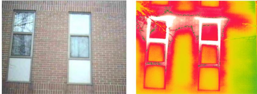
**Figure 0-4. Blower door tests complemented by thermography identify problems with building air tightness and areas with poor insulation where leakage occurs (shaded and white areas in the photo to the right)**
