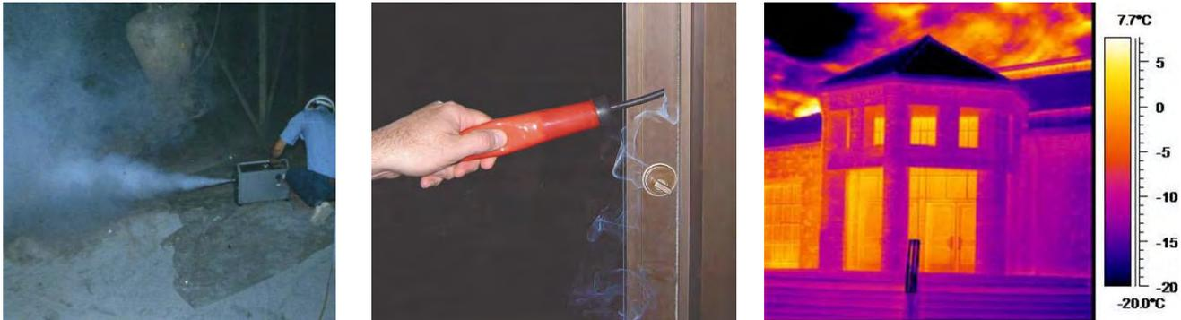
**Figure 0-9. Identification of leakage pathways using theatrical fog (left), smoke pencil (center), and infra-red thermography (right).**
