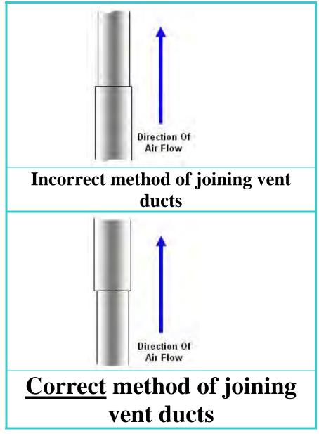
ECB: 2008-9 Subject: Proper installation of Type 1 Clothes Dryer vent system will extend dryer life, reduce energy costs and prevent fires.
