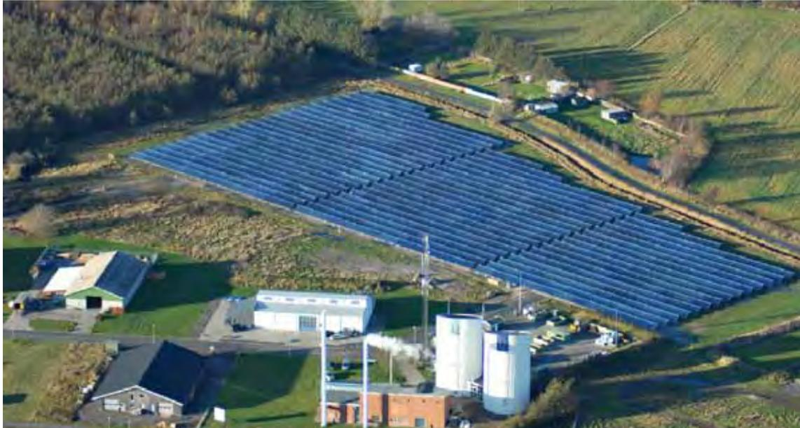
Figure A-22. Aerial image of the district heating plant of Strandby and the solar collector field.
